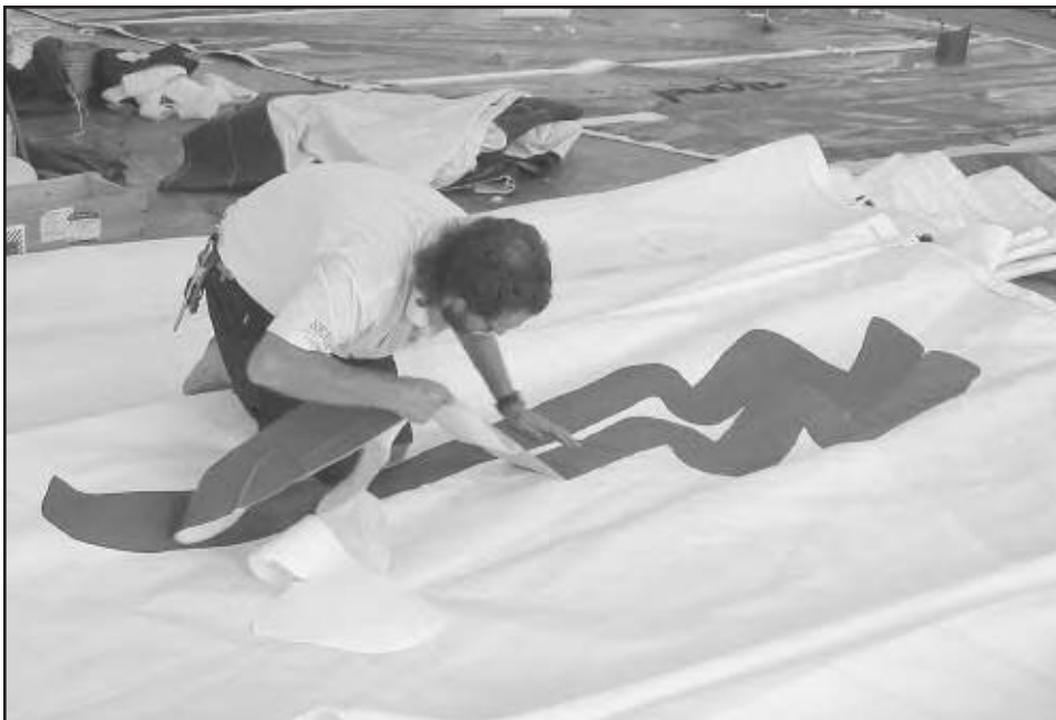
Most sailmakers will let you stroll around the loft floor so that you can watch sails being manufactured. Here a logo is being applied to a mainsail.
