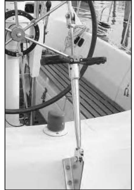
This mechanical vang works well for tensioning the backstay, but it's slow and cumbersome and best left to cruisers.
