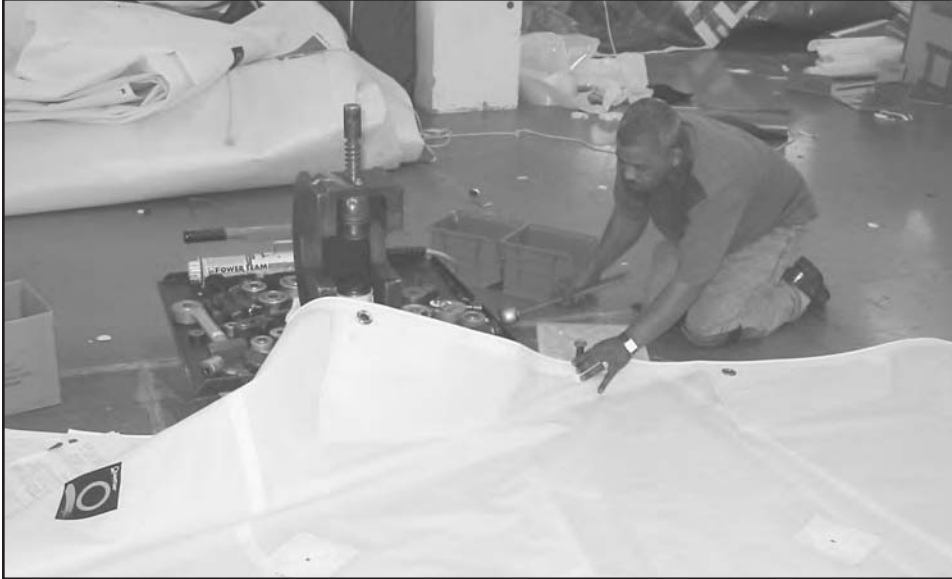
Workers use a hydraulic press to install heavy rings in the corners of sails.
