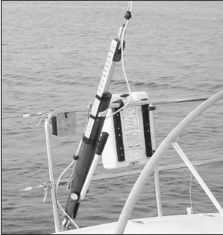
The hand-drawn gauge attached to this hydraulic backstay adjuster gives the sail trimmer quick and easy reference points.
