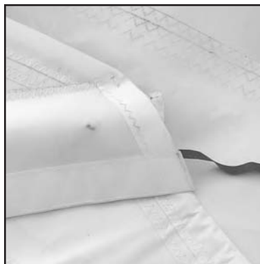
Detail work on the outboard end of a batten pocket showing tensioning device (left photo) and cover (right photo) that prevents the sail from hanging up on the backstay.
