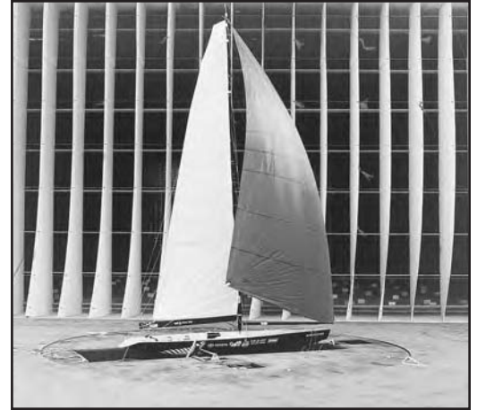
North Sails tests their America's Cup sails in a modern wind tunnel facility that can even simulate twist in the wind.
