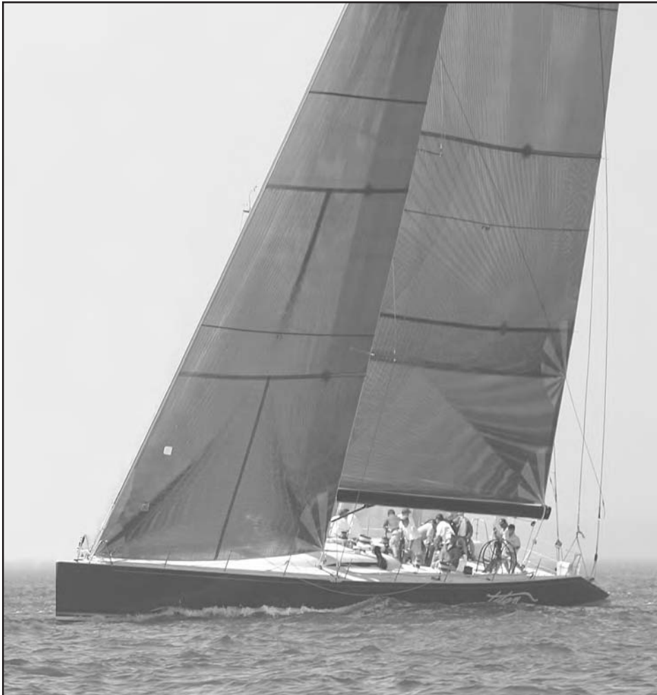
Doyle's D4 sails on board Titan. The D4 technology is starting to rival 3DL and Tape Drive.
