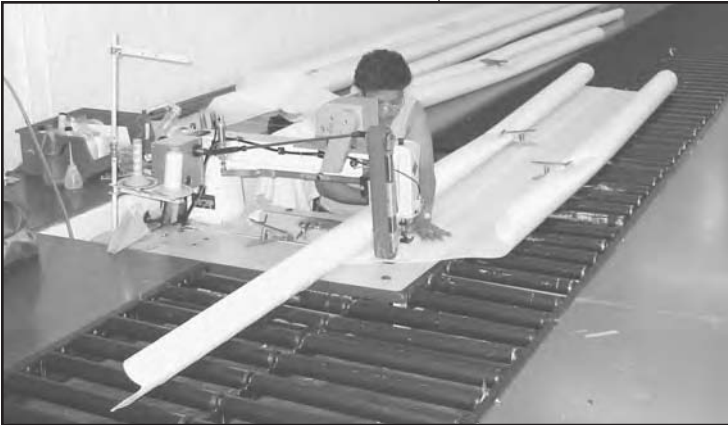
Sails are placed on rollers angled toward the sewing machine make it easier for the seamstress to handle large sails and sew a straight row of stitching.
