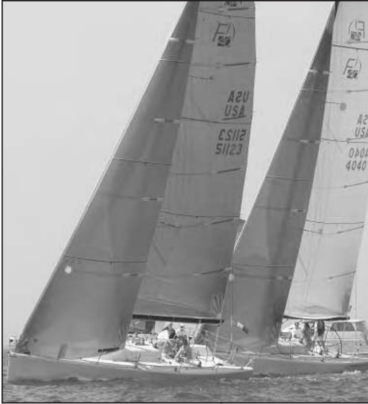
The telltales on the leech of this Farr 40 are all streaming perfectly meaning that the sail is trimmed properly.
