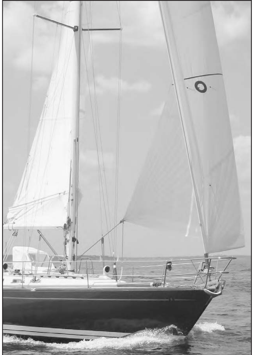
The foam pad along the luff of this headsail will allow for a better sail shape once the sail is reefed.
