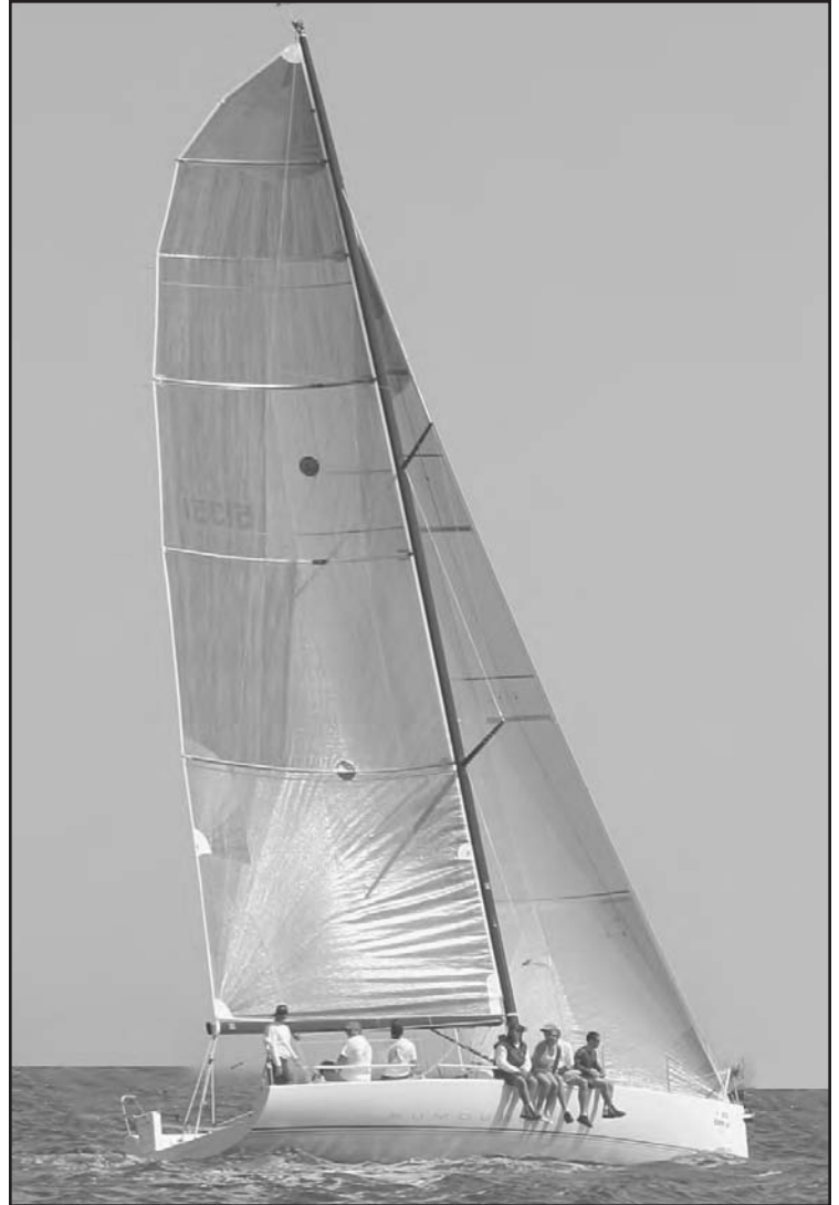
Full-length battens are necessary to support a large roach like the one seen on this sporty 30 footer.
