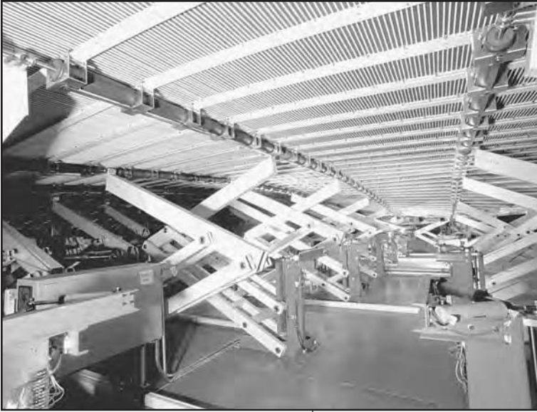
Looking under the 3DL mold platform where a series of computer-operated rams manipulate the shape of the mold to suit the design of the sail.
