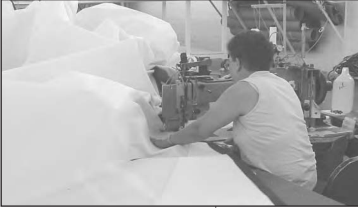
Sewing machines are sunk into pits so that it's easier for the seamstress to handle large, cumbersome sails.
