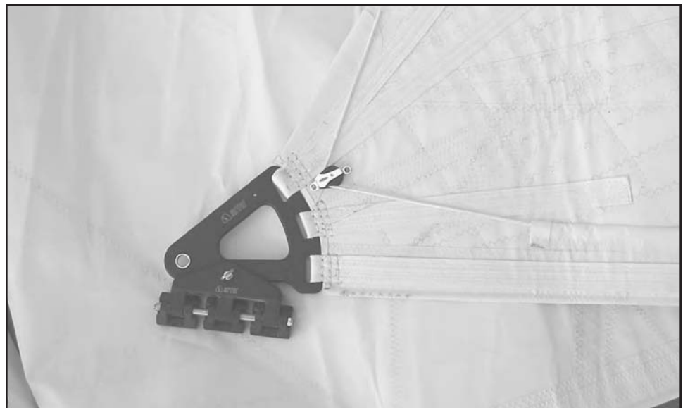
The head of a mainsail showing an overhead leechline running through a small block mounted just below the headboard.
