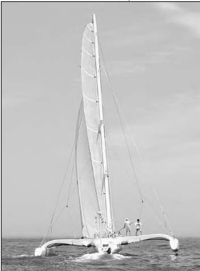
Looking up the back of the mainsail on this multihull reveals a flat shape perfect for a boat that sails at high speeds.
