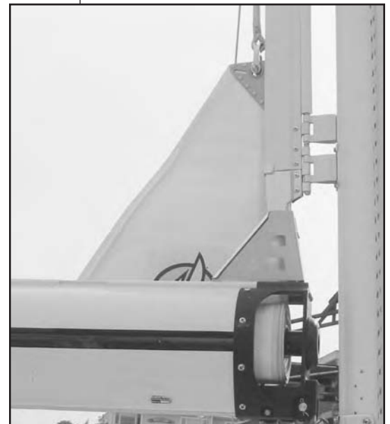
The gooseneck and luff feed system on an in-boom furling unit.
