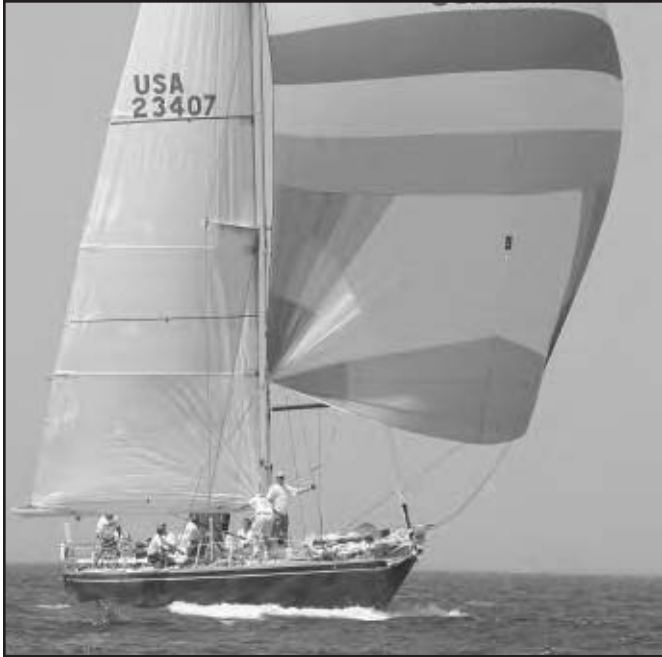
The tri-radial spinnaker revolutionized spinnaker design by allowing for more stable sail shapes.
