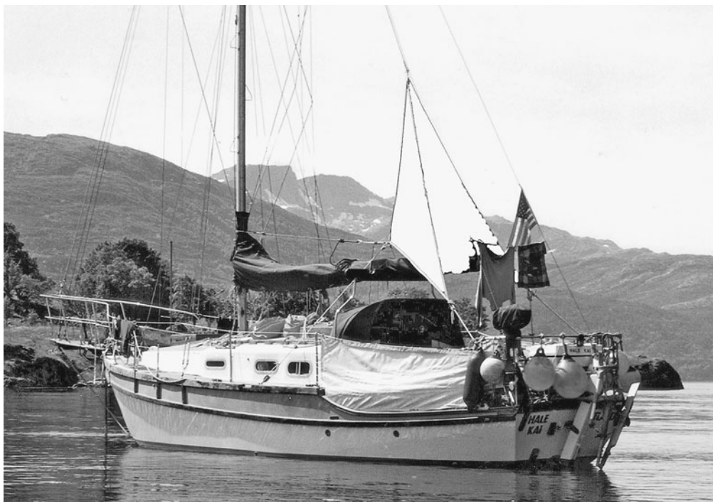
John Armitage's Hale Kai in Norway showing the V-shaped riding sail he devised after talking with local fishermen. Although John speaks of hoisting the riding sail on the ship's backstay, this photograph shows the head raised by the main halyard and the tack of the sail held in position by a line to the mast.
