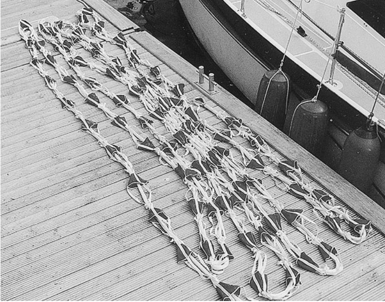
Cones and line spread out on a dock. For stowage, the drogue apparatus fits into one or two nylon duffel bags.
