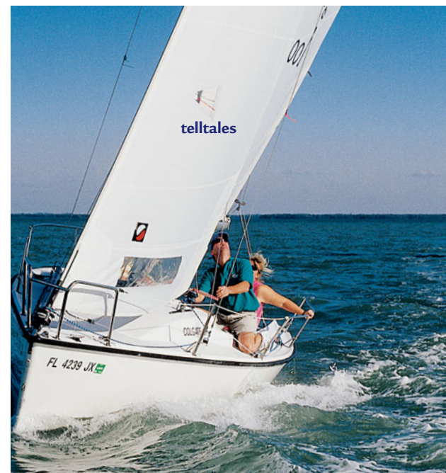
Figure 4-7. When both telltales stream aft, airflow is smooth and even.
