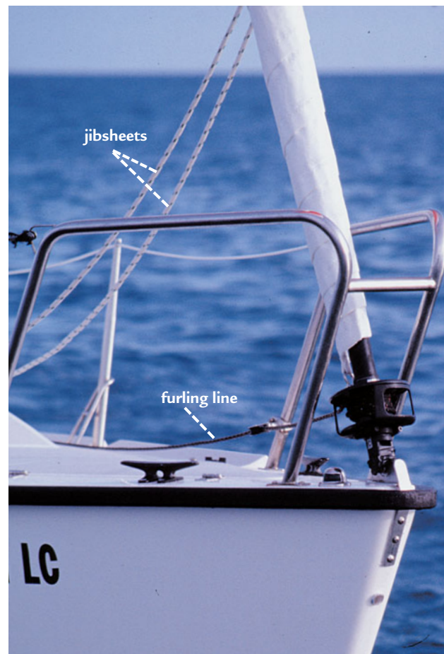
Figure 2-4. Jib furled around the headstay.
