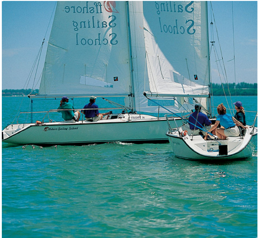
Figure 8-2. Same tack rule: boats are converging, leeward boat has right-of-way.
