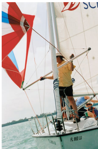
Figure 9-2. The start of an end-for-end jibe. Detach the pole from the mast first.
