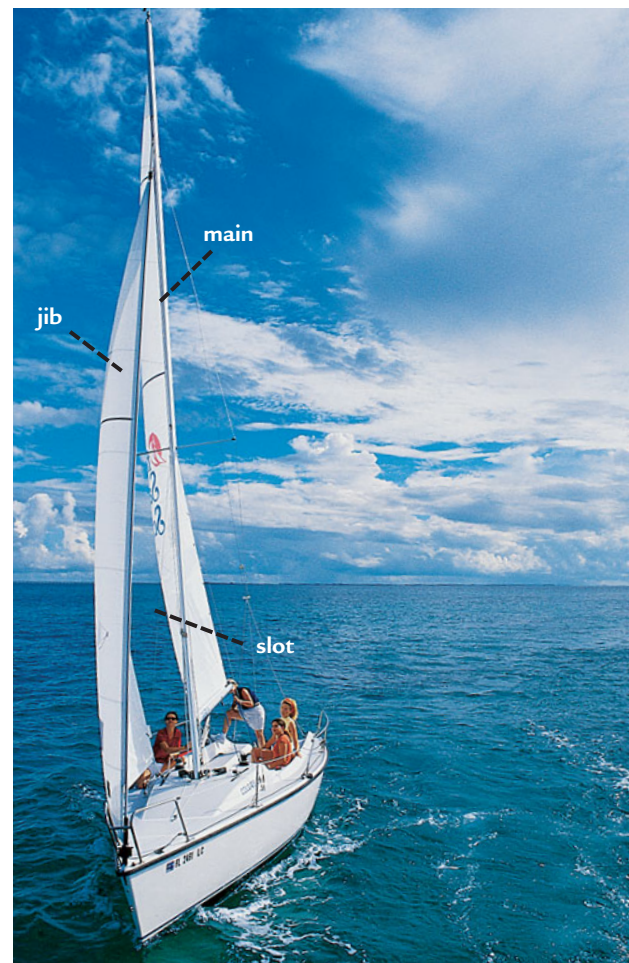
Figure 4-2. The slot between the jib and mainsail improves the wind flow and increases boat speed.
