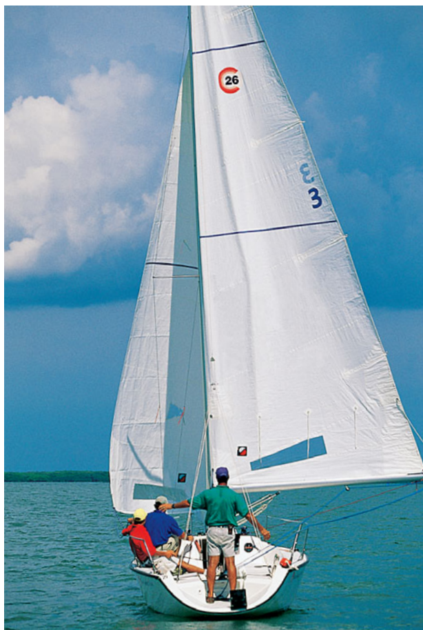
Figure 4-8. Sailing wing and wing with jib and main on opposite sides of the boat.
