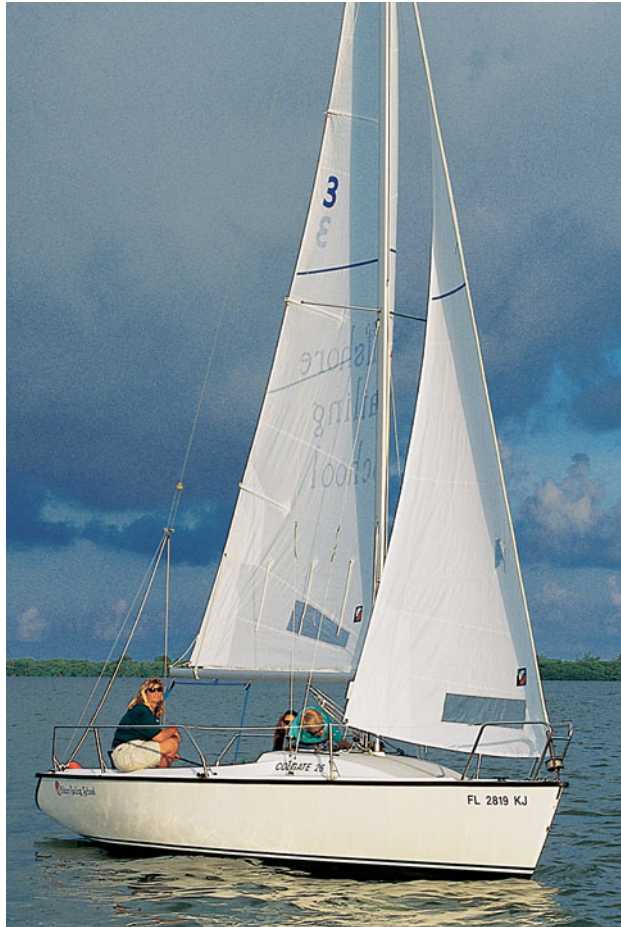
Figure 2-5. Backing the jib to get underway.
