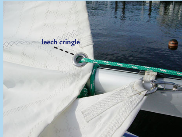
B. Tighten leech line to stretch foot of sail along boom
