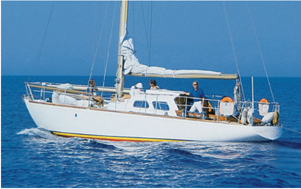
Figure 5-9. Left: Boat is traveling below hull speed (note small waves along hull).
