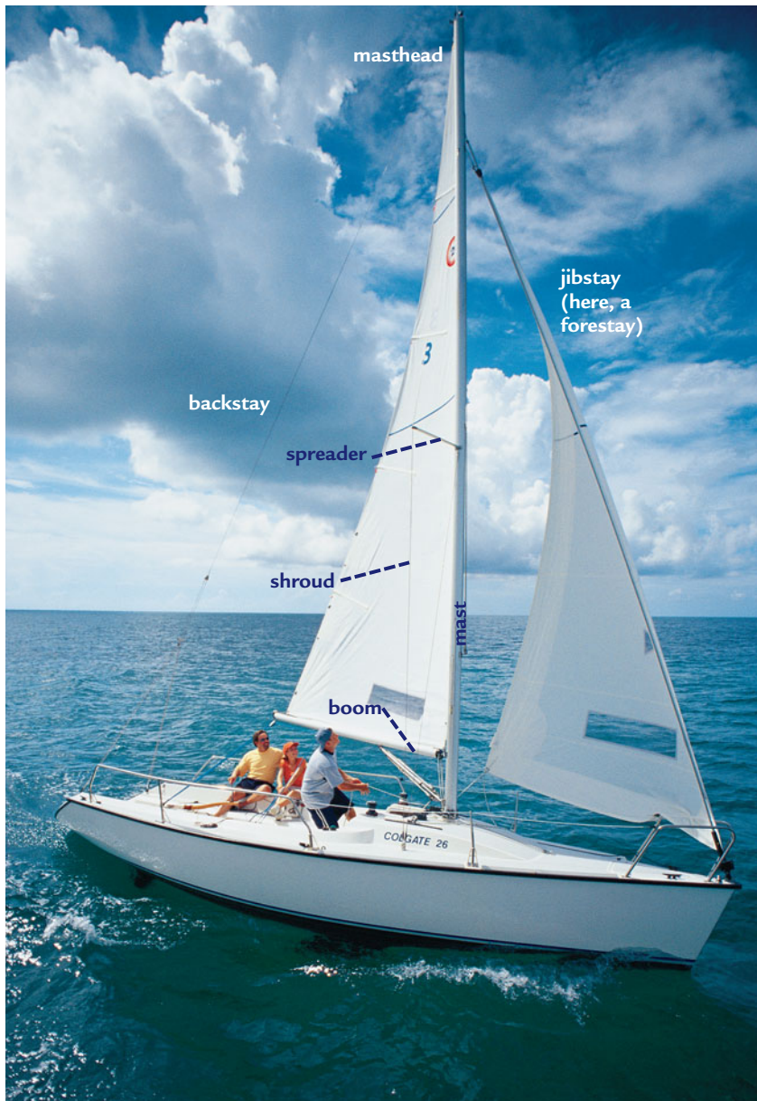
Figure 1-3. Terms that describe standing rigging.
