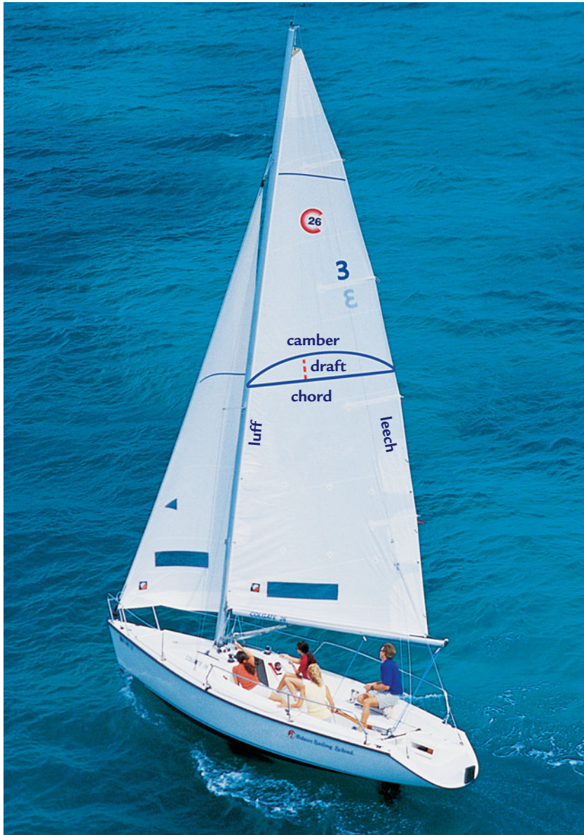
Figure 4-11. Chord, camber, and draft define sail shape.
