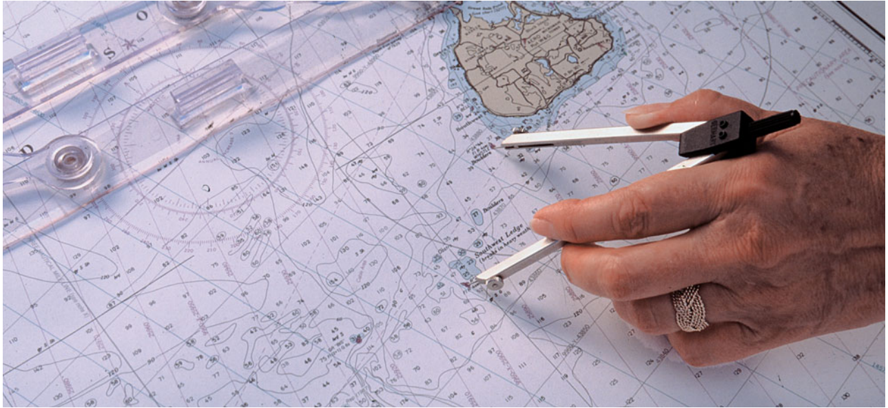
Figure 8-7. Finding distance using dividers.
