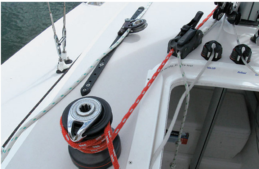
Figure 10-1. Here the halyard runs from the base of the mast, through a rope clutch, then to a self-tailing winch.
