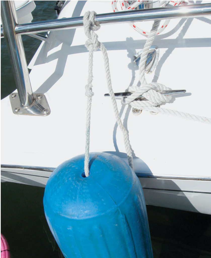
Figure 7-5. Tie fenders to the boat before docking.
