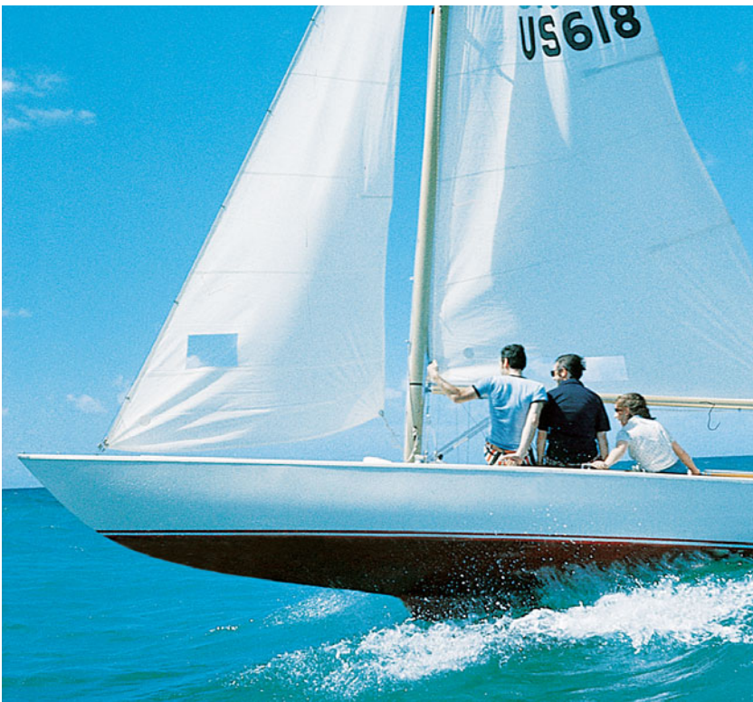
Figure 5-10. When sailboats surf, hull speed is exceeded.
