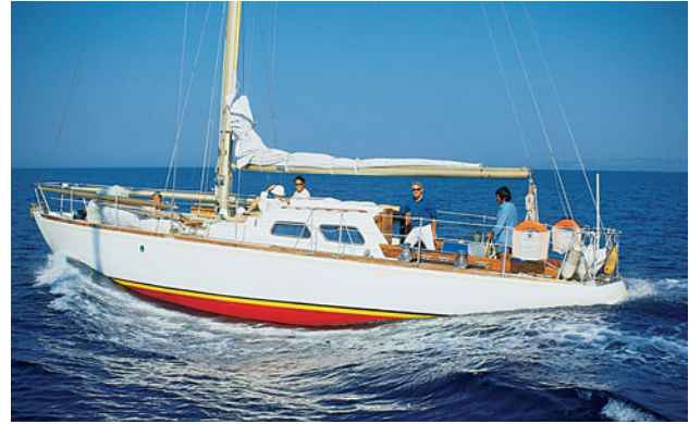
Right: Hull speed is shown in one long wave between the bow and stern.
