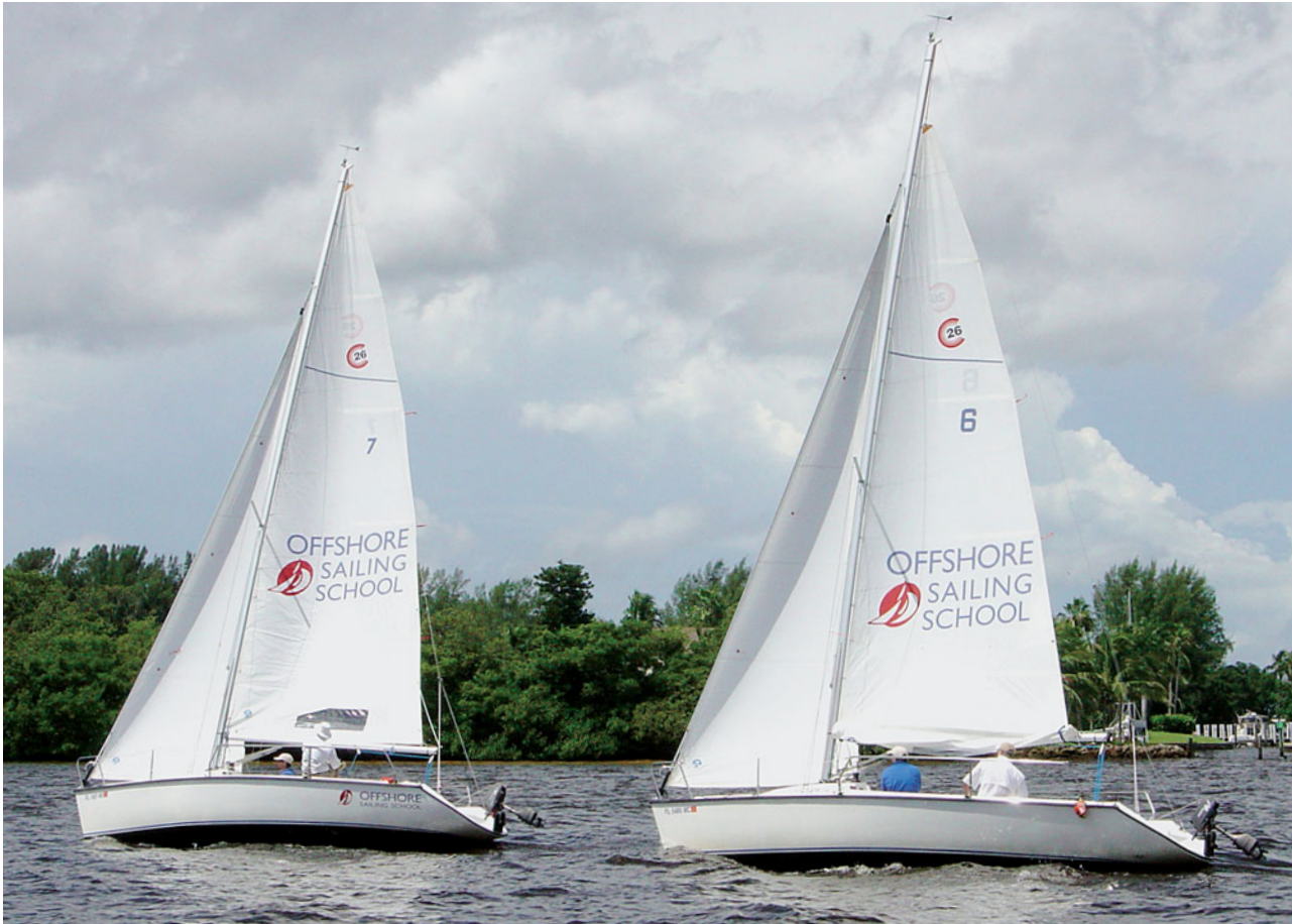
Figure 6-1. The difference between a reefed mainsail (right) and a full mainsail.
