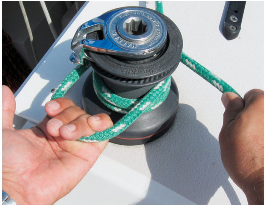
Figure 10-3. Improper way to add wraps to a winch.
