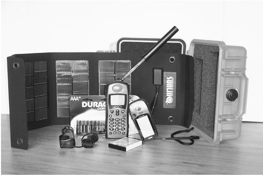
Figure 1-3. A modern electronic navigation backup kit. A satellite phone offers worldwide, all-weather connections as good as typical telephone calls. Dial 911 for assistance just as at home. Also shown is a handheld GPS unit and some extra batteries for it, but a satellite phone call can be triangulated for position even if the GPS fails. A spare battery for the satellite phone, solar charger, and rugged carrying case are also shown. On some systems you can place an emergency call as long as a SIM (subscriber identity module) card is in the device, even though a service plan is not active. Or you can move a SIM card from one unit to another. Check with your provider. (Courtesy globalmarinenet.net )
