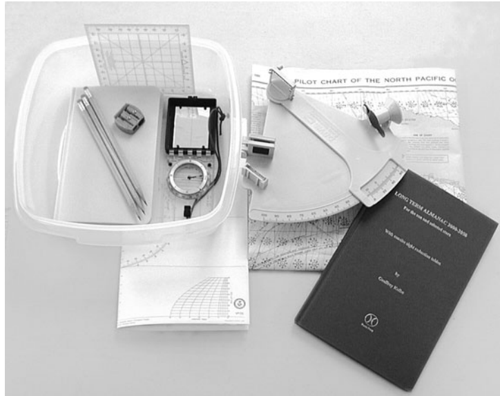
Figure 1-2. Backup navigational gear. Store this equipment in a waterproof bag, inside or near your regular emergency throw bag. Backup navigational procedures are discussed in Chapter 14. The Long Term Almanac by Geoffrey Kolbe shown here includes data for sun and stars until 2050 as well as a complete set of sight reduction tables, so this kit can take you safely to any port in the world, though it will be easiest if you are wearing a watch with known rate as suggested throughout the text. Also shown are a waterproof notebook, Pilot Chart, plotting sheets, pencils, sharpener, and compass.
