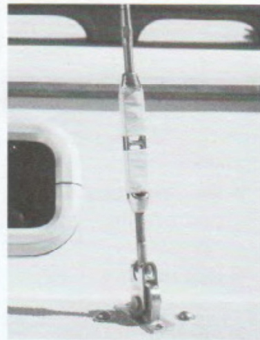
The shroud length can be adjusted at deck level by a mechanical device called a turnbuckle ③, which can be tightened or loosened. The turnbuckles are secured with pins, and the tape covering them protects you and the sails from rips or tears.
