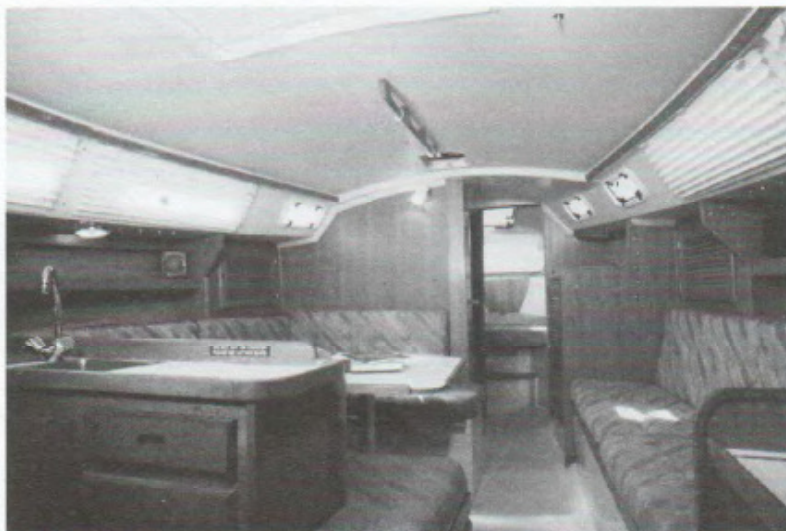
The saloon ① is viewed looking toward the forward cabin with the galley sinks and dining area on the left ( port ) side. Attached to the overhead is a grab rail to use when sailing upwind or in rough conditions.
