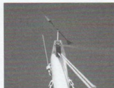
The masthead fly points to the direction from which the wind is blowing. With practice, you'll sense how close you can steer to the wind and stay in the groove.
