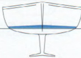
A winged-keel allows a shallow keel to perform more efficiently.
