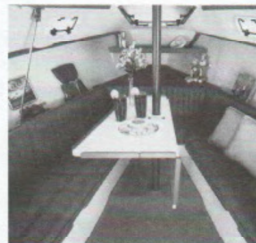
This is a view facing forward on a small cruising boat. The table can be lowered to convert into a vee-berth ④.
