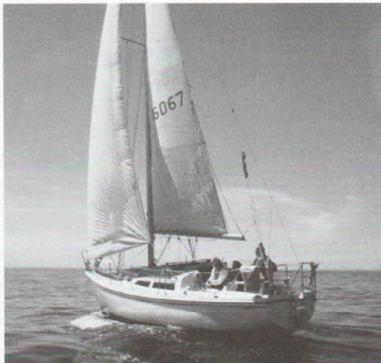
The sails are trimmed all the way in so that the wind flows smoothly off both the main and jib.
