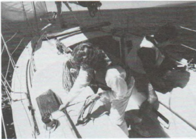
The boat is ready to tack. One of the jib trimmers prepares to release the sheet holding the jib while the other prepares to pull in the opposite sheet after the jib passes in front of the mast.
