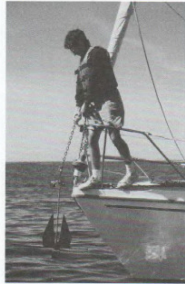
The crew is ready to lower the anchor, with the rode coiled and the anchor line led under the pulpit.
