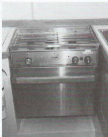
The stove is usually gimballed to stay level regardless of heel.
