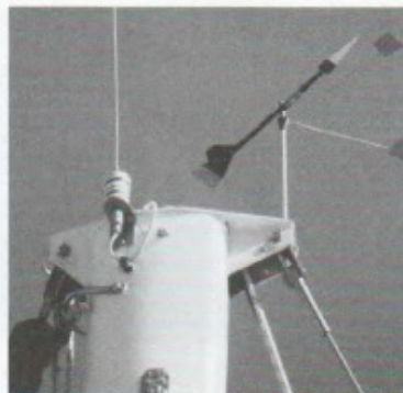
At the masthead ②, the halyards run over a pulley ( sheave ) at the top of the mast and then down to the deck.
