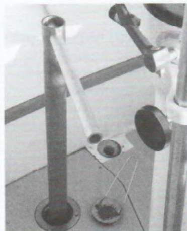
Remove the access plate above the top of the rudder post to install the emergency tiller. There are different types of emergency tillers. In this photo, the wheel has been removed to allow unobstructed movement of the tiller.
