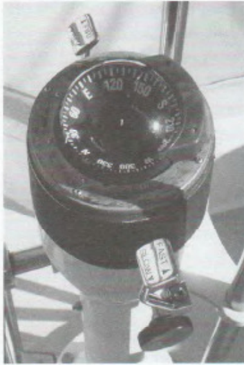
Engine controls are located close to the steering station so the helmsman can operate the throttle and gear shift.
