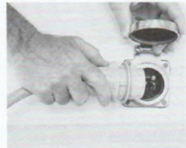
Shore power outlets on cruising boats provide electricity for charging the battery.
