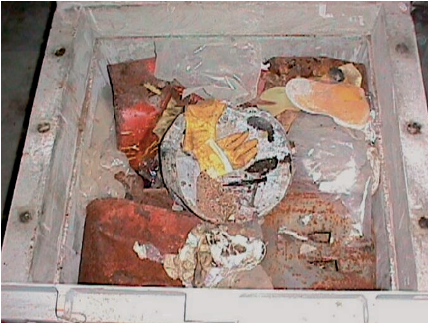
FIG. 9. Example of retrieved LLW in a transfer/storage container.
