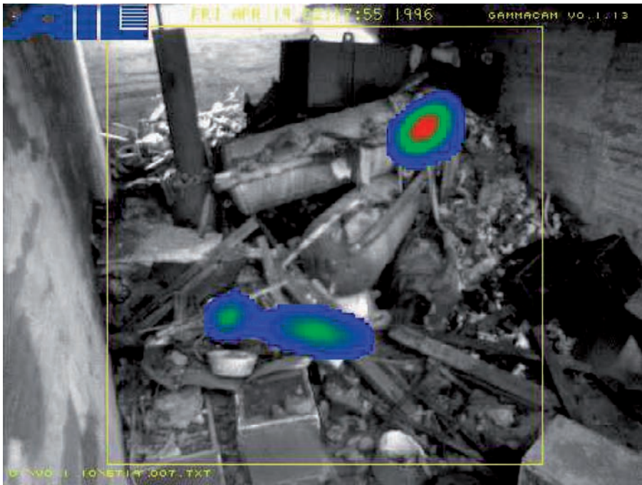
FIG. 10. Gamma image of an old waste storage cell identifying hot spots.
