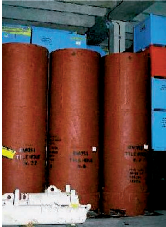
FIG. I-3. Storage of encapsulated tile holes in a low level storage building.
