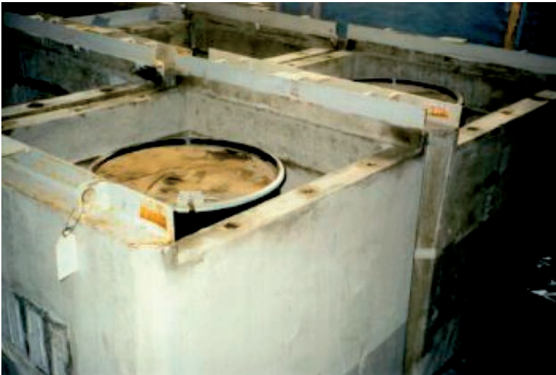
FIG. 25. Example of a concrete overcontainer for a drum.
