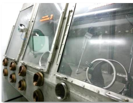
Figure 7.8. Facility for radioactive waste sorting before incineration
