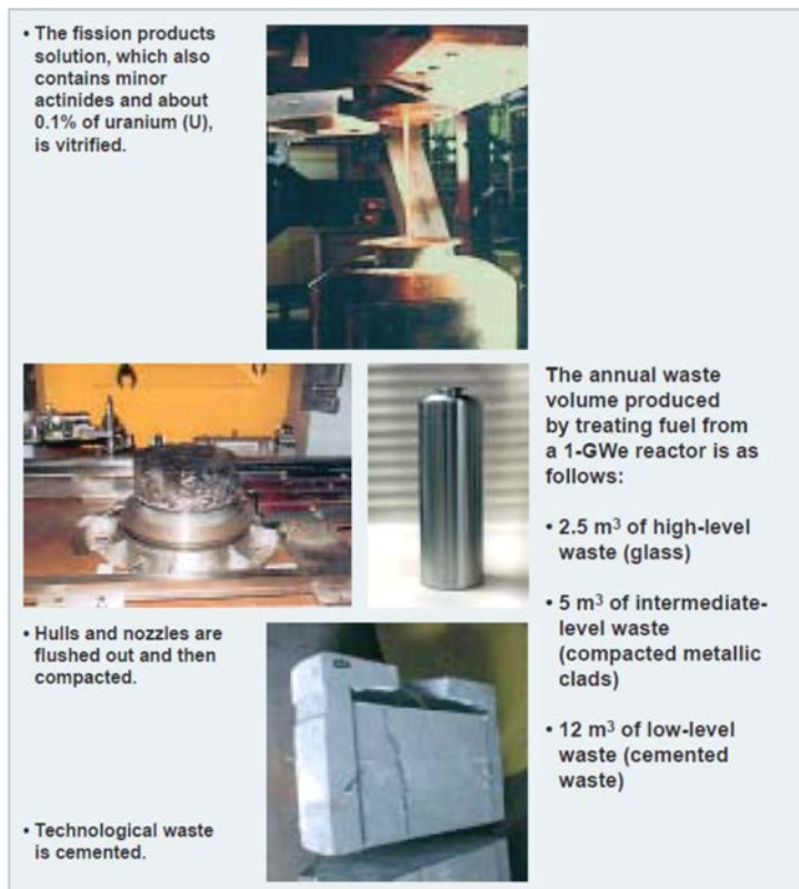
Figure 7.5. Ultimate waste arising from spent fuel treatment
