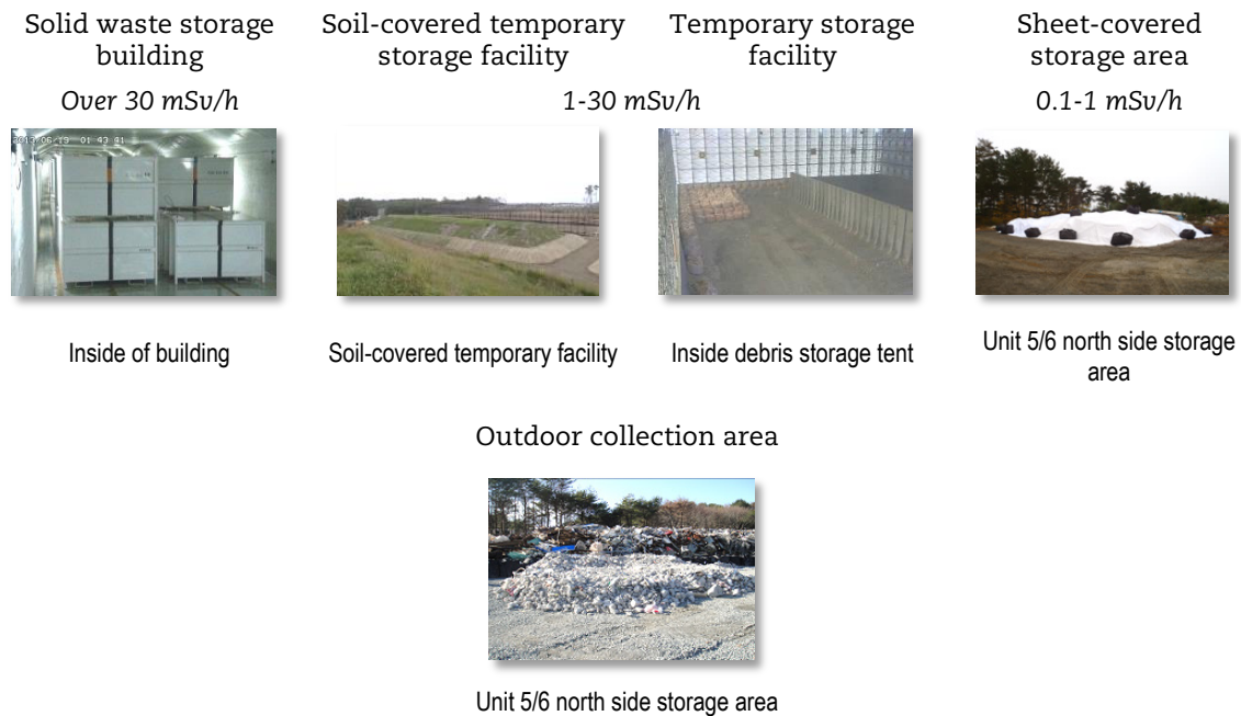
Figure 4.9. Debris collection at Fukushima: Waste categories and temporary storage areas
