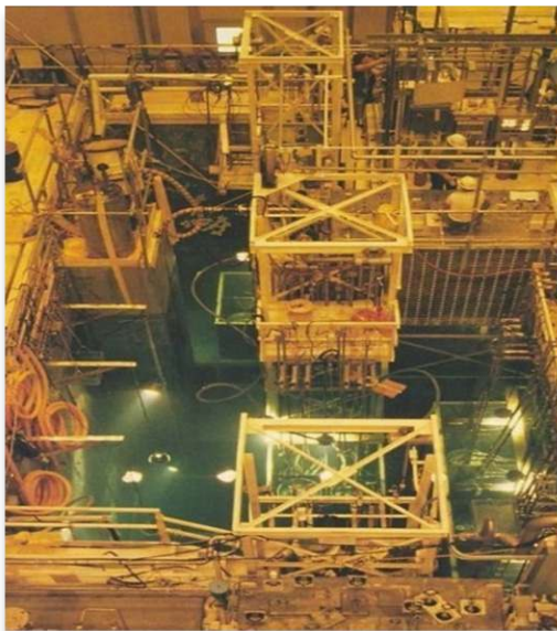
Figure 2.3. Processing and decontamination of high-level radioactive waste water by the SDS
