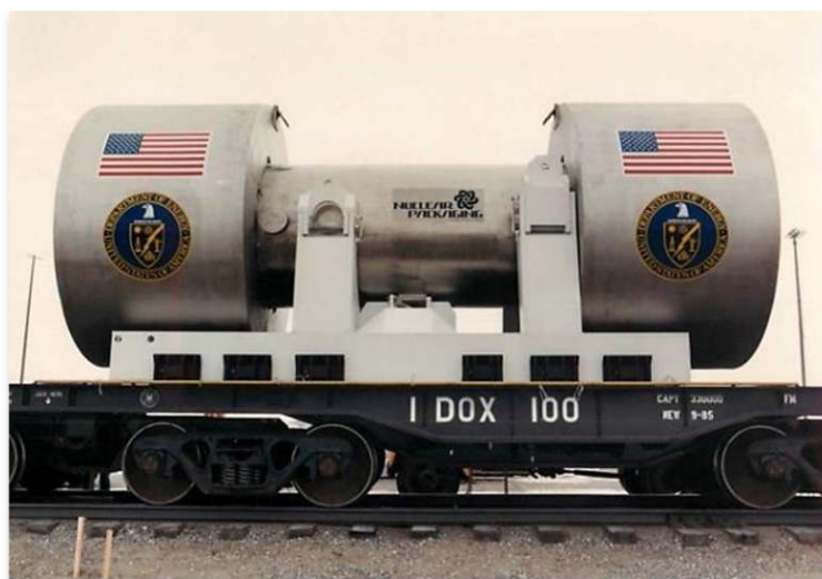
Figure 2.16. Model 125-B rail shipping cask used for transporting defuelling canisters
