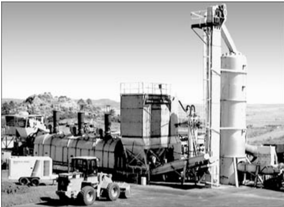
FIGURE 4.6.2.7 Indirectly heated thermal desorber: recovery ECS.
