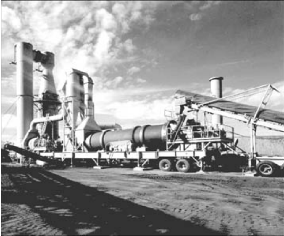
FIGURE 4.6.2.6 Directly heated thermal desorber: destructive ECS.
