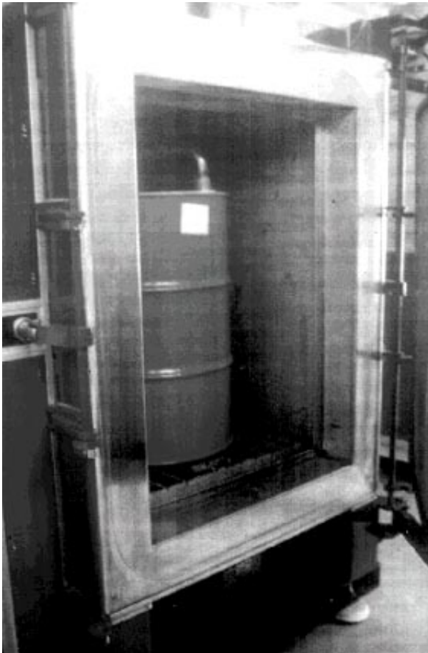
FIGURE 4.3.2 Drum feeder with door open and drum inside.
