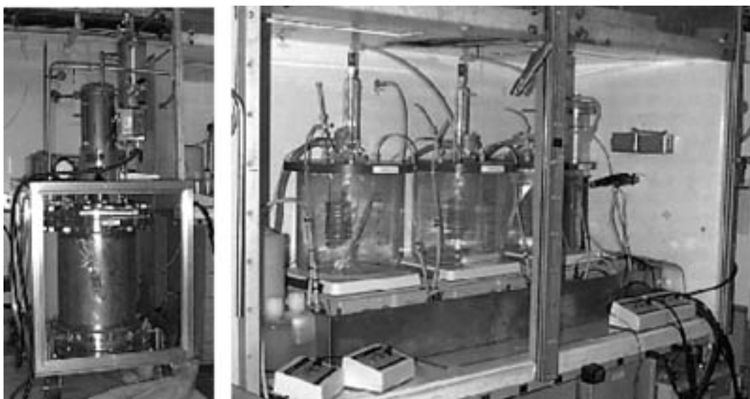
Figure 5.2.4.4 Pilot-scale laboratory unit used in destruction of trichloroethane (TCA) solvents, 15 kg/day. The 60-L hydrolysis vessel (left) converts TCA into water-soluble species, which are oxidized in a three-stage CSTR system (right). Data from this system is presented in Table 5.2.4.6 .
