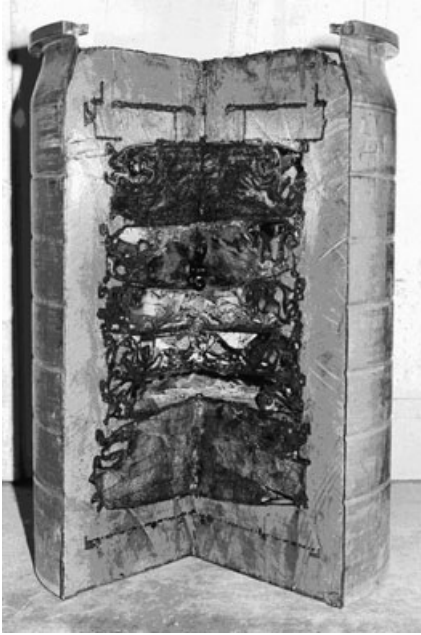
12.10 Sectioned waste package consisting of a series of 'pucks' (supercompacted 200 litre drums) cemented into a larger stainless steel drum (courtesy Sellafield Ltd, UK).
