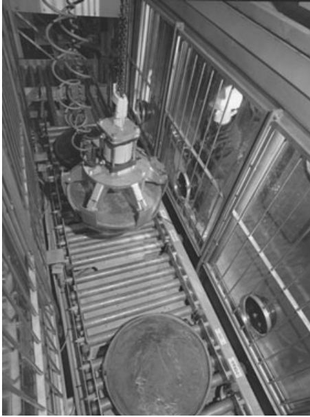
2.9 High-force compacted pellets in an ISO disposal container (photo courtesy of UKAEA Dounreay).
