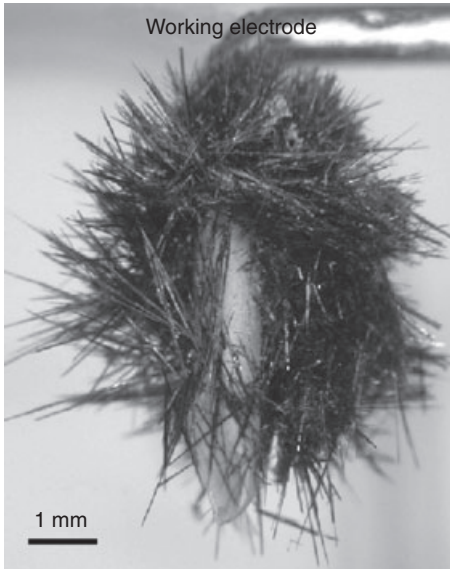
10.13 Optical microscope image of hollandite crystals grown at the tip of the working electrode observed by Abe et al. [99].
