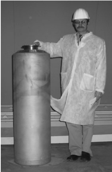
12.6 Stainless steel container (primary waste package) for vitrified high-level waste in France and UK (courtesy Sellafield Ltd, UK).
