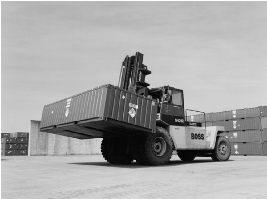
12.14 A waste container being handled by forklift in Vault 8 at the UK near-surface repository for LLW in north-west England (courtesy LLW Repository Ltd, UK).
