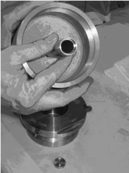
12.11 BOSS capsule and container with concrete insert. The lids of the container and capsule can be seen at the bottom of the picture.
