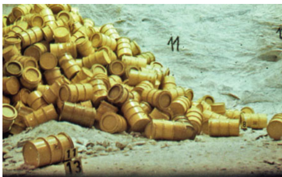
Fig. 6.21 MAW-barrel cone, storage on the 511 m level (emplacement chamber 8). Source Michel [34]
