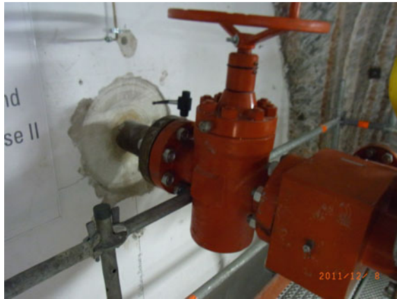
Fig. 6.23 Fact-finding, drilling site with preventer. Source M. Lersow
