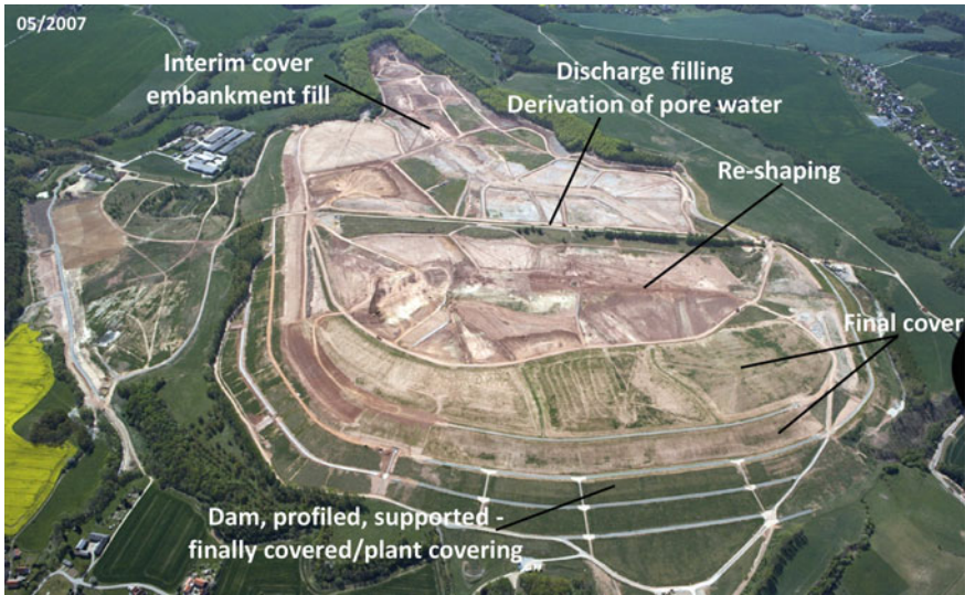
Fig. 5.13 Uranium mill tailings Pond “Trünzig”, cover details during the remediation progress. Source [29]
