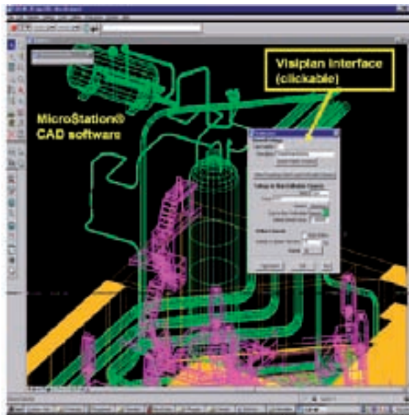
FIG. 6. Typical Visimodeller screen shot. Geometrical elements from complex environments are selected by a simple click of the mouse.
