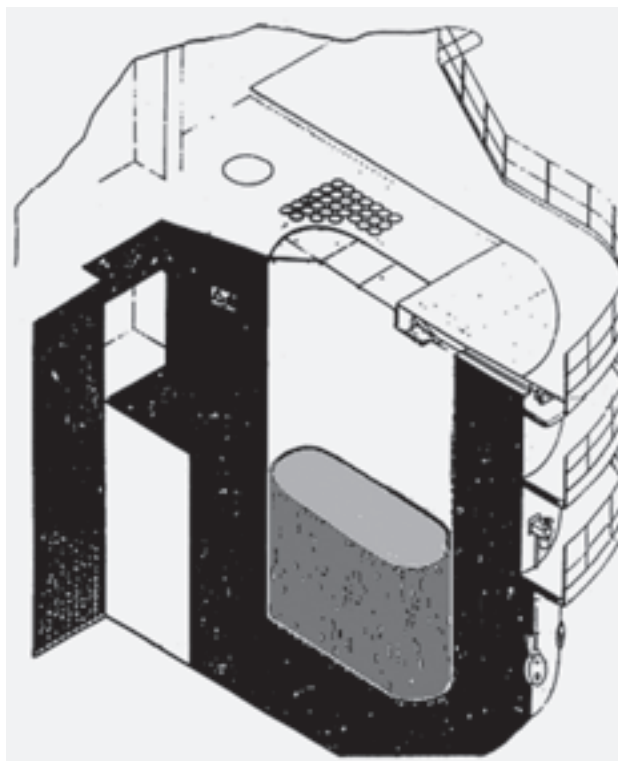
FIG. 14. Sketch of the tank of the IRT-M nuclear reactor after concreting.
