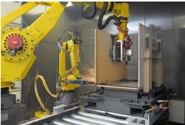
Fig. 8.26 Automated Fuel skip sectioning using robotic laser cutting.
