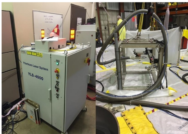
Fig. 8.27 Underwater laser cutting set-up.
