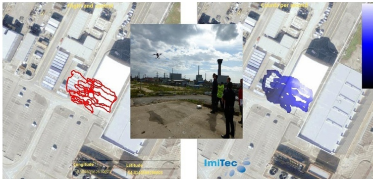
Fig. 8.12 ImiTec Autonomous Drone Outdoor Radiation Mapping at Sellafield [125].
