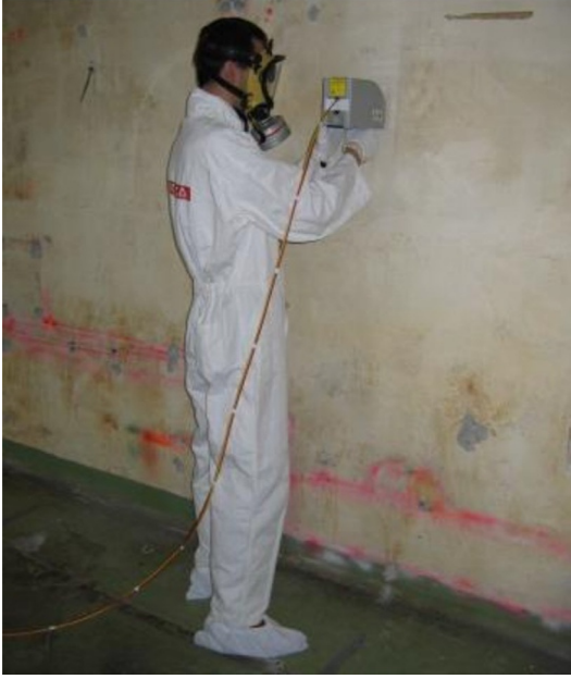
Fig. 8.18 CEA LIBS prototype testing at uranium manufacturing facility [125].
