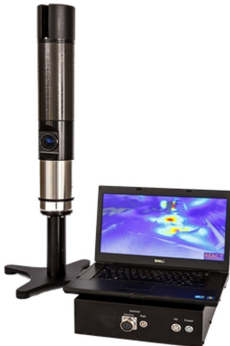
Fig. 8.9 NVisage reduced size 3D gamma camera [124].
