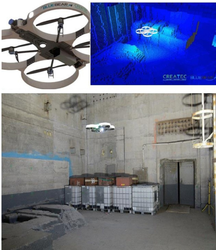
Fig. 8.11 RISER NVisage 3D gamma camera on blue bear autonomous drone [126,125].
