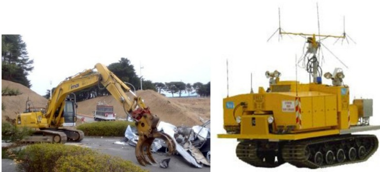
Fig. 8.32 Remotely operated excavator used at Fukushima Daiichi from [157] and French INTRA EREL T (Tele-operated Relay Robot) Mobile Wi-Fi Platform. [164]
