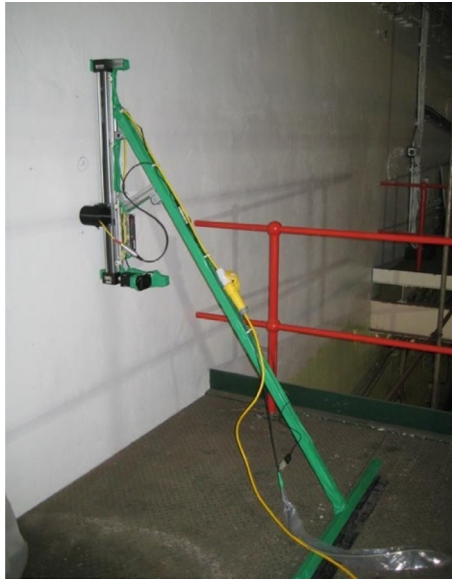
Fig. 8.15 Example of concrete profiling equipment setup undergoing testing at Sellafield [125].
