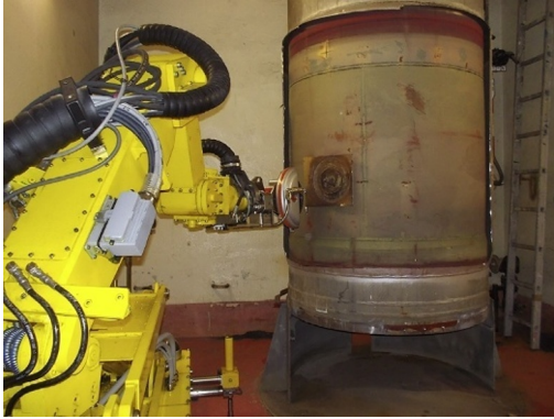
Fig. 9.15 Remotely controlled teleoperator MT 80 fragmentation evaporator of D_2O .
