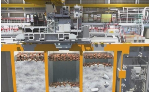
Cut away view of Sellafield Magnox Swarf Silo.
