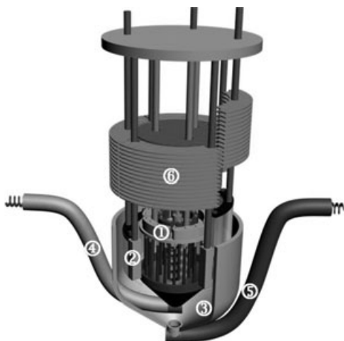
10.33 Conceptual design of continuous high-throughput electrorefiner of KAERI. 1) cathode module, 2) anode basket, 3) reactor wall, 4) deposit withdrawer, 5) noble metal withdrawer, 6) heat shield.
