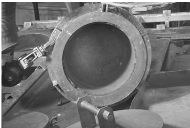
10.26 Zirconia-lined graphite crucible after cathode processing.
