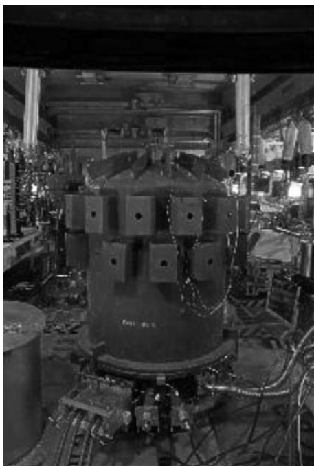
10.23 Furnace for producing metal waste form installed in hot cell of INL.
