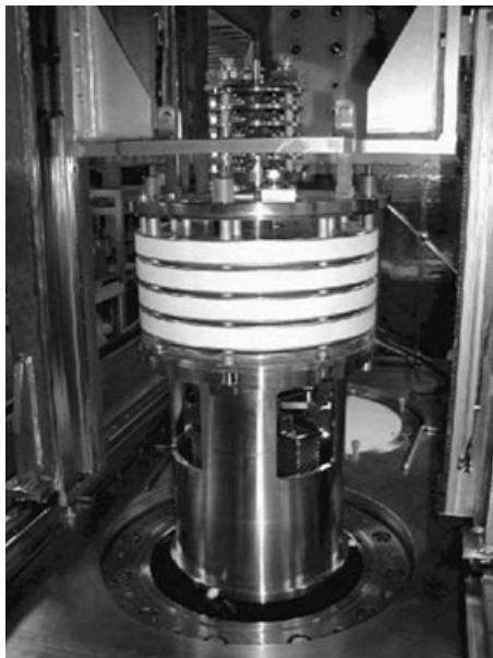
10.13 High-throughput anode-cathode module of CRIEPI.
