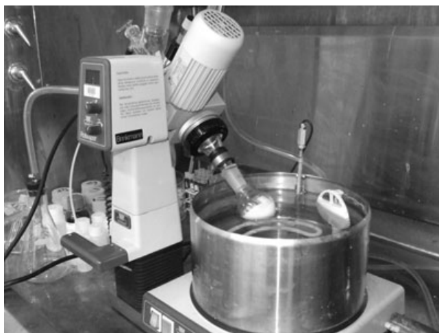
13.2 Resin preparation via dry impregnation – diluent evaporation step.
