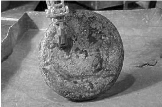
10.17 Plutonium-uranium-MA ingot obtained in cathode processing.
