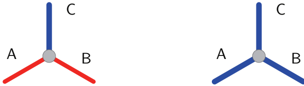
(a) AND vertex. Edge C may be directed outward if and only if edges A and B are both directed inward.
