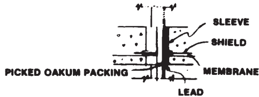
TYPICAL SLEEVE THROUGH FLOOR SLAB WITH MEMBRANE
