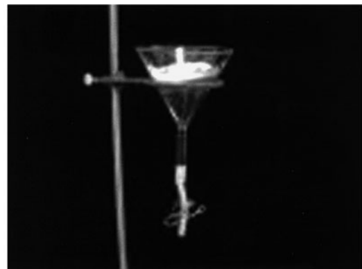
Figure 28.2 (Upper) Baermann apparatus. (Illustration by Nobuko Kitamura.) (Lower) Baermann apparatus set up in the laboratory.
