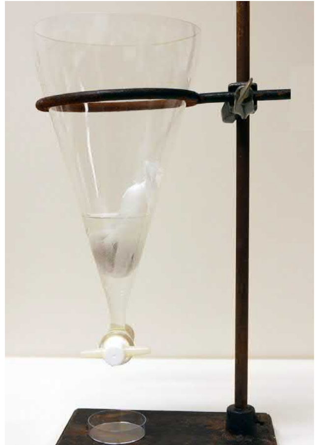
FIG. 11.3 The principle of the Baermann method: the fecal sample is placed into a water-filled funnel in a gauze pouch. Nematode larvae migrate through the gauze into the water and sink to the bottom of the funnel, from where they can be collected for microscopy.
