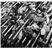
Figure 2.27. Bar screen for separation of overthick chip (Rader®).
