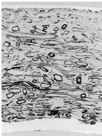
Figure 4.7. Cross section of a box board with CTMP in the middle and chemical pulps in the outer layers.
