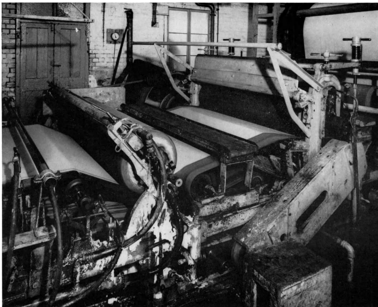
No. 136. Couch and press part of a machine at the Melbourne Mills of Australian Paper Manufacturers Limited, made by Redfern, Smith and Law, of Bury, Lancs., in 1871, and still running. Apart from a few small modern additions this machine is much the same as when supplied nearly ninety years ago.
