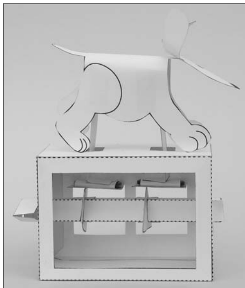
Figure 10-22: The pushrods attach to the cam followers.
