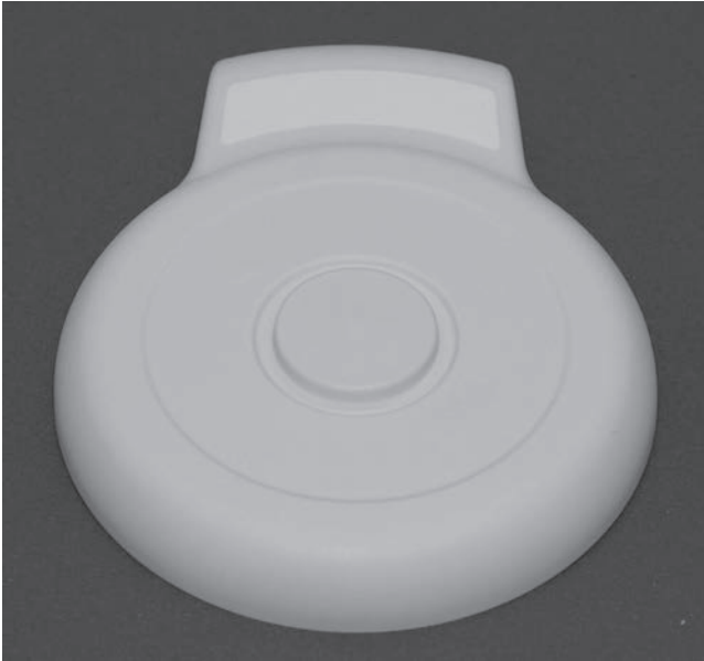
Figure 4.34. This figure shows the new Toco transducer developed by Philips: It has an integrated maternal optical reflection sensor system giving a continuous maternal pulse rate signal that is automatically used to detect fetal/maternal signal coincidence.
