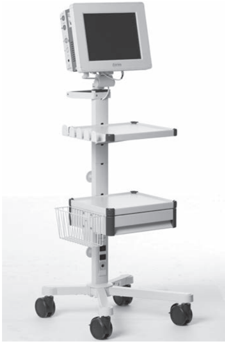
Figure 9.7. This is the device marketed by Neoventa of Sweden that contains an FHR monitor and a computer that analyzes the fetal ECG and alerts the clinician to various changes of the ECG waveform that suggest fetal hypoxia.
