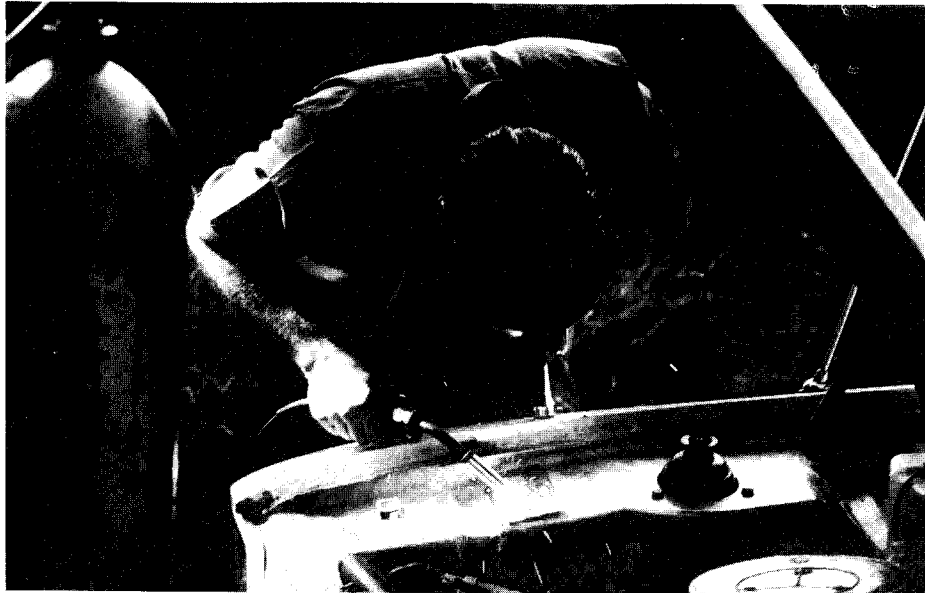
Welding a patch under a car bonnet is a common repair and is effectively a fillet joint round all four sides of the patch. Note earth clip, centre foreground.
