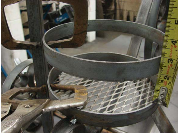
Figure 13-45. Lower, top ring clamped in place.
