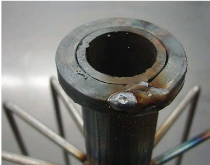
c) Void in rim filled with a series of small tacks.
