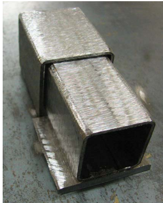
Figure 8-6. Attaching the Top and Center Tubes.
