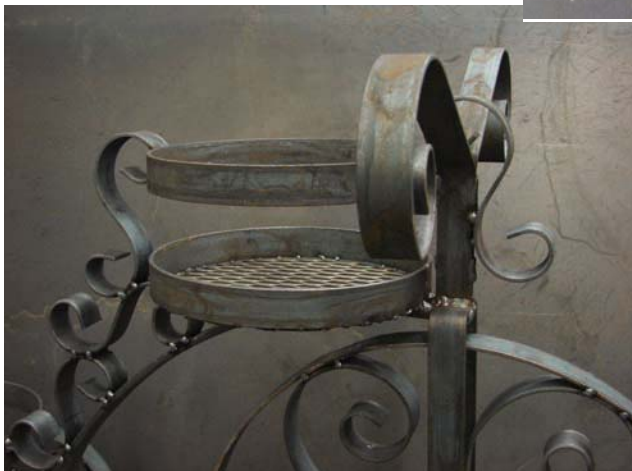
Figure 13-48. Upper rings and wrought iron pot connectors attached and welded solid.
