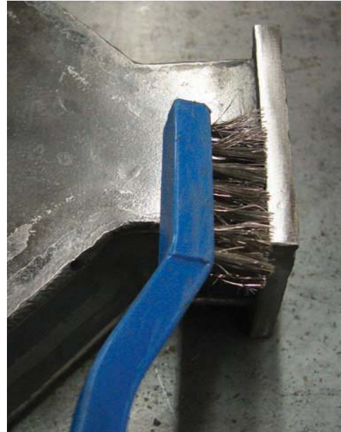
Figure 7-39. Using a wire brush to clean the hard to reach areas of the vase.
