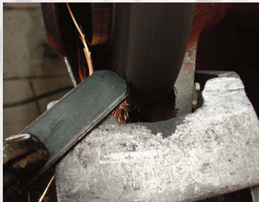
Figure 2-15. Shape the rounded end of the tongue.
