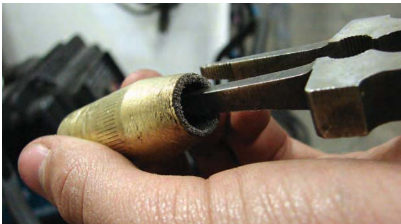
Figure 1-25. a) Clean the nozzle regularly to allow maximum gas flow from the nozzle. b) MIG pliers are specially designed to help you tighten or remove consumable parts in the wire feed gun, clean the nozzle, and clip wire.
