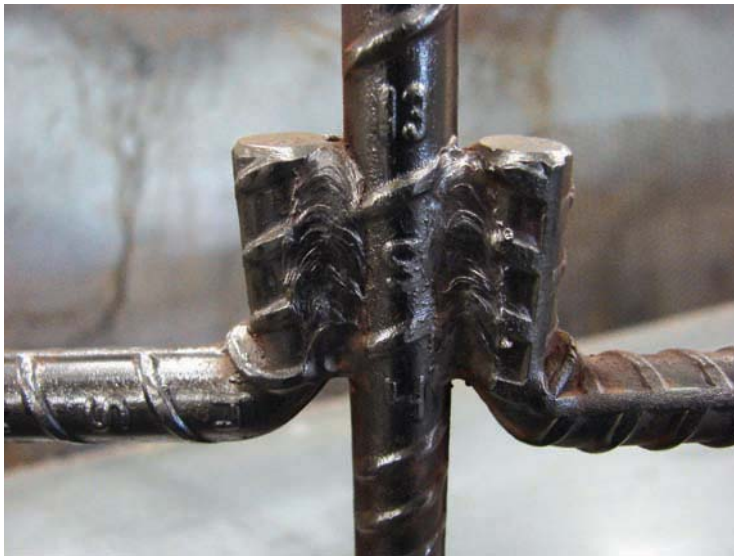
Figure 10-8. Center arms welded to main pole.
