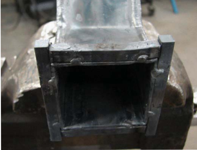
Figure 7-36. Front and back side rims attached. The parts will look rough at this point, but it's nothing that a little cleanup can't fix.
