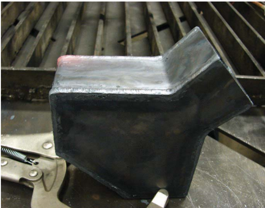
Figure 7-31. Weld the upper section of the 90-degree angled part..
