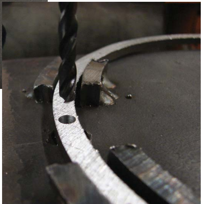
Figure 12-9. Checking for hole centering after drilling the first hole.
