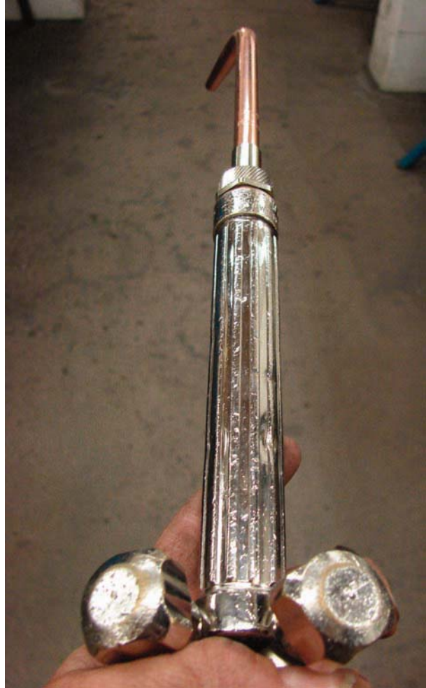
Figure 2-8. Figure 6-11. Pointing the torch in the direction of the weld will provide a comfortable hold while welding.
