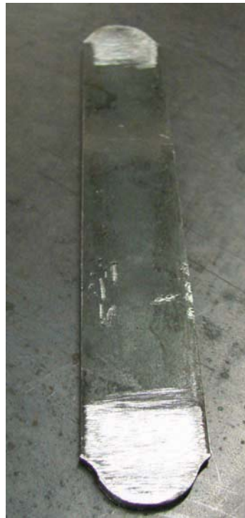
Figure 9-8. The body front, top cap rounded and ready to be cut to size.
