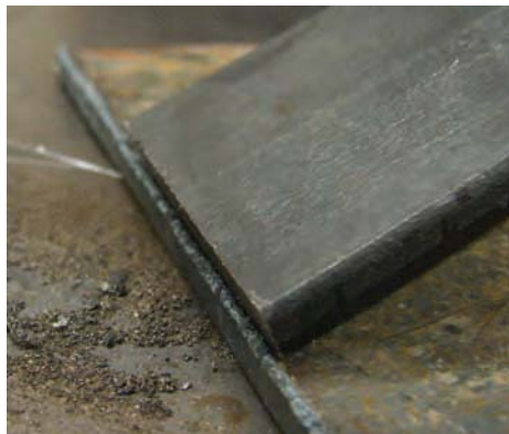
Figure 1-17. Removing dross from plasma cut steel with flat bar.
