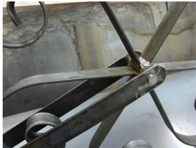
Figure 13-35. Attaching the axle through the front wheel and fork.
