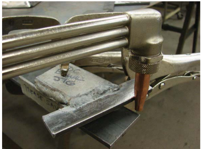
Figure 4-6. a) Plan views of the cutting torch jig used to cut the angled sides. b) Constructed jig, clamped to 1/4" x 2" flat bar, ready to be cut.
