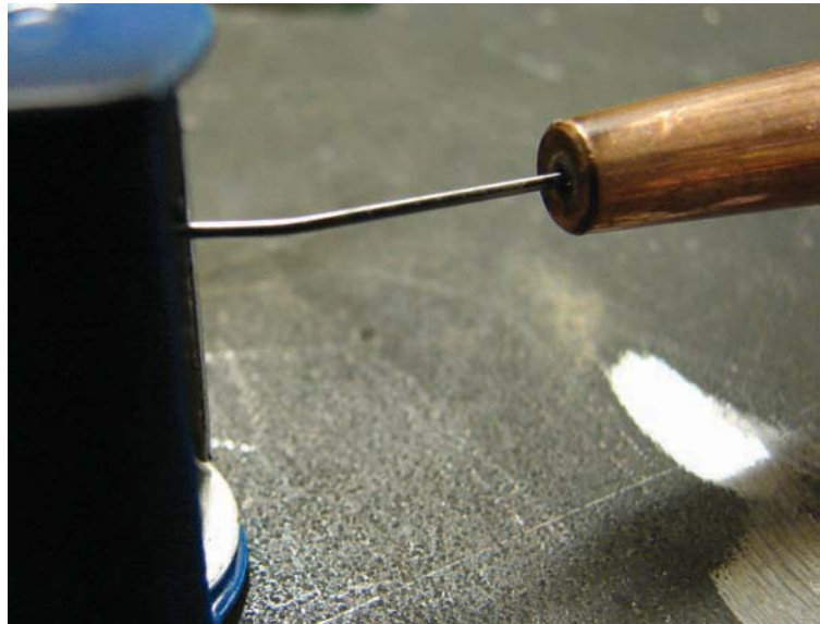
Figure 7-19. Cleaning a tip before every use is very important. Dirty tips produce uneven and a hard to maintain flame.
