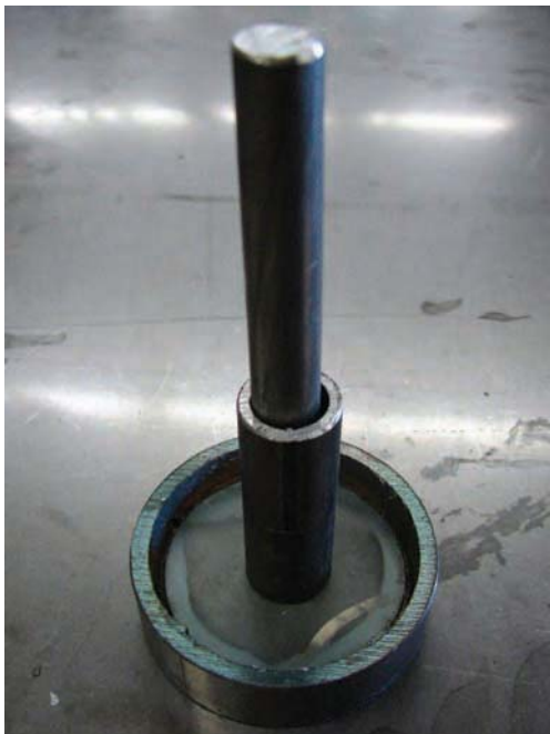
Figure 1-35. Axle through the wheel center and axle supports slid onto axle.
