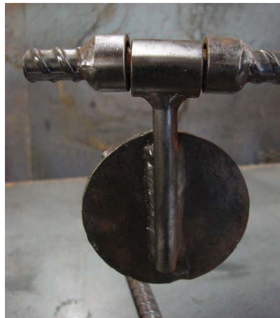
Figure 10-13. Lower target welded and attached to target framework.
