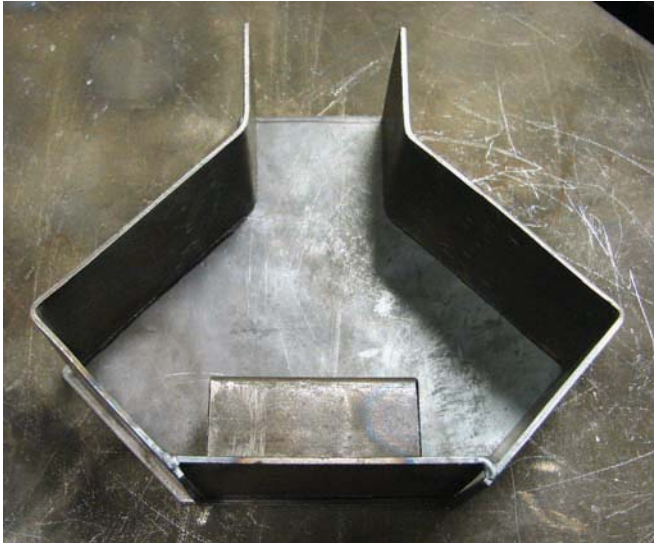
Figure 7-20. Tack the bottom to the sides in the top corners.
