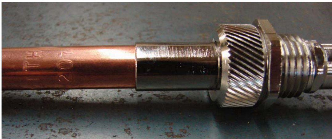
Figure 6-10. The gas torch should be tightly screwed into the torch head to prevent gases from leaking out of the fitting.
