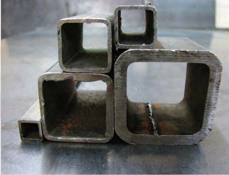
Figure 1-1. a. Square tube is identified by height, width, and thickness. Example: 1" x 1" x 10ga sq tube.
