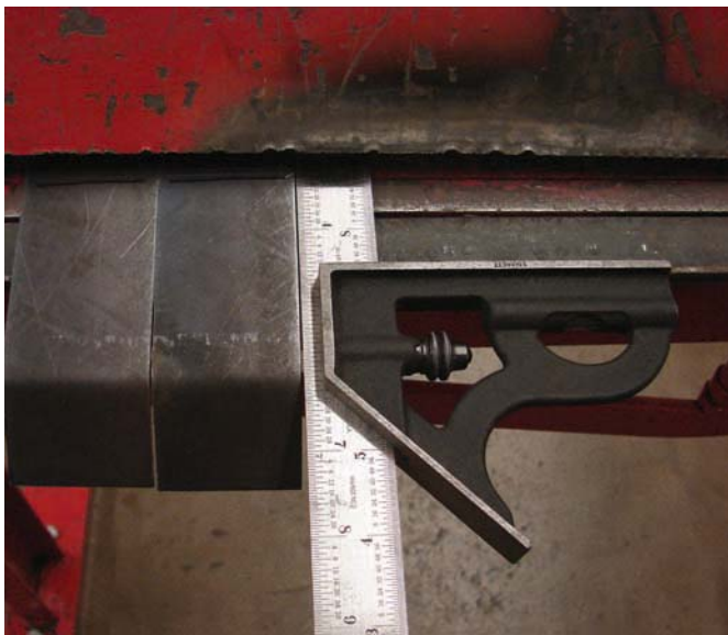
Figure 7-12. Preparing to make the 90-degree bend in the two side parts.
