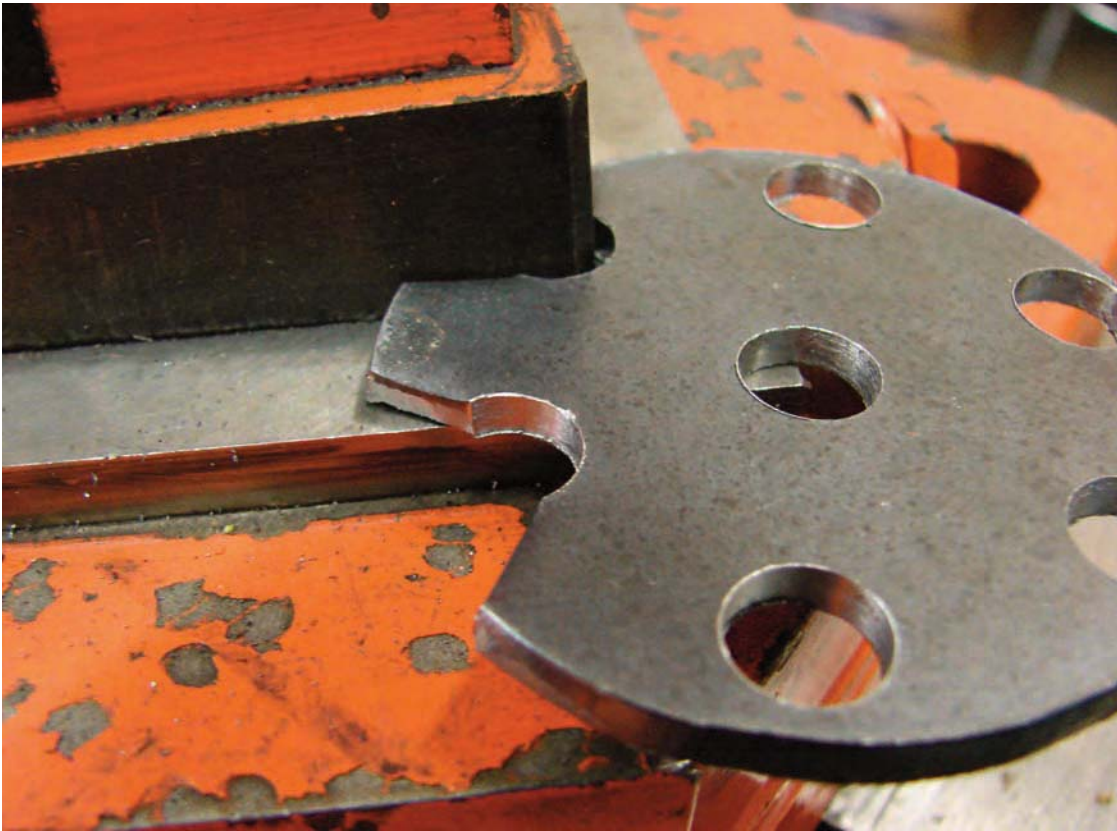
Figure 9-19. A notcher attachment on an iron worker can make finishing the spokes on the large tire centers quick and easy.
