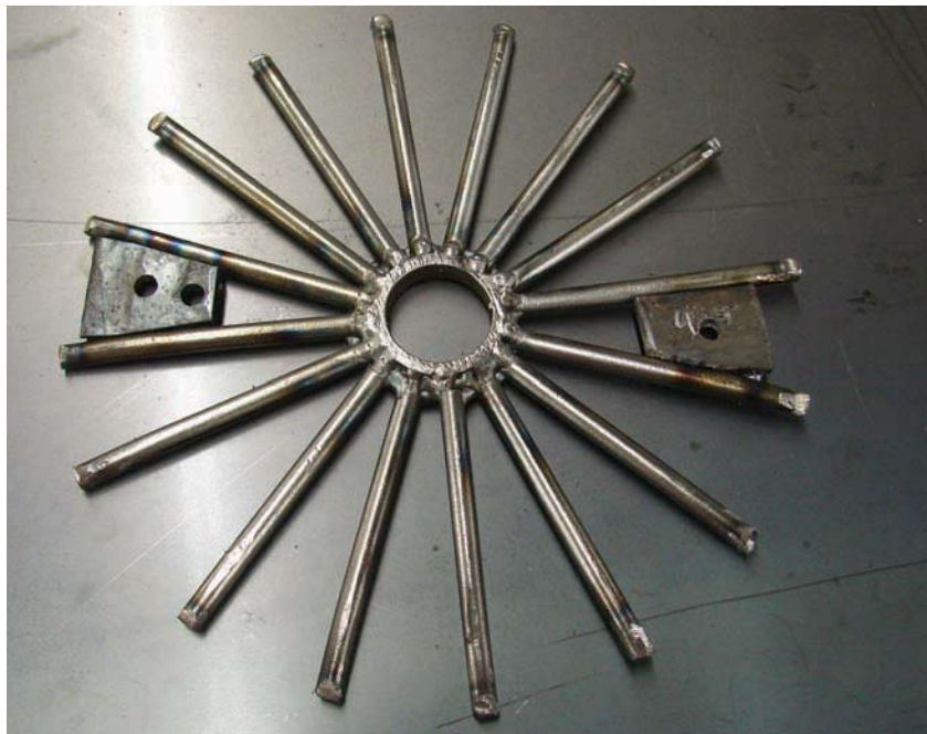
Figure 12-33. Tabs welded to the bottom spokes.
