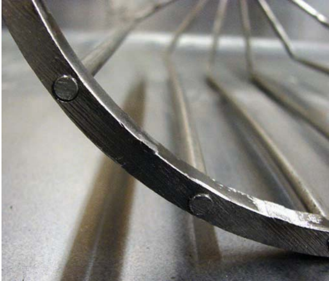
Figure 12-27. Bottom side of the bottom outside ring after the side spokes have been inserted.
