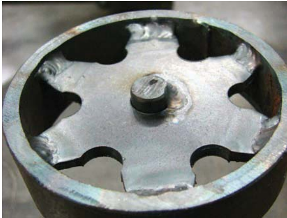
Figure 9-44. Large tire axle tacked to large tire center.
