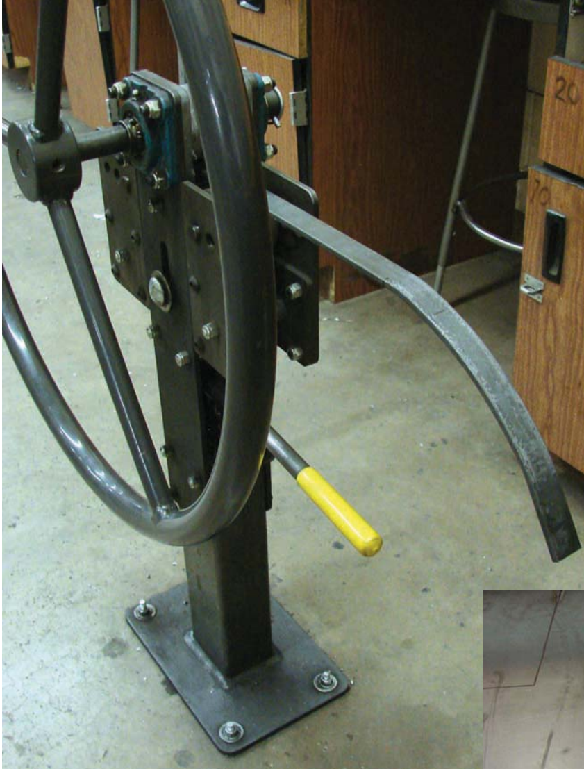
Figure 13-24. Ready to bend the second arc in the connector arm.
