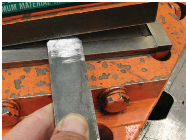
Figure 9-9. A metal shear provides a quick option for cutting the small part to size with no additional clean-up necessary.
