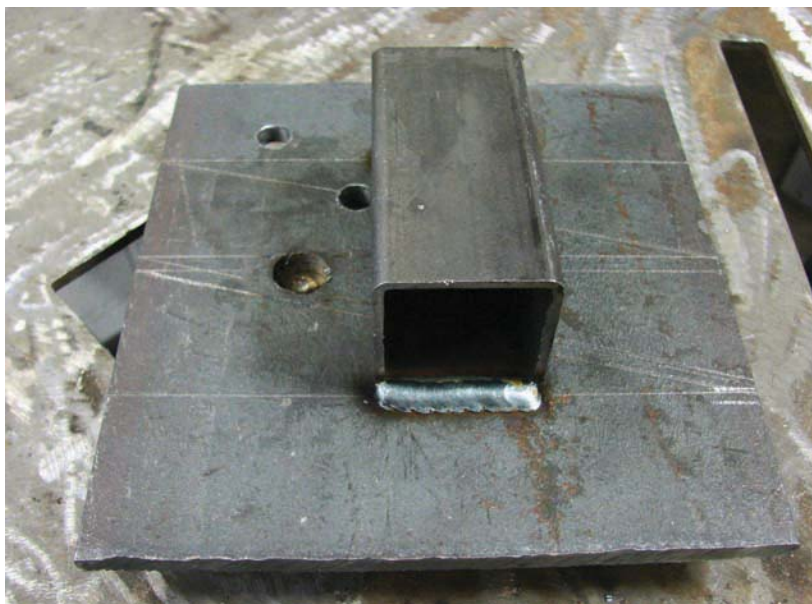
Figure 11-12. Square tubing welded to the bottom of the jig. Notice, only the ends were welded. Welds on the sides can affect how flat the jig will set in a vise.
