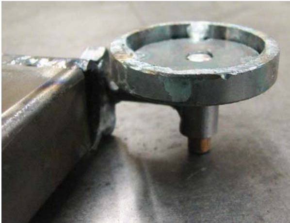
Figure 9-41. The first small tire in place and ready to be welded to the axle.
