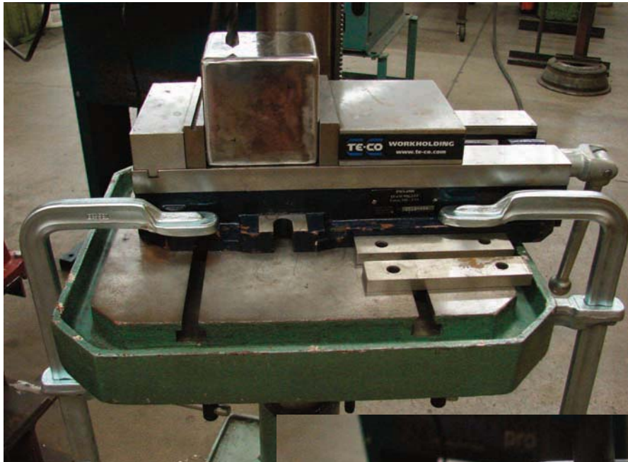
Figure 6-27. Dice in position and ready for the first corner hole to be drilled with the vise secured in place with two clamps.
