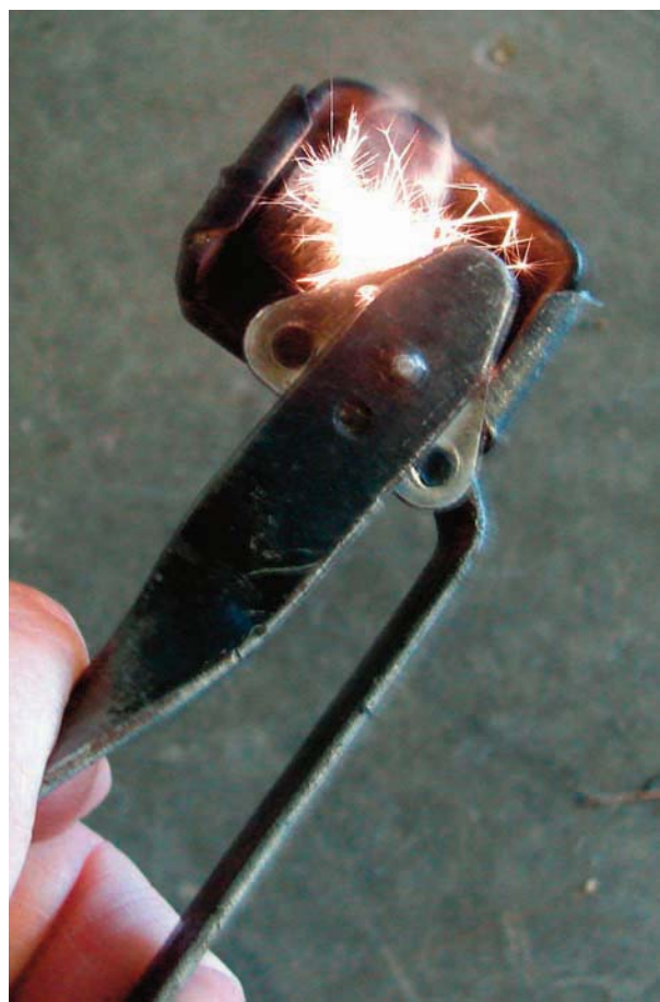
Figure 6-5 b) Keep the striker in good condition so that it produces a strong spark.
