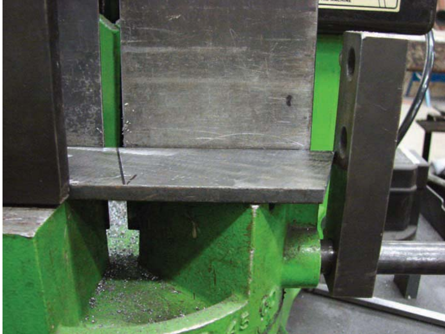
Figure 4-5. A band saw parts stop allows for multiple parts being cut the same length, quickly and accurately.
