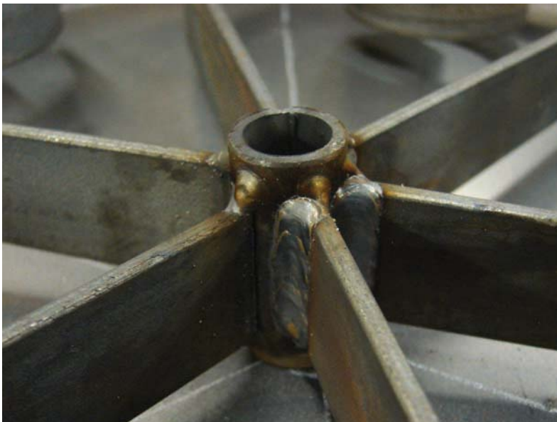
Figure 13-21. Axle support centered and welded to the large wheel spokes.
