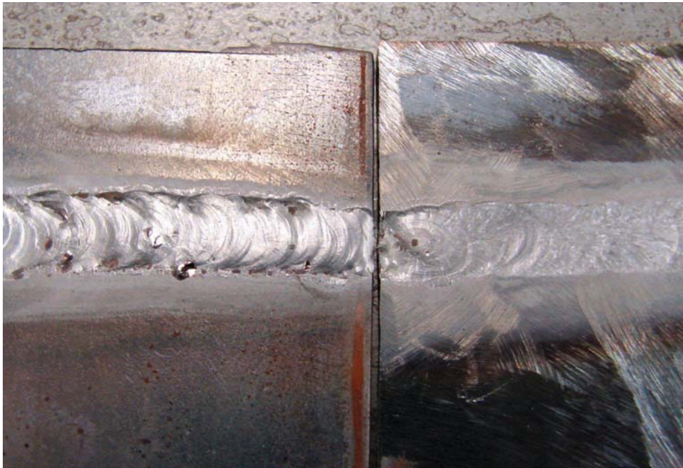
Figure 8-3. Notice the smoothness of the puddle on the right; it was pushed on clean steel compared to the puddle on the left, which was pushed on rusty unpolished steel.
