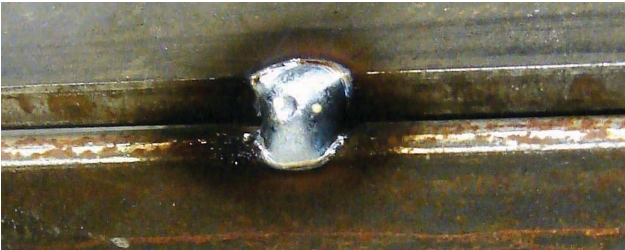
Figure 2-9. Example outside corner joint.
