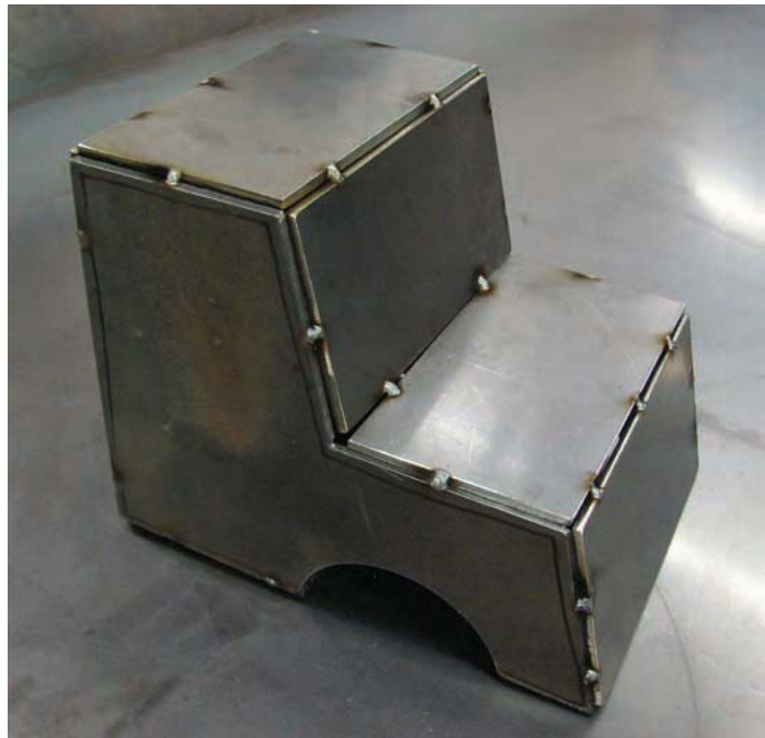
Figure 1-22. Truck cab tacked and ready to be welded solid.
