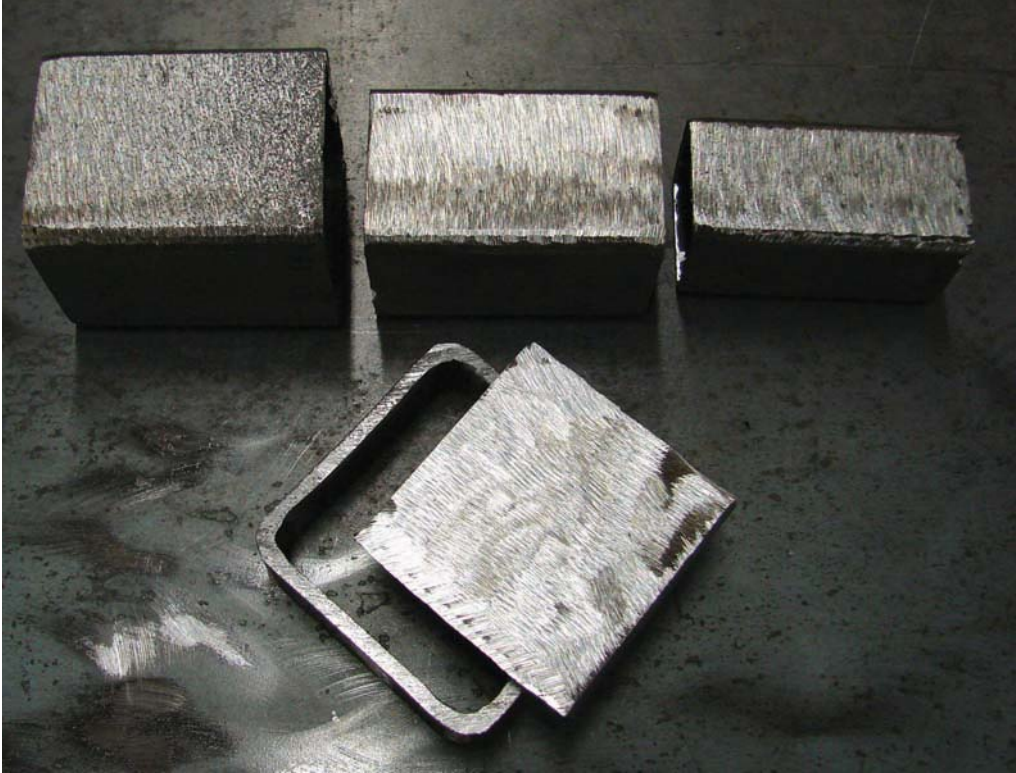
Figure 8-2. Parts cut to size with all rust and mill scale removed using an angle grinder.
