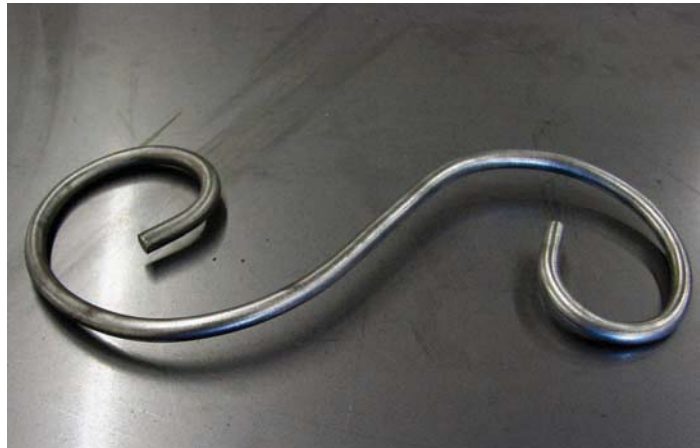
Figure 11-26. This part was not placed in the bender correctly and as a result has a slight arch in the middle.
