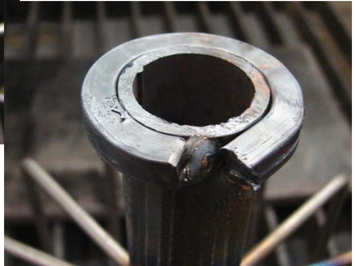
b) Excess rim material removed.
