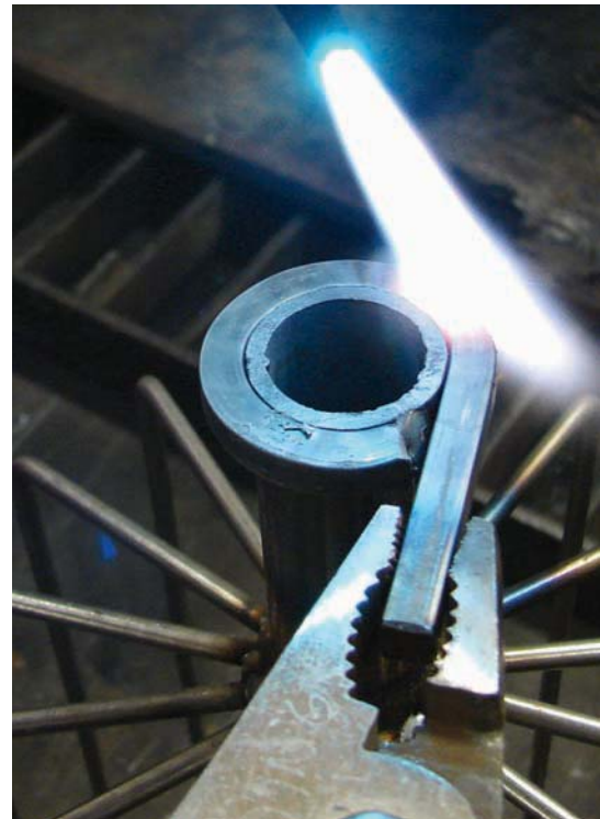
Figure 12-31. a) Beginning the bend. b) Rim almost around the spout with a tight fit between the two parts. c) Bending complete.
