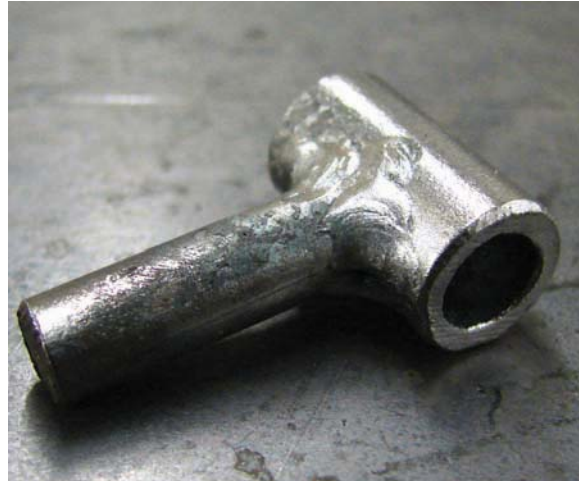
Figure 9-39. Completed welds on the axle and support parts.
