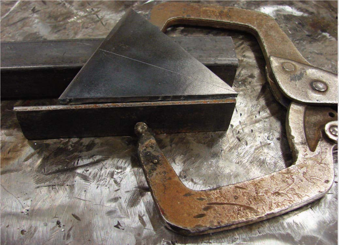
Figure 2-13 a) Use 1"x 1" sq. tube and locking C-clamp pliers to align the hitch parts before tacking.
