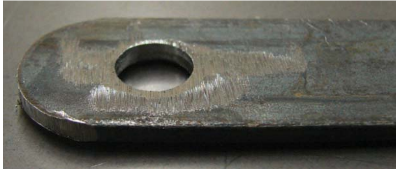
Figure 13-30. Completed end on the front wheel fork.
