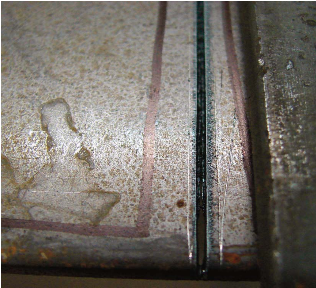
Figure 6-2. In this example, the kerf is correctly centered between the scribed lines.
