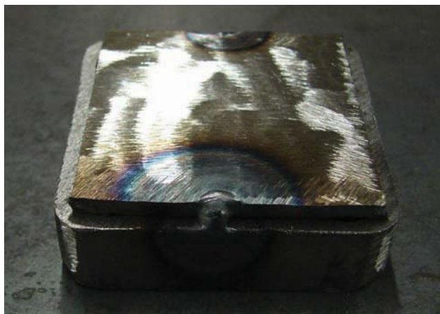
Figure 8-10. Base top attached to the base bottom with two small tacks on each side.
