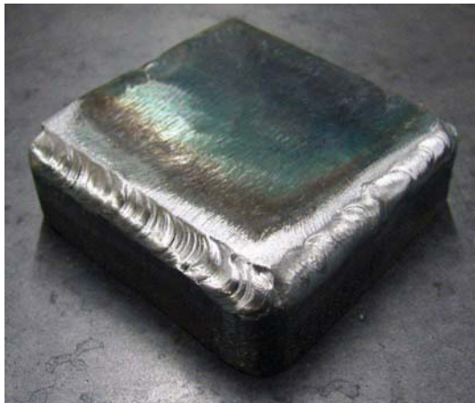
Figure 8-11. Outside corner welds completed on two sides of the bottom base using 1/8" filler rod.
