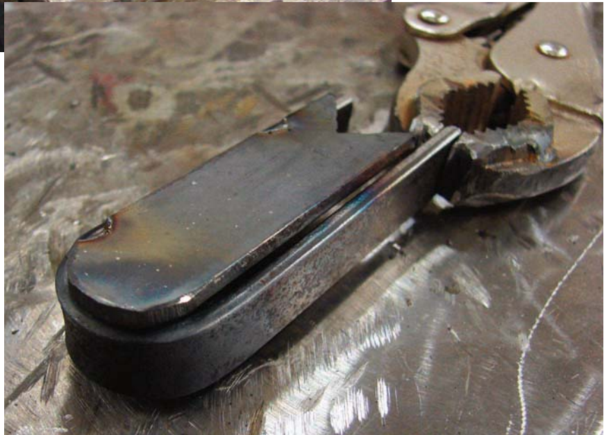
Figure 2-19. a) Tongue parts removed from the vise and ready for final bending. b) Completed bend on tongue side. Notice the proper outside corner alignment.
