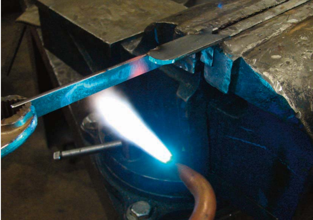
Figure 2-17. Heating the tongue side so that it can be bent around the front of the tongue top.
