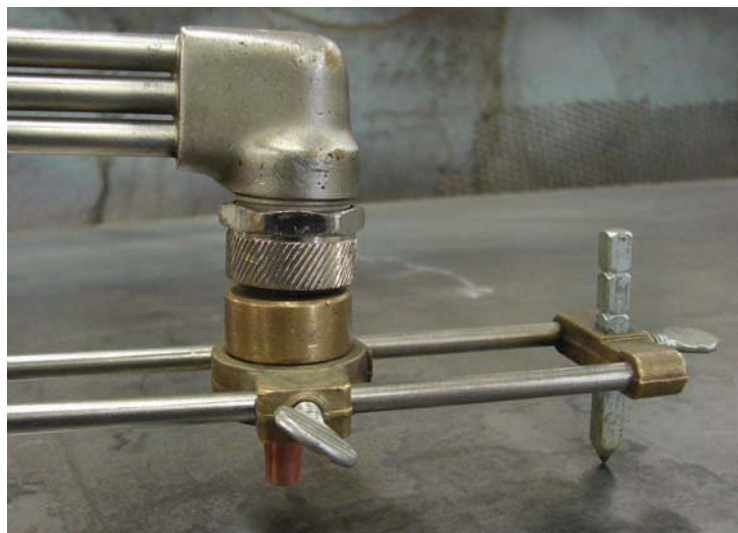
Figure 10-11. Circle cutting attachment for a cutting torch.
