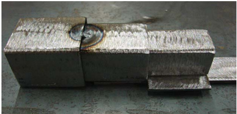
Figure 8-8. Center and bottom tubes ready to be tacked.
