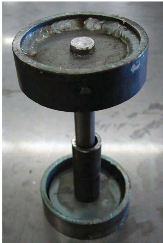
Figure 1-36. Wheel assembly slid together.
