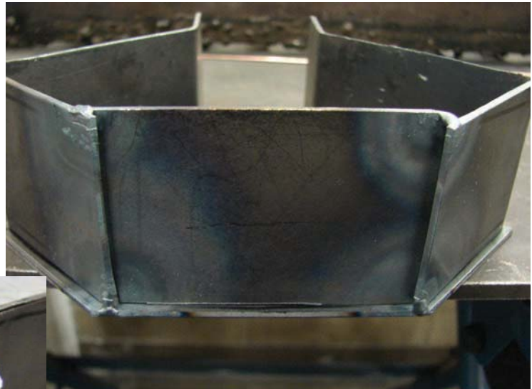
Figure 7-22. Tacks joining the bottom face to both sides.
