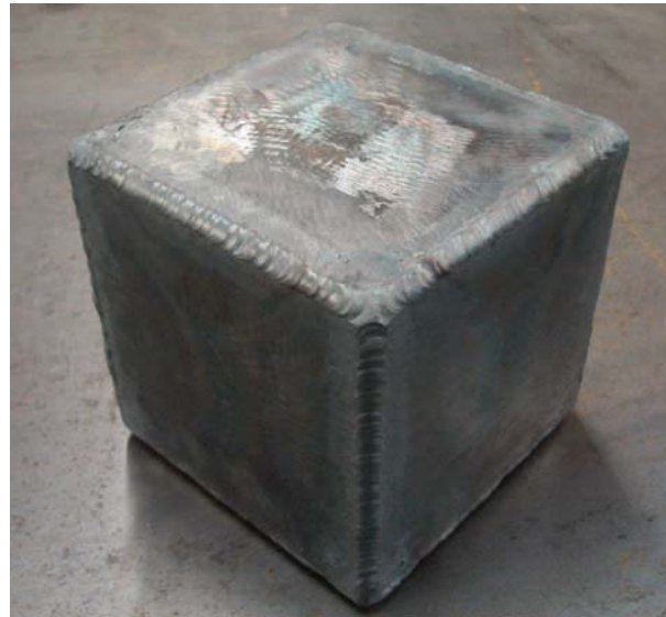
Figure 6-22. Finished cube before polishing and adding the holes. Corners are closed and free from holes. The outside edge joints are filled and the weld has evenly spaced ripples.
