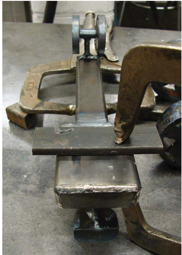
Figure 9-46. Use locking pliers to aid in accurately placing the axle support.
