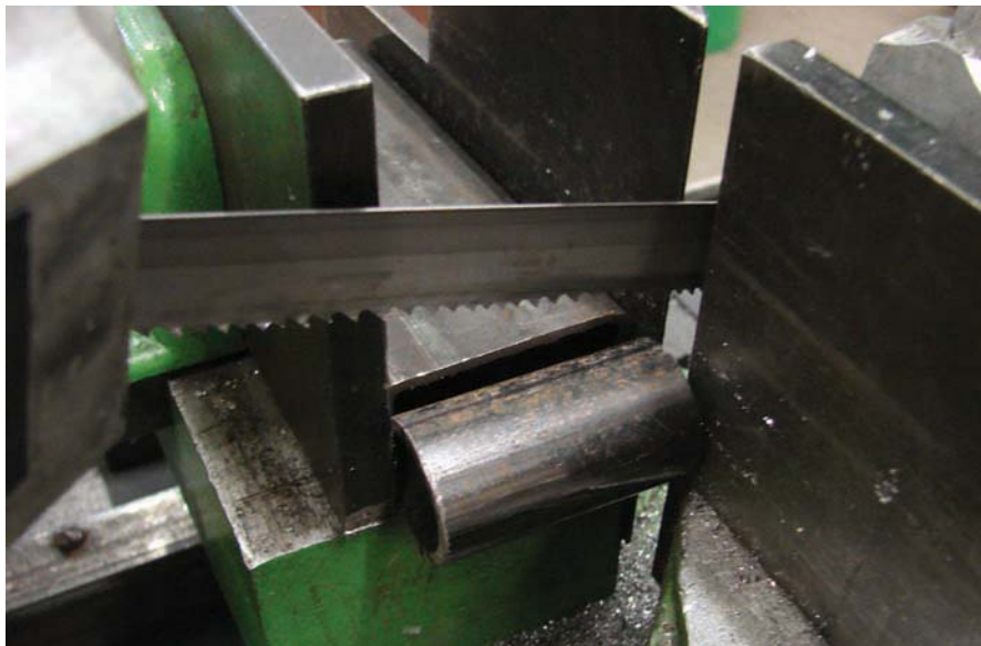
Figure 9-4. The body front secure in the vise and ready to be cut in half using a band saw.
