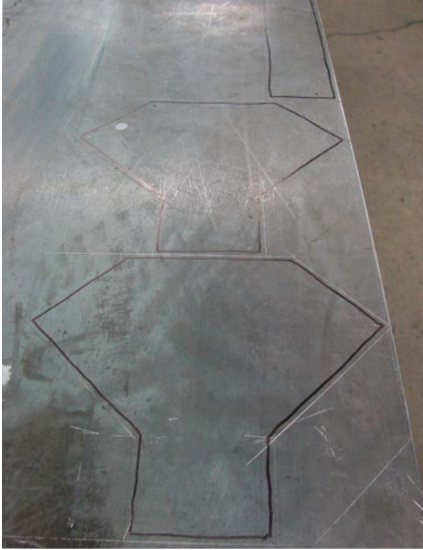
Figure 7-3. When using a permanent marker to help locate lines, make sure to stay inside the lines. Drawing on the lines will make the lines difficult to see and defeat the purpose of using the marker.
