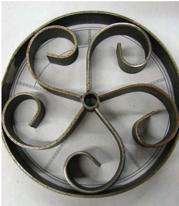
Figure 13-16. Spokes trimmed and ready to be welded.
