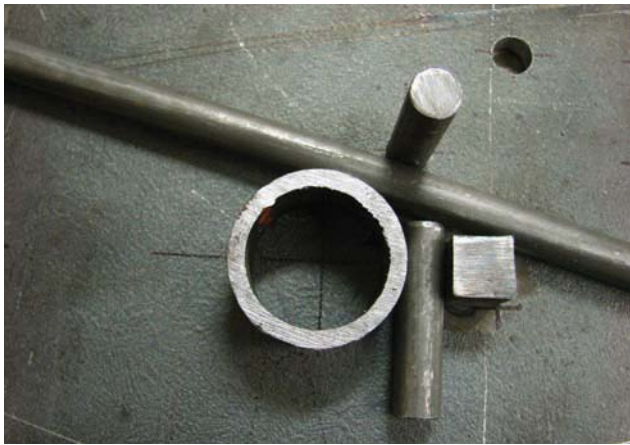
Figure 11-10. Align the pipe in the proper location using the previously cut 3/8" rod.
