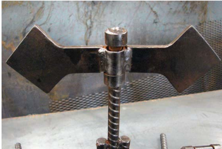
Figure 10-12. Upper target welded and attached to target framework.
