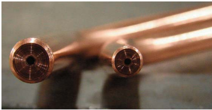
Figures 6-6. a) The orifice of a 207 and 205 Smith gas welding tip. The larger the orifice, the more gas that is released and the hotter the flame. b) 205 and 207 Smith gas welding tips.
