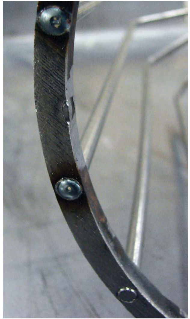
Figure 12.28. Tacks on bottom ring used to hold the side spokes in place.
