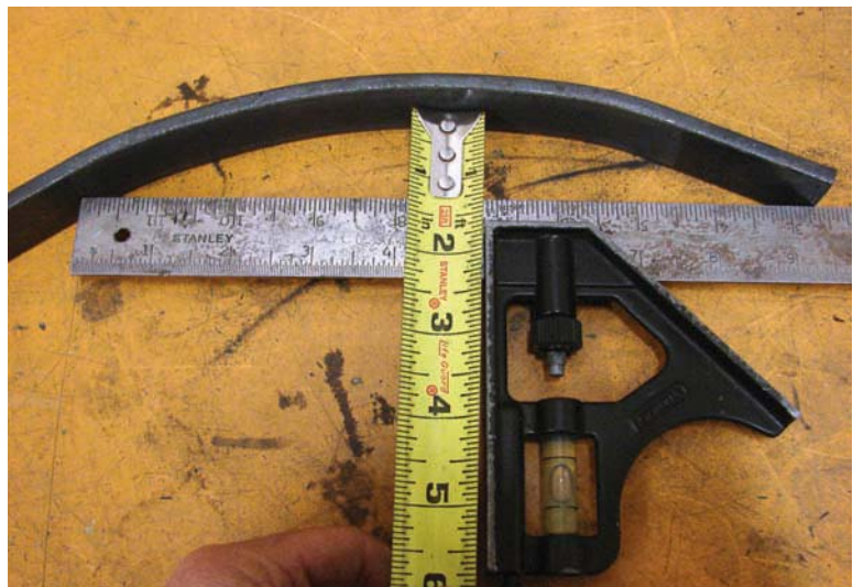
Figure 13-23. Checking the arc bend.
