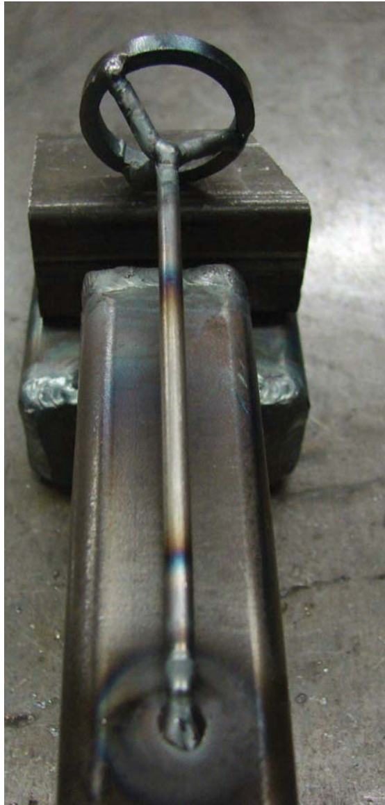
Figure 9-30. Steering bar attached to the main body with a small tack weld.
