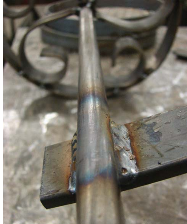
Figure 13-40. a) Tacked connector arm. b) Connector arm welded to the back axle.
