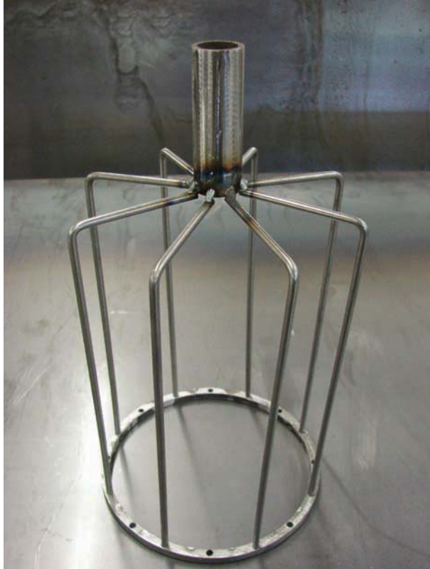
Figure 12-25. The first 8 spokes tacked in place.
