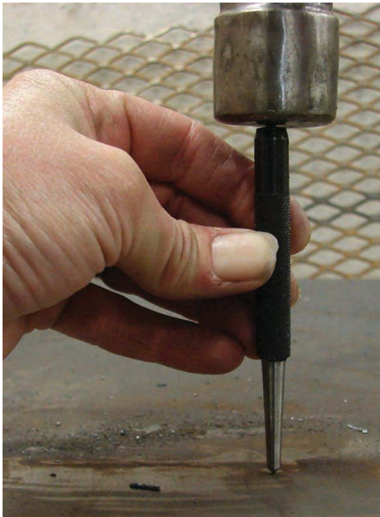
Figure 1-12. Using a punch and hammer to mark circle centers requires a solid surface and a steady hand. When making your punch mark, hit the punch one time only. Back to back hits can give you two divots. If the divot is not deep enough from the first hit, reset the punch and then strike again with a single blow.
