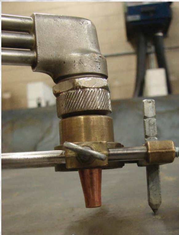
Figure 3-10. a) Use a ruler to set your radius for the circle cutting attachment. Measure from the pivot point to the outside of the center oxygen orifice.
