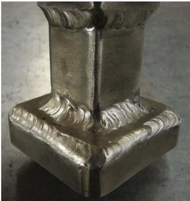
Figure 8-13. Completed T-weld at the base of the pencil holder.
