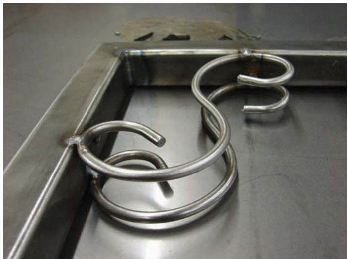
Figure 11-27. Wrought iron parts welded in place.
