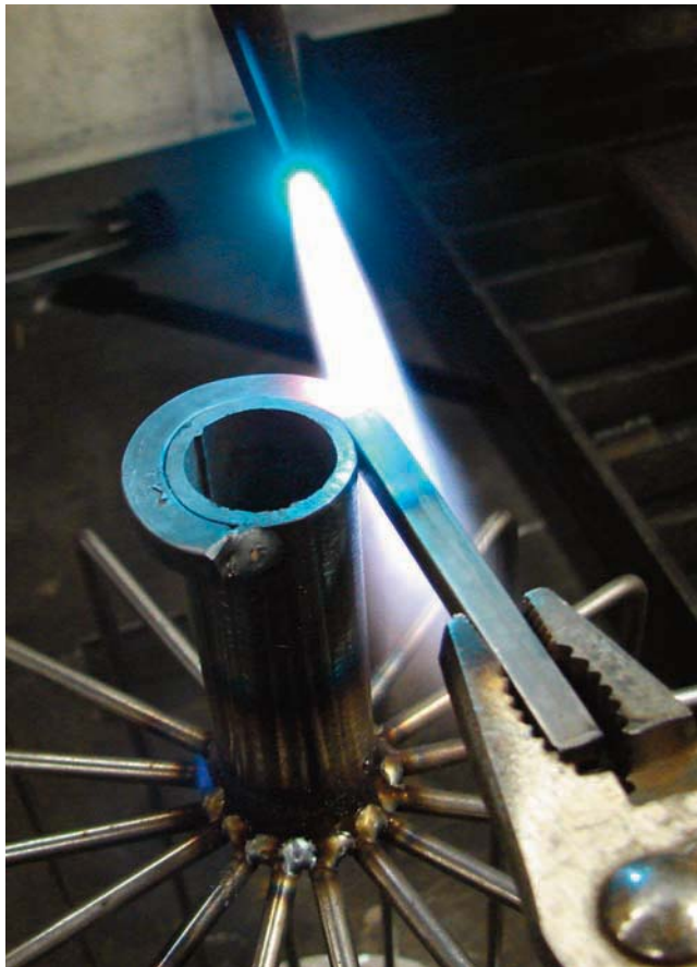
Figure 12-31. a) Beginning the bend. b) Rim almost around the spout with a tight fit between the two parts. c) Bending complete.
