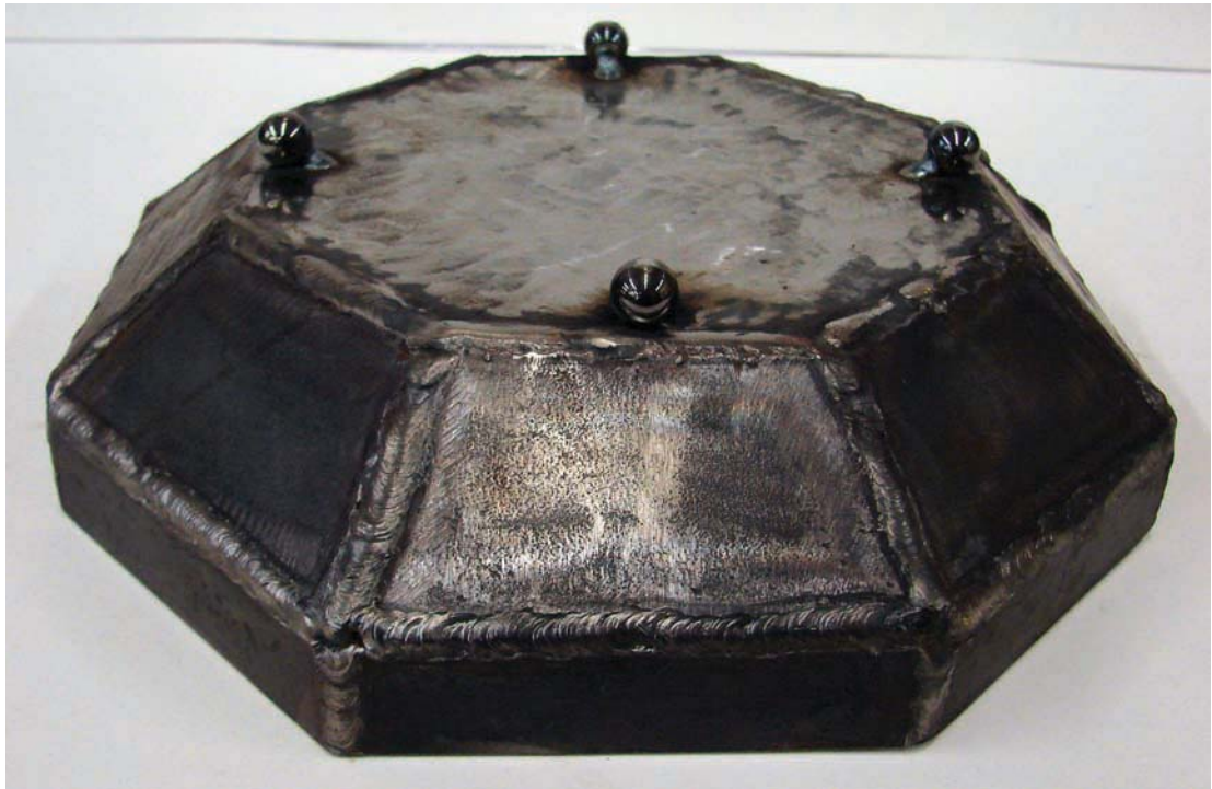
Figure 4-13. Steel balls attached with strong solid tack welds.
