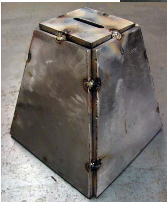
Figure 3-20. Check for clearance so that the bank will sit flat on all four sides rather than resting on the mushroomed pin.
