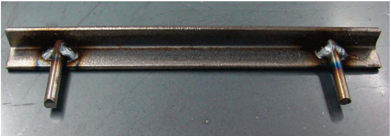
Figure 2-24. a) Bumper mounts in place and ready to be tacked. b) Attached bumper mounts.
