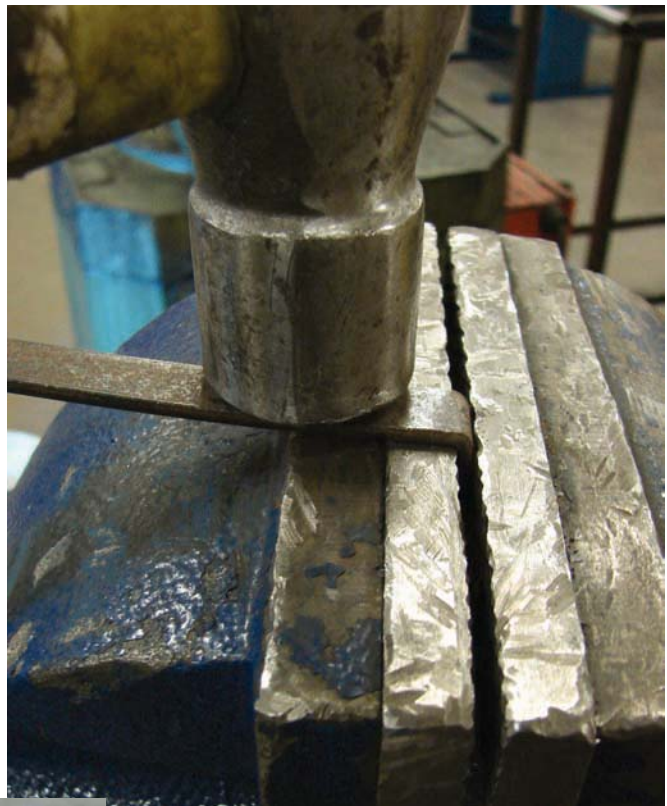
Figure 9-51. Hammering the angle on the rear hitch
