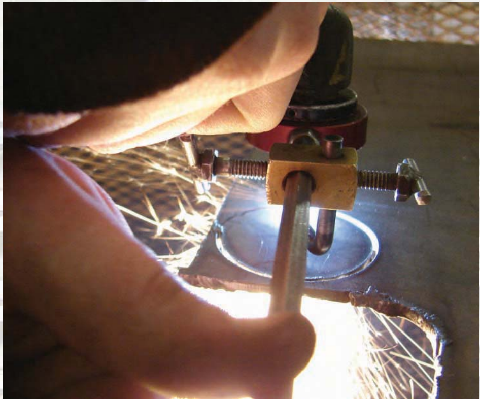
Figure 1-13b. Cutting a circle with a plasma circle cutting at- tachment.
