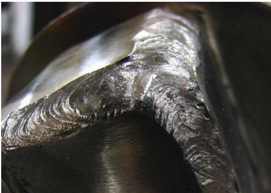
Figure 5-6. Completed weld intersection.
