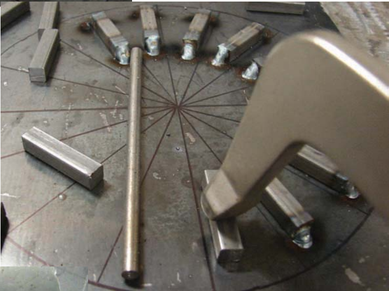
Figure 12-13. a) Attaching the stops on Jig #2. b) Completed Jig #2.
