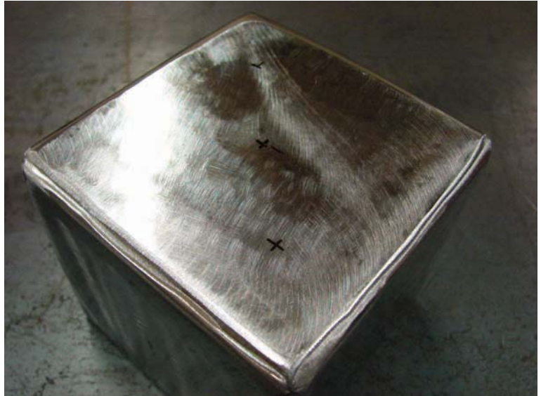
Figure 6-25. The number three hole positions marked with a permanent marker.
