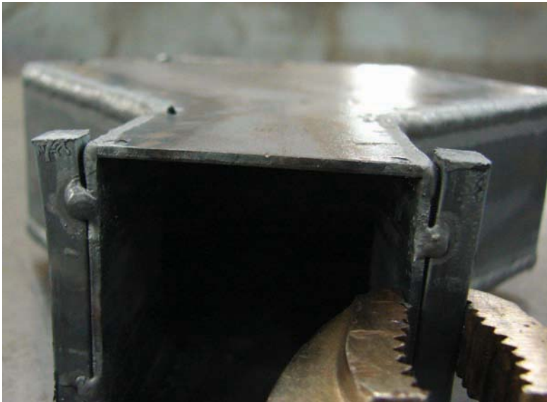
Figure 7-35. Side rims attached.
