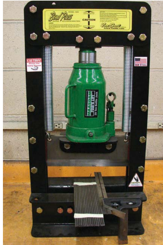
Figure 12-17. Metal bending brake press.
