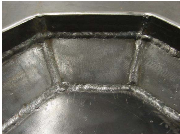
Figure 4-11. Inside welds of the bowl.
