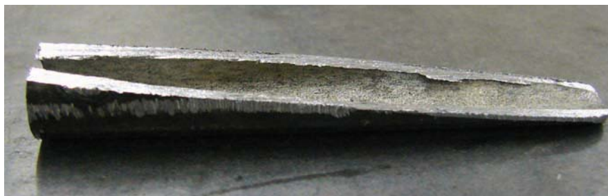
Figure 9-31. a) Tack the 1/8" sch40 pipe to a scrap piece of rectangular tube. b) Turn the tubing over and place three strong tacks on the back side. c) Place the part in the band saw and split it in half using approximately a 7° angle. d) Remove any sharp edges and excessive mill scale from the half section of pipe.
