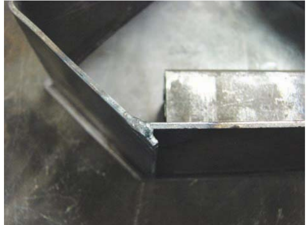
Figure 7-21. A small but strong gas weld tack.
