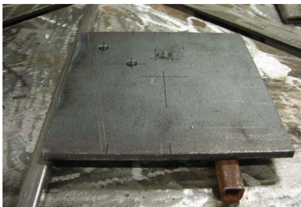
Figure 11-8. Preparing to tack the square bar to the plate.
