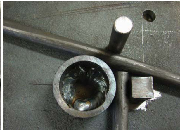
Figure 11-11. Pipe welded securely to the plate.
