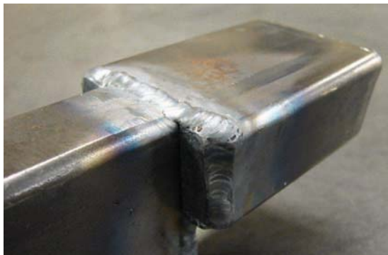
Figure 9-15. Final welds made to the main body of the tractor.
