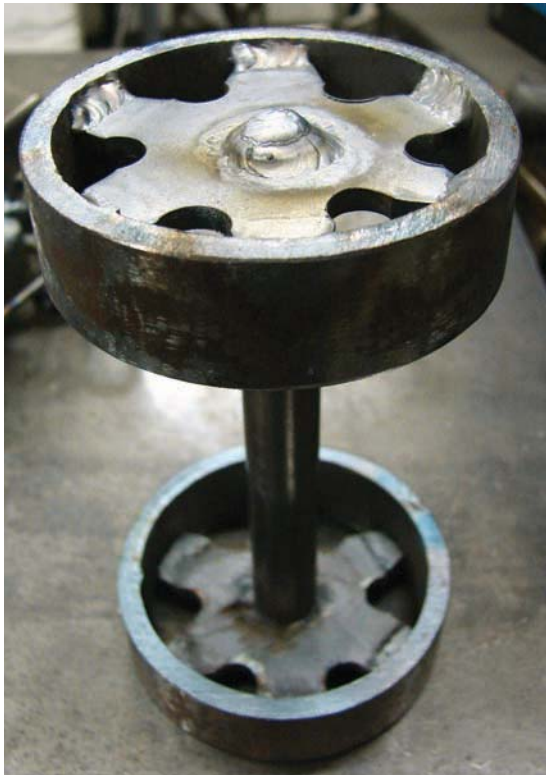
Figure 9-45. Completed large tire axle assembly.
