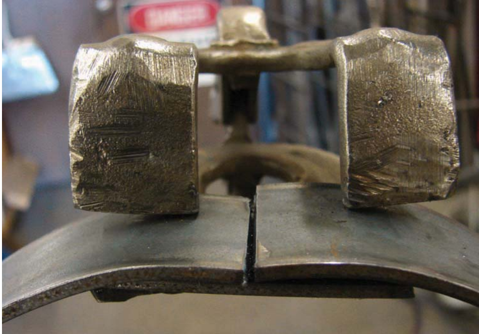
Figure 13-11. Use u-shaped locking pliers to hold the ring while welding the butt joint.
