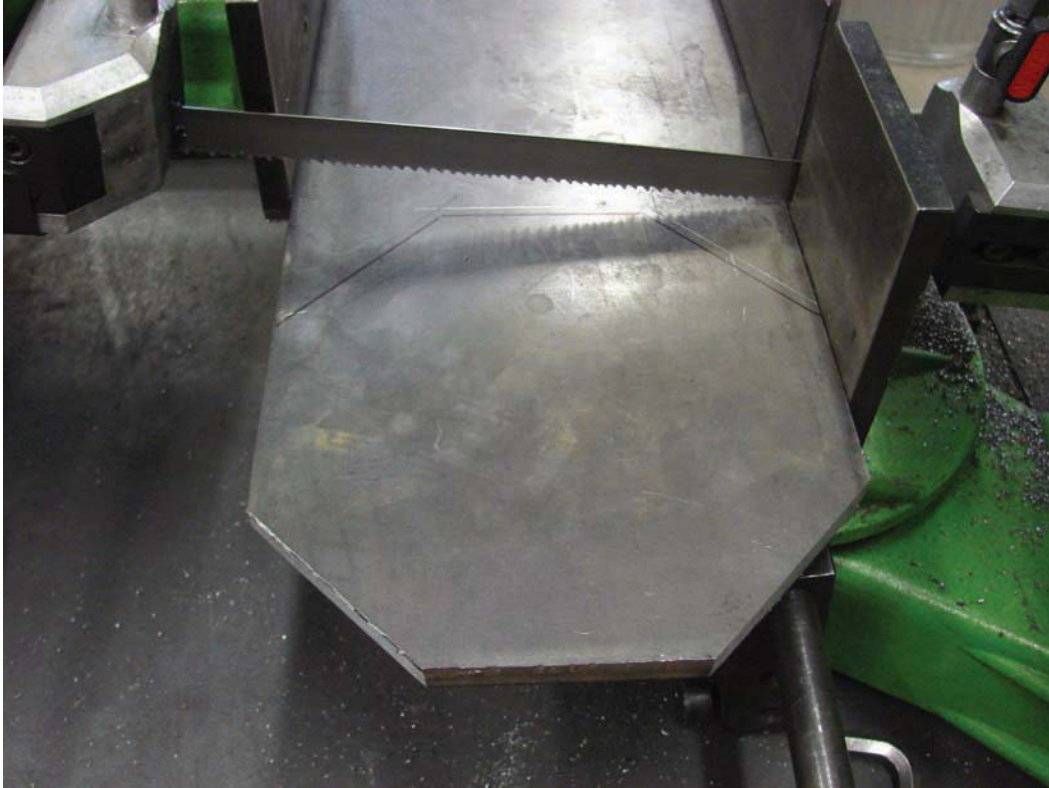
Figure 4-3. This octagon was cut from some scrap material that just happen to be 6-5/8" wide. The first two corners were cut off first; then the width was cut, and finally the last two corners.
