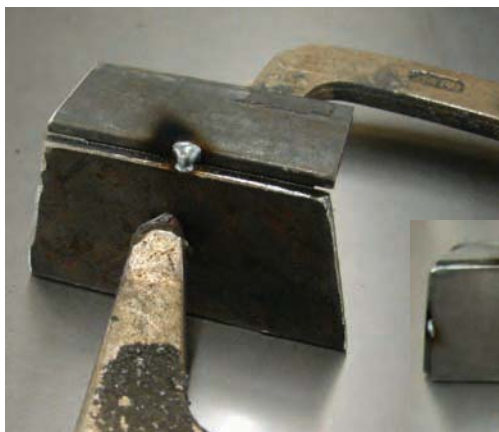
Figure 1-28. a) Use locking pliers and 1"x 1" square tubing when tacking the hub parts.
