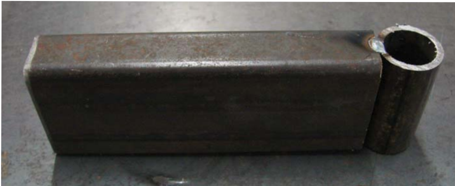
Figure 9-3. The body front tacked securely to rectangular tube.
