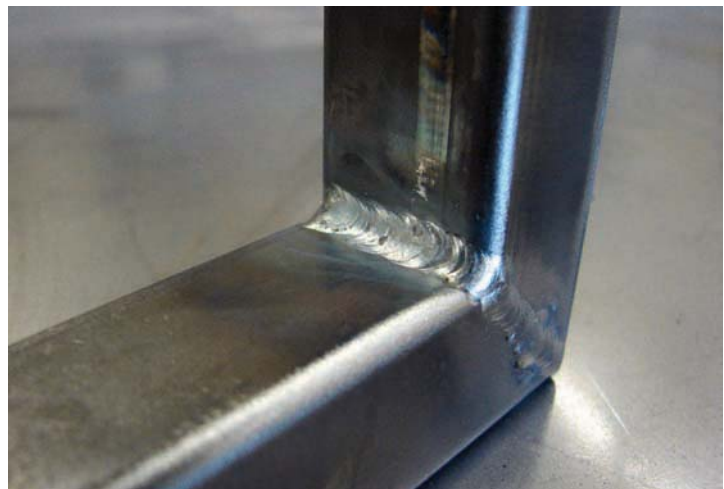
Figure 11-4. Supports welded using the TIG welding process.
