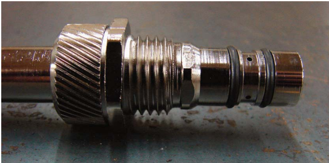
Figure 6-9. The O-rings on a gas torch tip should be inspected prior to using.
