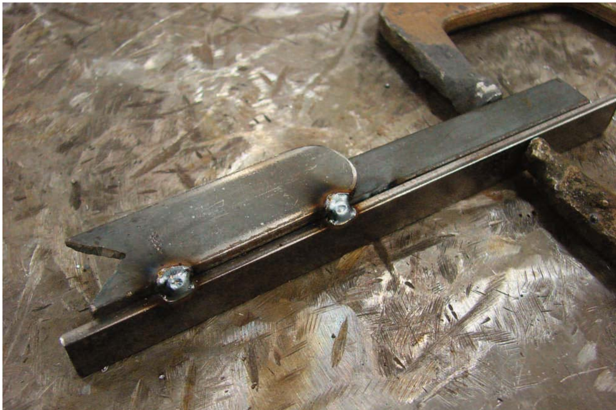
Figure 2-16. Tongue top and sides tacked and ready for bending.
