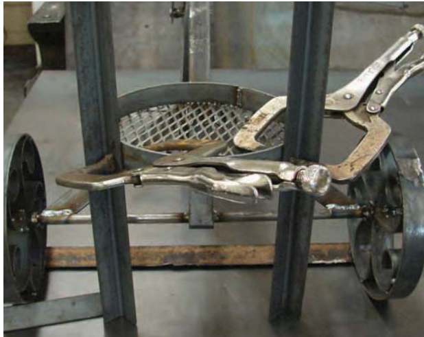
Figure 13-43. a) Positioning the lower, bottom plant holder ring. b) Centering the lower, bottom plant holder ring.
