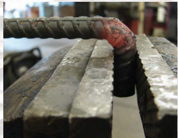
Figure 10-6. a) Heating the rebar with a cutting torch. b) Rebar bent at a 90-degree angle.
