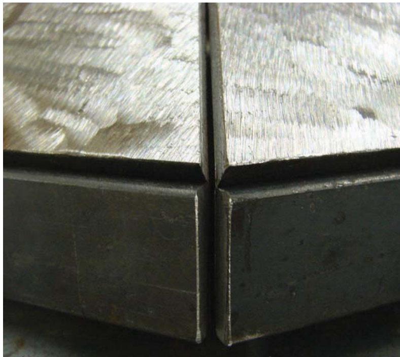
Figure 4-10. Outside corner joints of bowl ready to be filled with weld.
