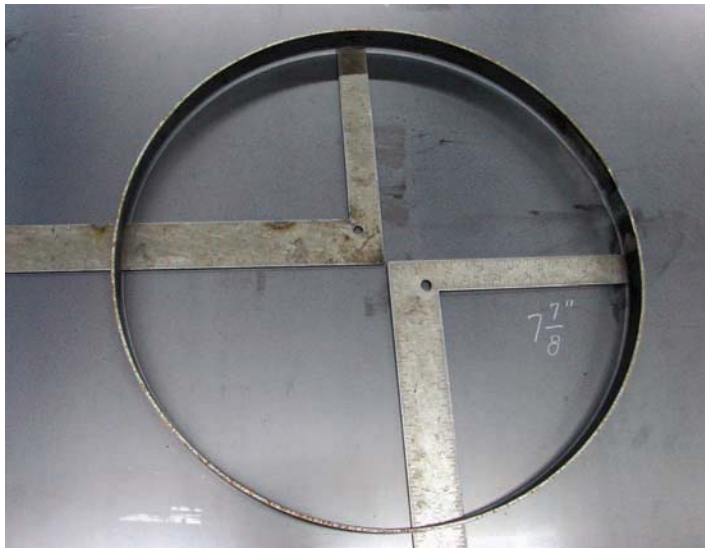
Figure 13-18. Use framing squares to mark the center and draw a line dividing the circle.
