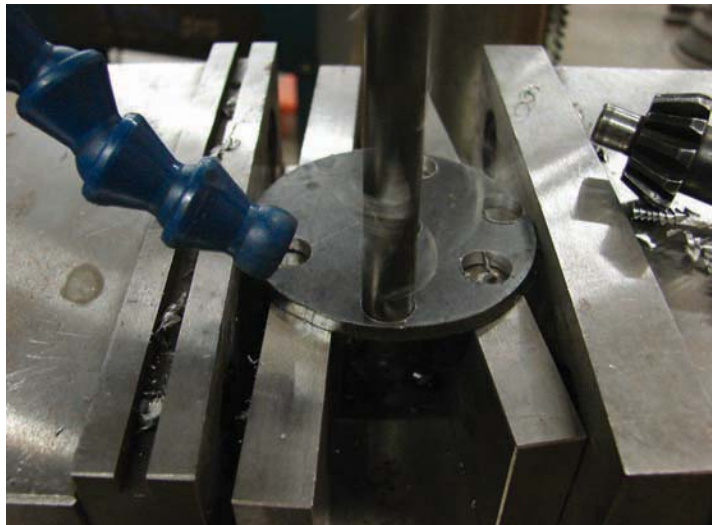
Figure 9-17. Drilling the holes in the large tire centers.
