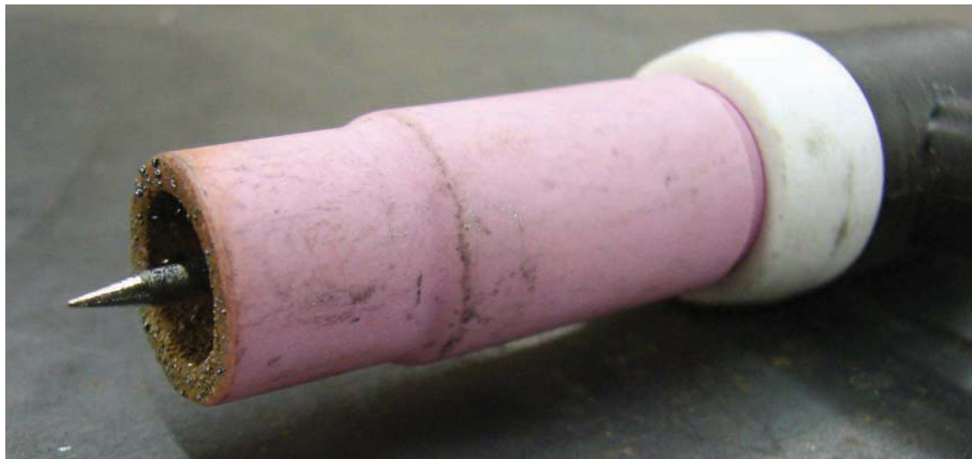
Figure 8-4. TIG nozzle and properly pointed tungsten electrode.
