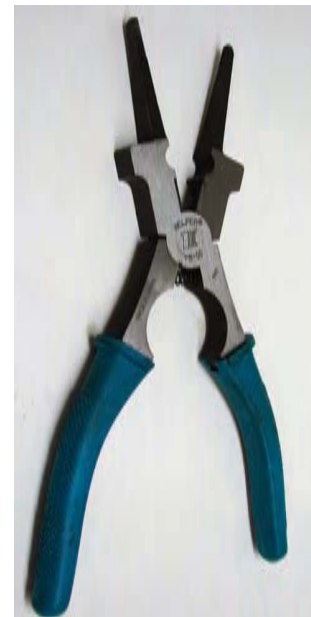
Figure 1-25. a) Clean the nozzle regularly to allow maximum gas flow from the nozzle. b) MIG pliers are specially designed to help you tighten or remove consumable parts in the wire feed gun, clean the nozzle, and clip wire.
