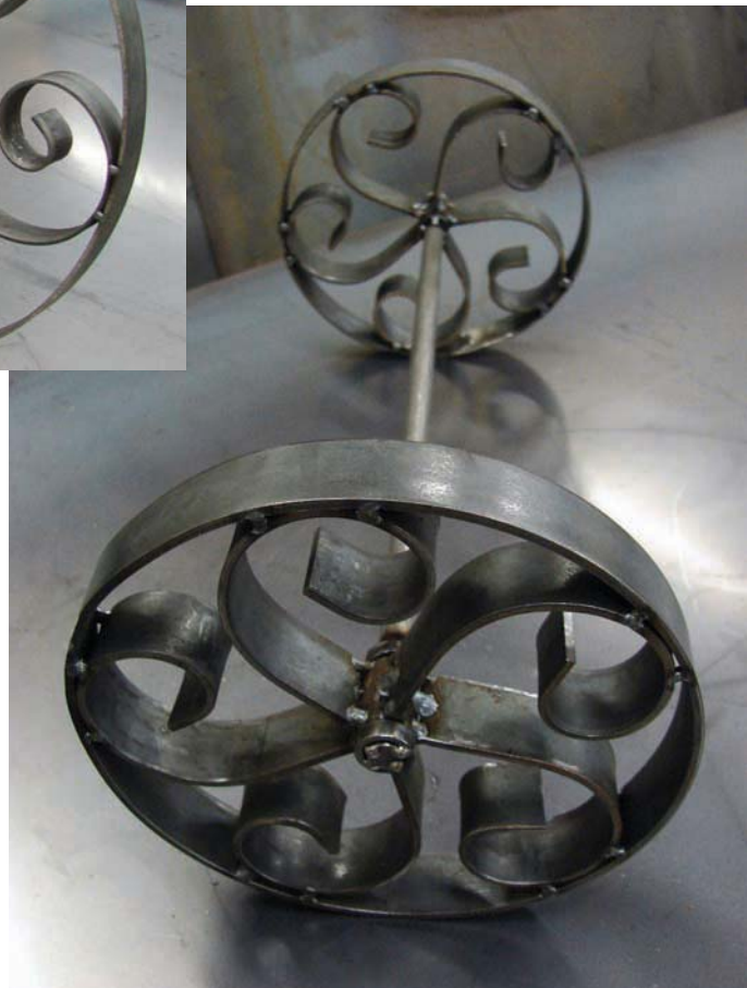
Figure 13-37. Completed back wheel and axle assembly.
