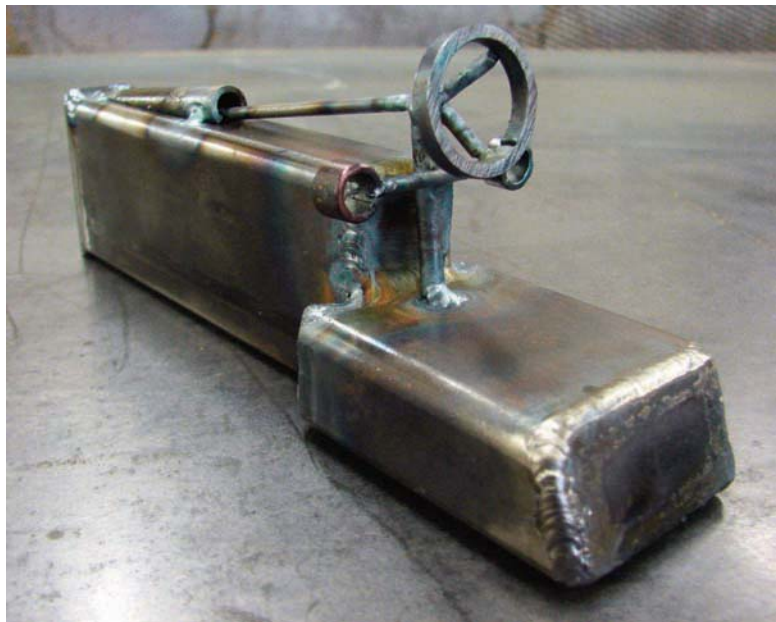
Figure 9-33. Attached steering support.
