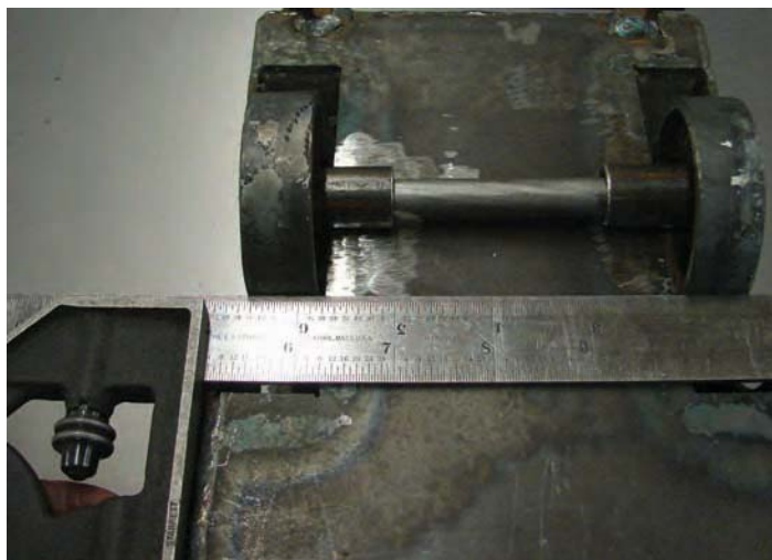
Figure 1-38. Use a square to position your wheel assembly on the truck properly.
