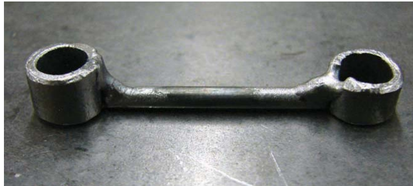
Figure 9-27. Finished light bar.
