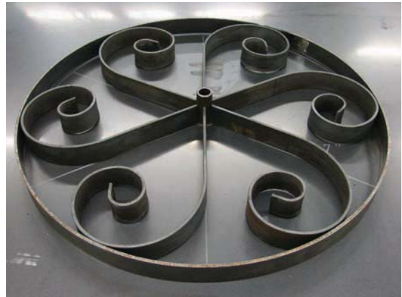
Figure 13-20. a) Lay out each spoke one at a time and mark where it needs to be trimmed. b) Large wheel spokes trimmed and in place.
