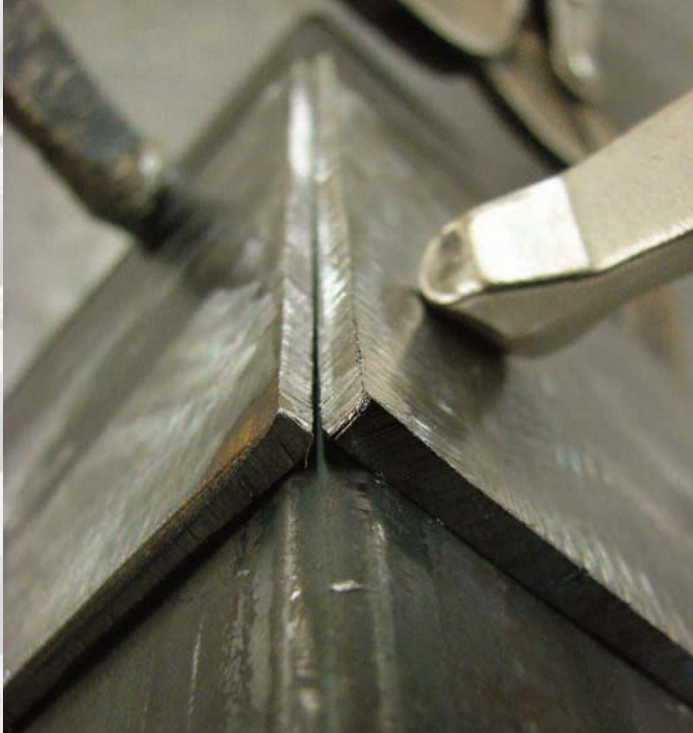
Figure 6-14. Properly aligned outside corner joint.
