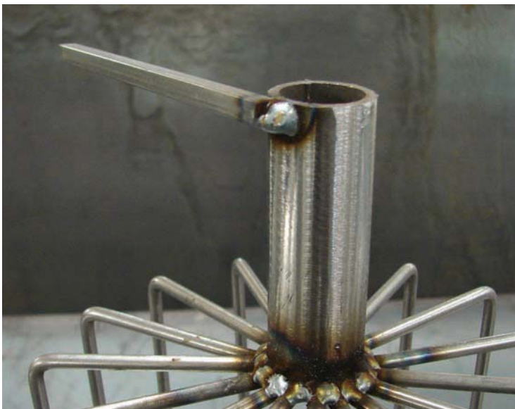
Figure 12-30. Spout rim tacked to the spout.
