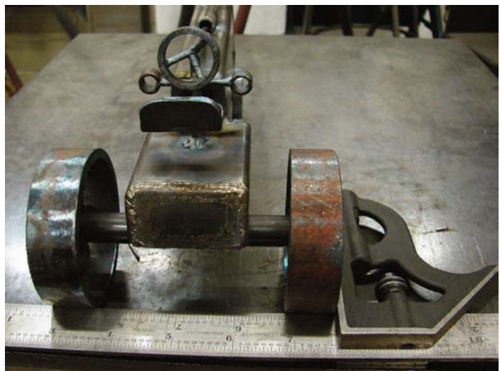
Figure 9-43. Use a square to align the tires before tacking the axles to the large tire centers.
