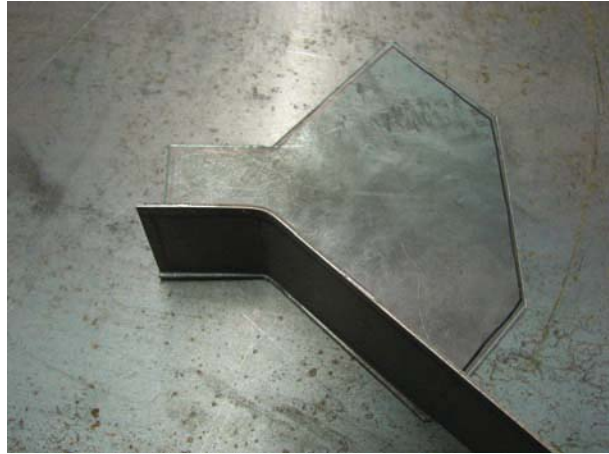
Figure 7-11. Proper angle alignment for the 45-degree corner.
