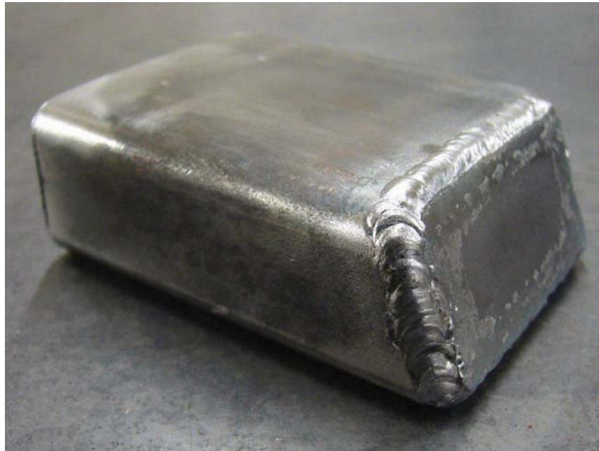
Figure 9-12. Welded seat base back cap.
