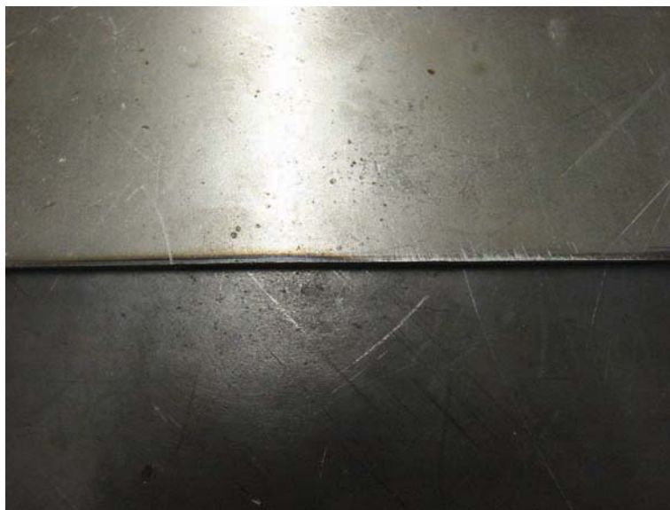
Figure 7-2. The bottom half of this image is hot-rolled steel. The mill scale gives the steel a blue-gray finish and the surface can feel slightly rough. At the top is cold-rolled steel. The finish is gray and the surface is smooth
