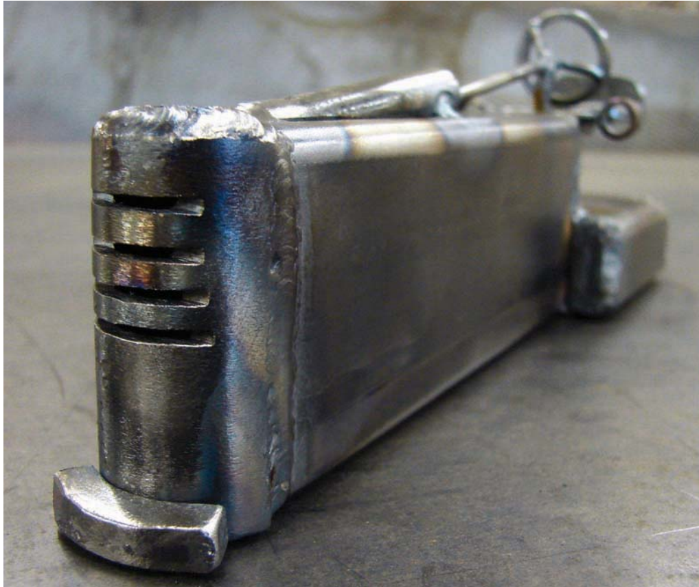
Figure 9-37. The front bumper welded in place.
