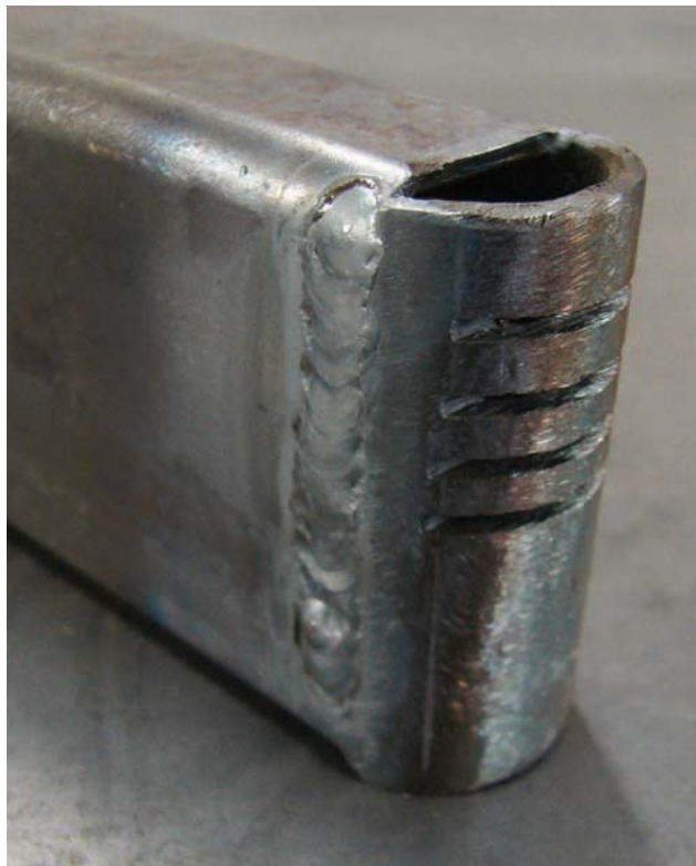
Figure 9-10. Butt weld joining the body front to the main body.
