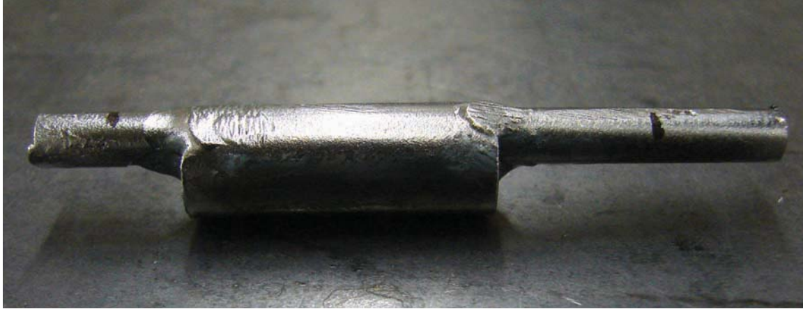
Figure 9-55. Welded smoke stack with marks made where the ends of the top and bottom sections need to be trimmed.
