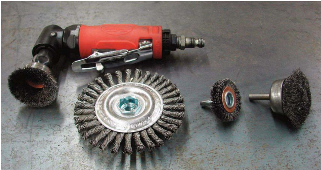
Figure 4-12. Examples of wire wheels that can be used in a die grinder and an angle grinder for finish clean up. From left to right: A cup brush attached to a die grinder, a straight knot wire wheel designed to be used in an angle grinder, a smaller die grinder straight wire wheel, and a round head wire brush.
