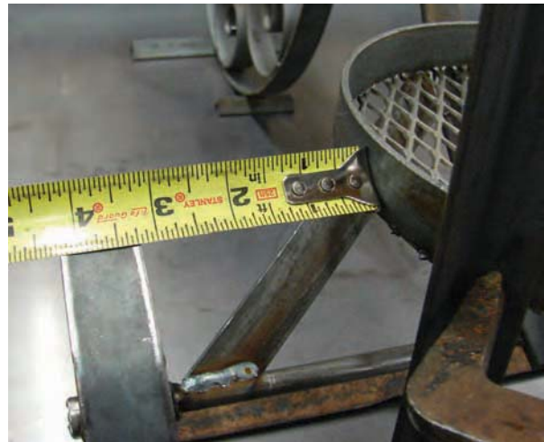
Figure 13-43. a) Positioning the lower, bottom plant holder ring. b) Centering the lower, bottom plant holder ring.
