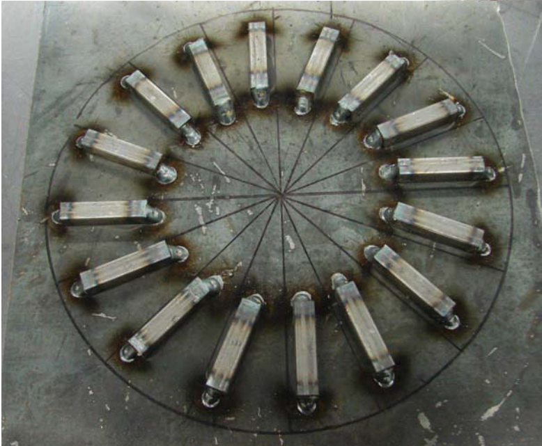
Figure 12-13. a) Attaching the stops on Jig #2. b) Completed Jig #2.
