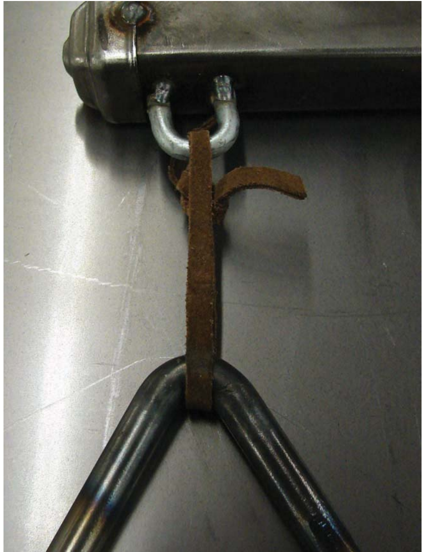
Figure 11-30. Attached chain link with a piece of leather tied from the link to hang the bell.
