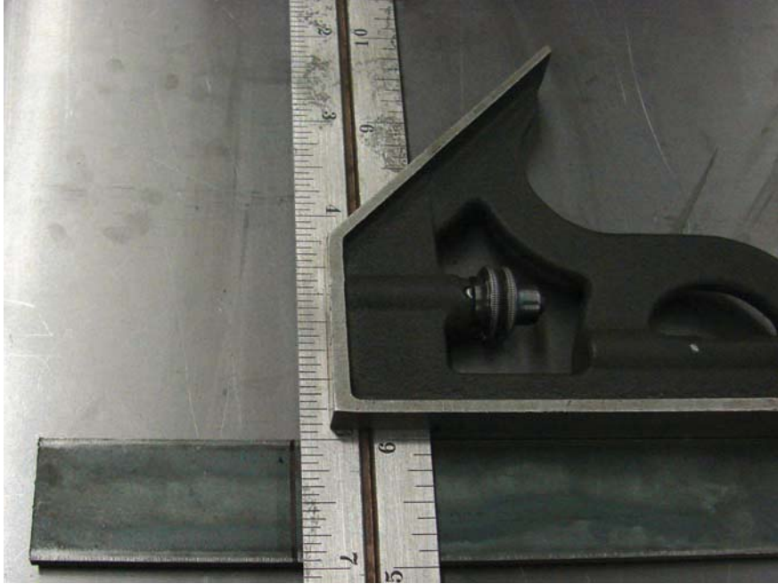
Figure 13-6. Marking the ends that will remain flat after rolling
