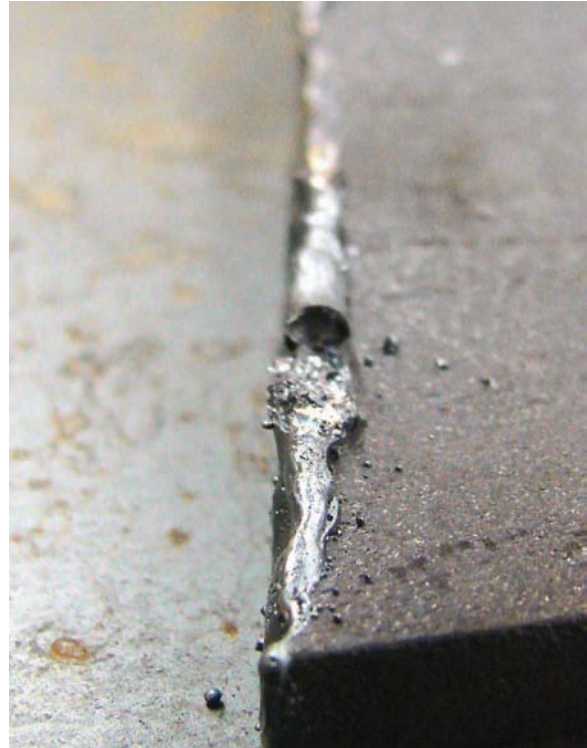
Figure 3-11. Example of slag buildup on the bottom side of a cut part.
