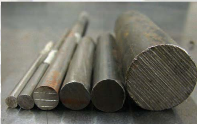
c. Round bar, also referred to as rod, is identified by its diameter. Example: 1/4" rod.
