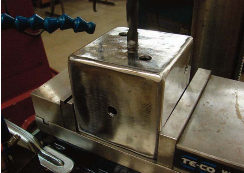
Figure 6-29. Drilling the center holes
