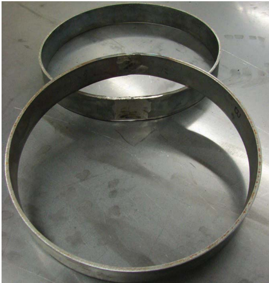
Figure 13-12. Completed small wheel rings.
