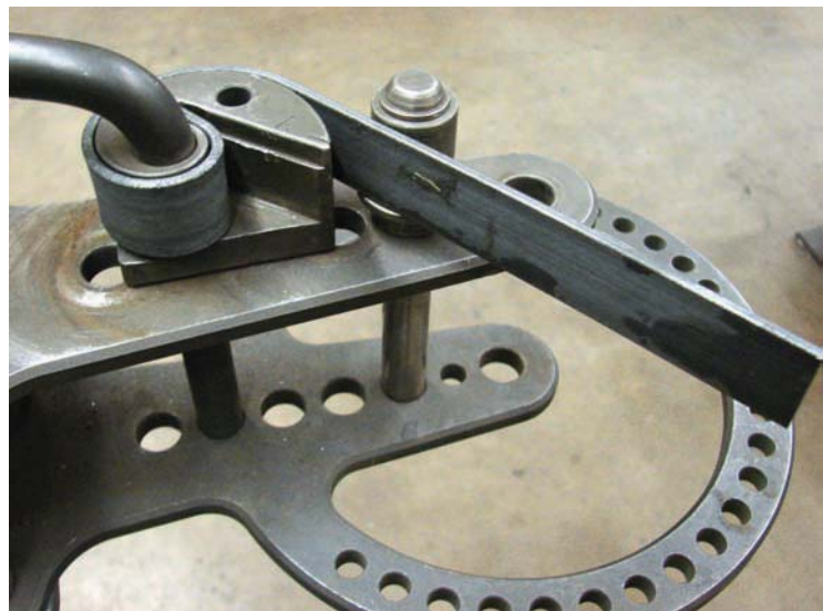
b) Turn the handle until the flat bar hits the template at the 6" mark.
