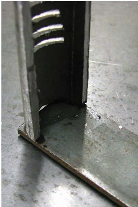
Figure 9-7. Use the body front to trace the shape needed for the body front top cap.
