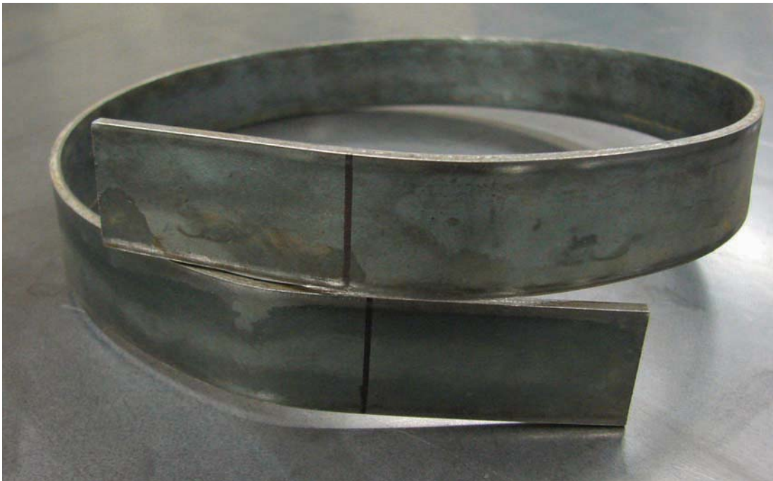
Figure 13-4. Notice the flat ends on this completed ring.
