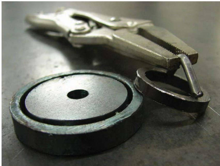
Figure 9-24. Use locking pliers to hold your part in place while welding.
