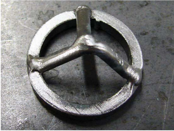
Figure 9-25. Completed steering wheel with supports.
