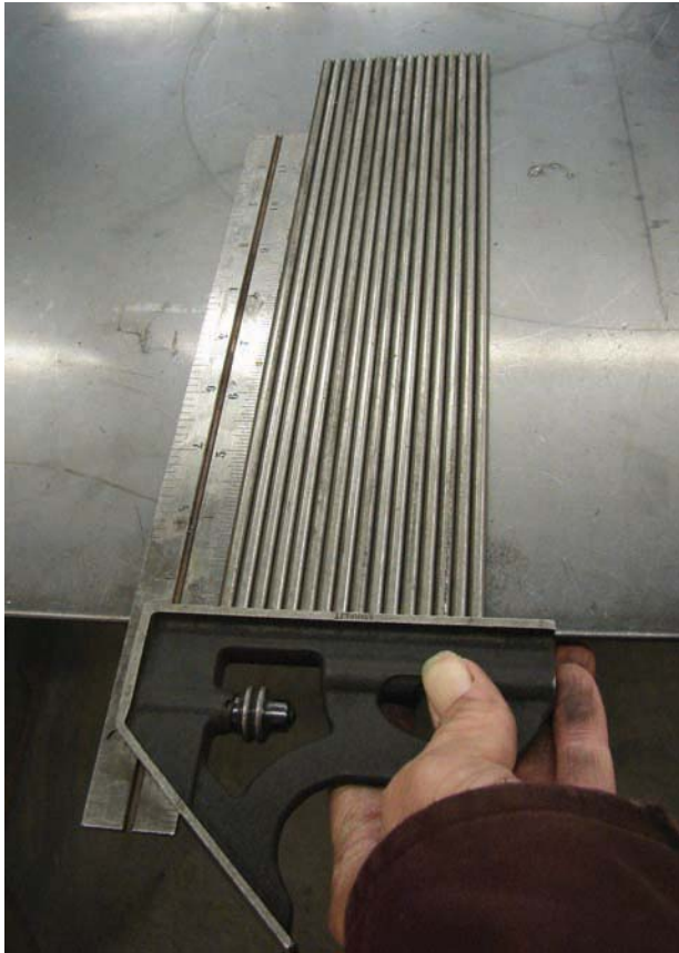
Figure 12-18. a) Sides aligned and square.
