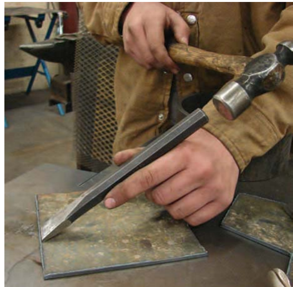
Figure 1-18. Removing dross from plasma cut steel with a chisel and hammer.
