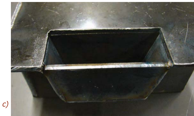
Figure 1-30. a) Hubs tacked in place. b) Hubs and sides welded solid. c) Underside of the hub free of any weld.
