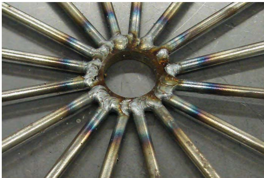
Figure 12-16. Bottom spokes welded on the bottom side.
