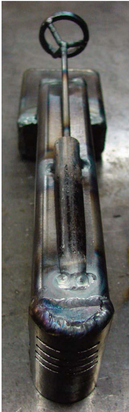
Figure 9-32. Attached steering bar cover.
