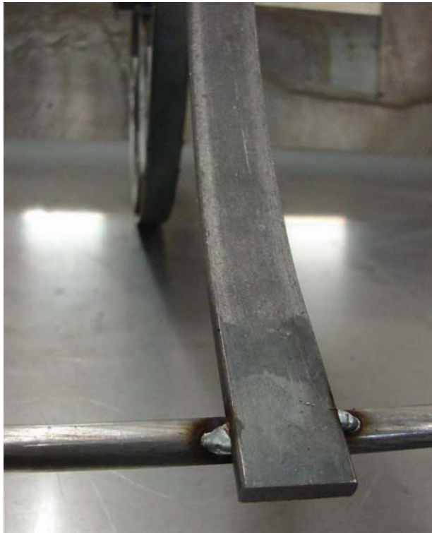
Figure 13-40. a) Tacked connector arm. b) Connector arm welded to the back axle.
