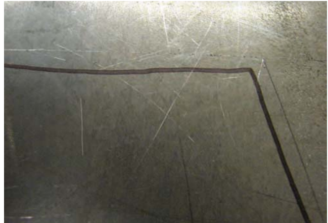
Figure 1-7. A line drawn with a marker can be helpful in locating scribed lines more easily.
