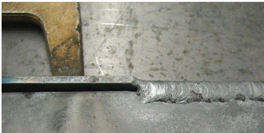
Figure 7-18. Practice outside corner joint without filler rod.
