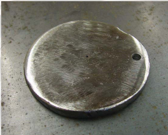
Figure 3-15. Finished bottom hole closure.
