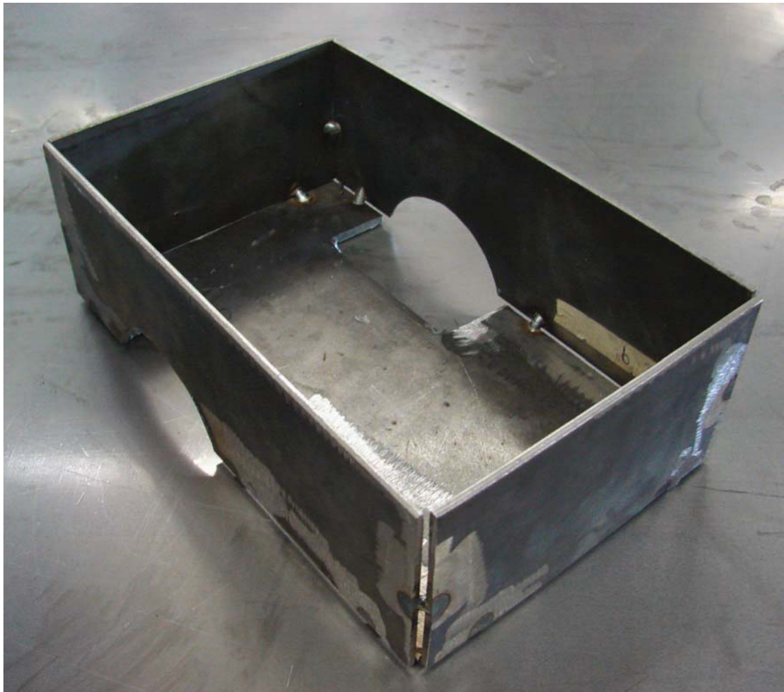
Figure 2-10. b) Wagon box tacked together.
