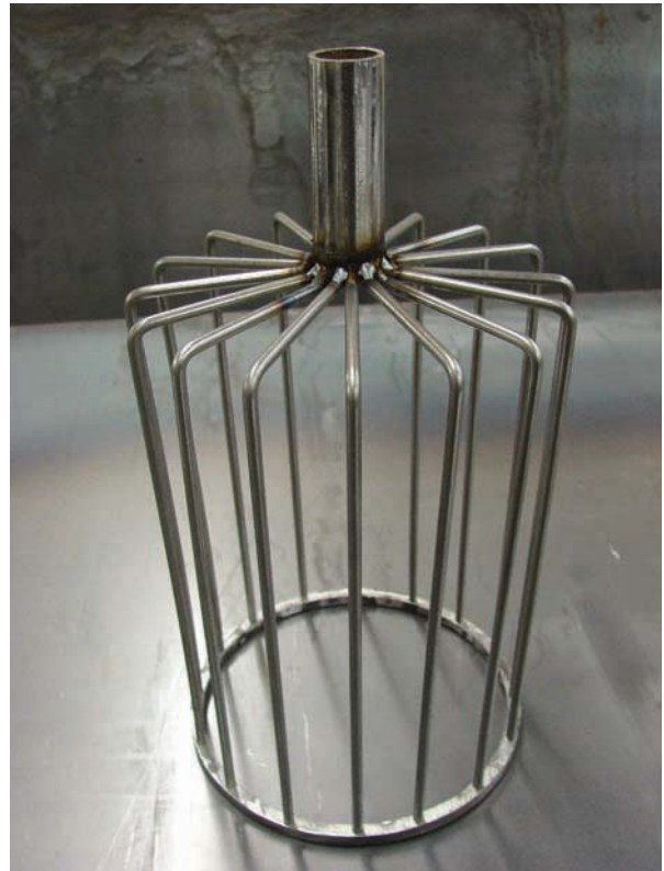
Figure 12-26. All side spokes attached to the spout.
