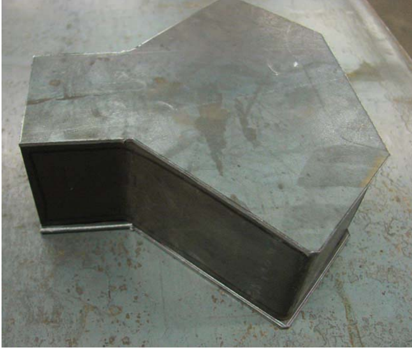
Figure 7-16. Vase sheet metal parts cut, bent, and ready for welding.
