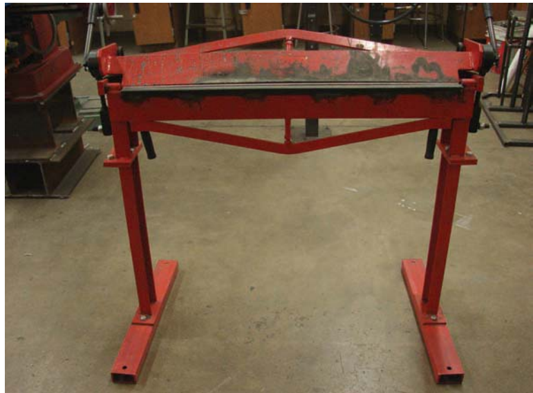
Figure 7-9. For this fairly inexpensive, light duty break, it is not recommended to bend anything thicker than 16 gauge sheet metal.
