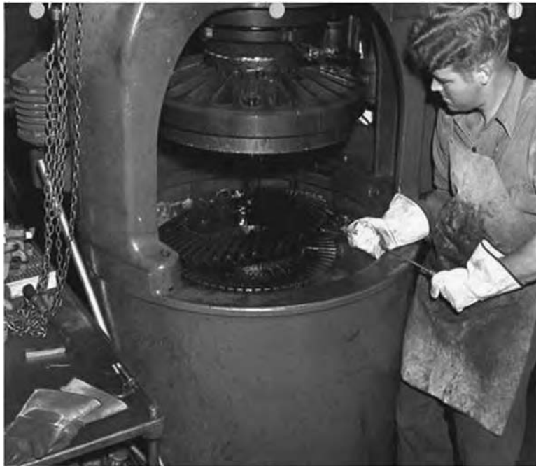
Fig. 1 One of the 64 cm (25 in.) automatic quenching machines manufactured by The Gleason Works in Rochester, NY, in the early 1930s. The operator is removing a large spiral bevel gear from the lower die assembly after the quenching operation has been completed. Courtesy of The Gleason Works, Rochester, NY
