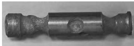
Fig. 15 Example of metal dusting in a 25 mm (1.0 in.) diameter RA 330 alloy pusher head axle pin exposed to rich carburizing atmosphere at approximately 550 °C (1020 °F) for 1 year
