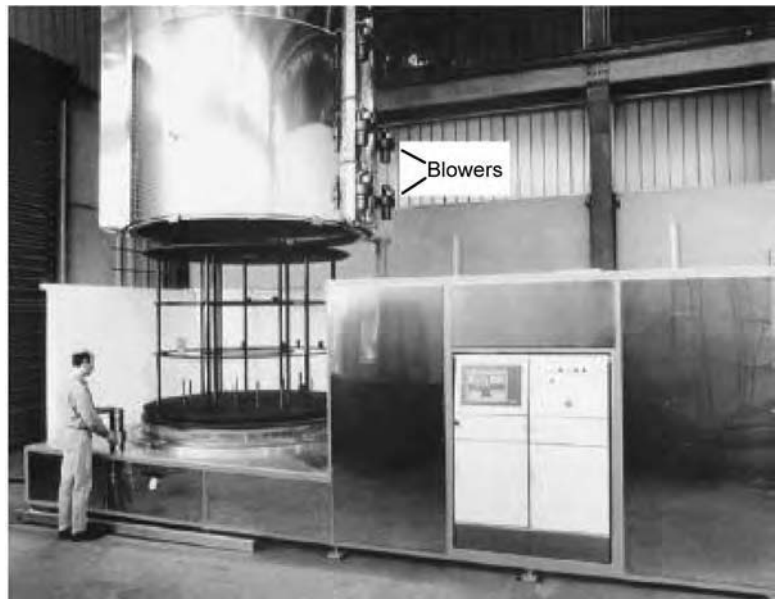
Fig. 12 Hot-walled plasma nitriding furnace. Arrows indicate air blowers that cool the external wall of the vessel. Courtesy of Plateg GmbH
