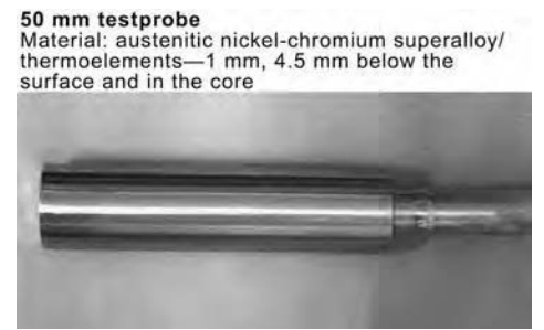
Fig. 10 Photo of the Liščić/Petrofer probe. Courtesy of Petrofer GmbH
