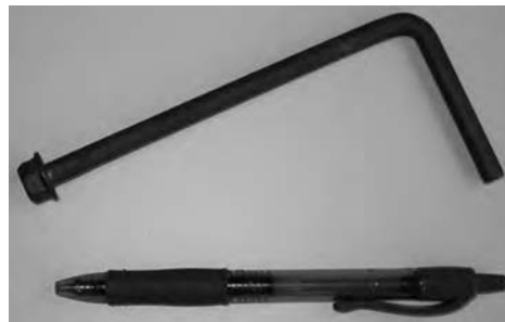
Fig. 15 A 9.5 mm ( \frac{3}{8} in.) diameter 8640 steel unthreaded bolt austempered to 44 HRC and bent 90° without cracking exhibits the superiority of a bainitic microstructure at higher (>40 HRC) hardnesses. Courtesy of Applied Process Inc.
