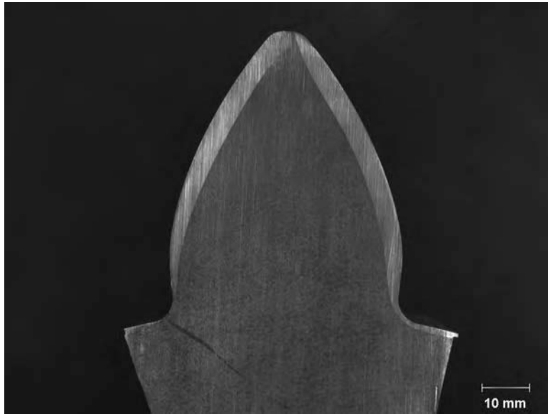
Fig. 18 Induction-hardened gear tooth polished with silicon carbide abrasive paper and etched with 10% nital. Courtesy of Materials Evaluation and Engineering, Inc.
