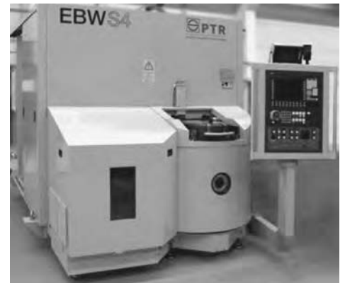
Fig. 19 Load-lock cycle facility for hardening. Chamber volume: 0.04 \text{ m}^3 ; beam parameters: 60 kV, 6 kW. Courtesy of PTR
