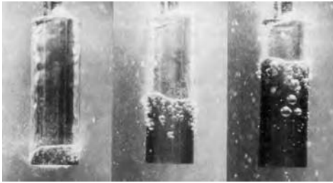
Fig. 1 Quench of a 25 mm diameter \times 100 mm (1.0 in. diameter \times 4 in.) cylinder of a CrNi steel into water at 30 °C (85 °F) with an agitation rate of 0.3 m/s (1 ft/s). Courtesy of H.M. Tensi, Technical University of Munich
