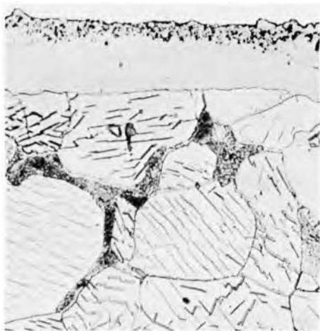
Fig. 5 Nitrided case and diffusion zone produced by cyanide-cyanate liquid nitriding. The characteristic needle structure is seen only after a 300 °C (570 °F) aging treatment. Depth of compound zone about 0.01 mm
