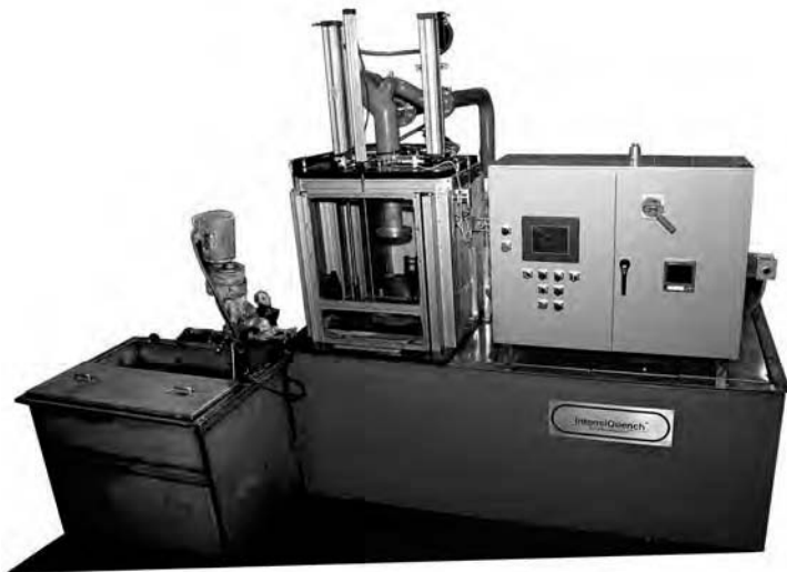
Fig. 19 Single-part production intensive quenching system for processing helicopter gears up to 200 by 480 mm (8 by 19 in.) diameter. Source: Ref 25
