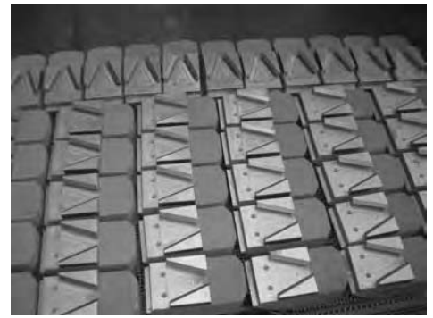
Fig. 3 Tool parts coated with stop-off paint (Condursal N633) prior to nitriding
