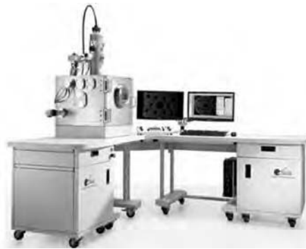
Fig. 18 Universal-chamber electron beam machine for hardening, welding, engraving, and structuring. Chamber volume: 0.5 \text{ m}^3 ; beam parameters: 60 kV, 10 kW. Courtesy of FOCUS
