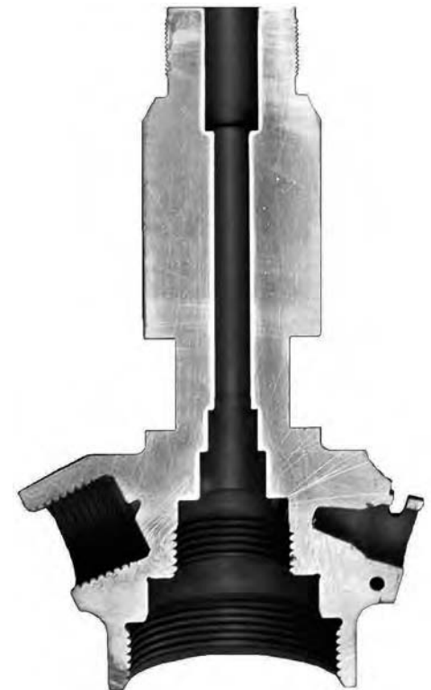
Fig. 11 Shape of investigated injector body. Source: Ref 18
