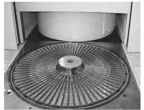
Fig. 5 Lower die assembly of a quenching machine in the "out" position. Note the spring-loaded center expander cone and the individual slotted rings. Courtesy of The Gleason Works, Rochester, NY
