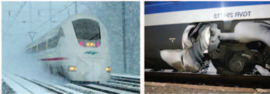
Figure 1. Snow fly and stick to the underfloor equipment.
