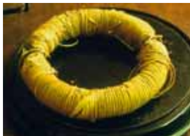
Figure 6.1 Two insulated circuits wound on an iron ring, used in Michael Faraday's investigations of electromagnetic induction.
