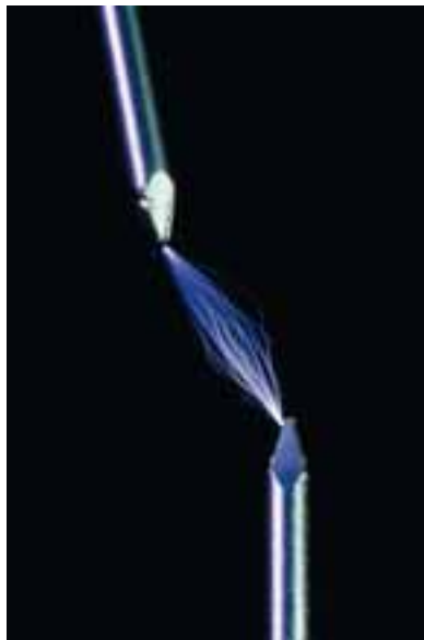
Figure 1.18 Sparks flying between two nails.
