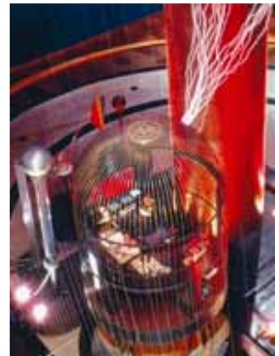
Figure 5.6 A trusting volunteer sits inside a Faraday cage, surrounded by powerful electrical discharges.
