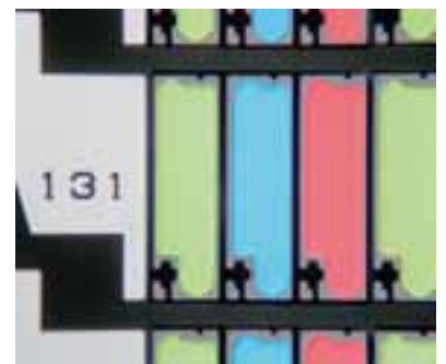
Figure 5.11 Part of the liquid crystal display of a laptop ( \times 100 ). Each triplet of green, blue and red is 1 pixel. By varying the amount of light passing through each coloured area, 16 million shades can be produced.
