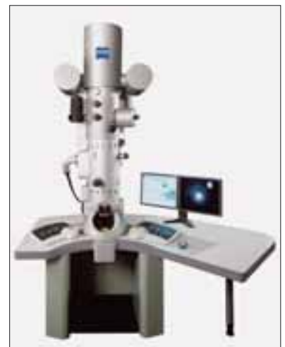
Figure 1.4 The electrons in the beam of this electron microscope travel at 70% of the speed of light.
