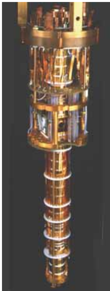
Figure 3.18 A Penning trap used to compare properties of protons and antiprotons.
