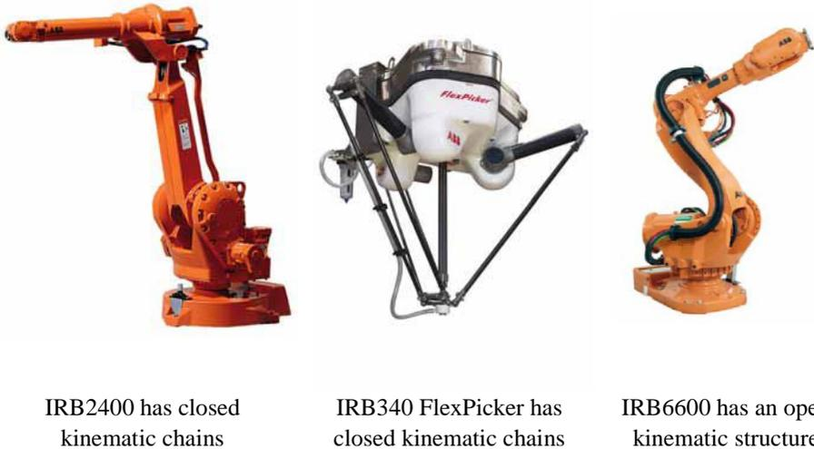
Figure 2. Robot configurations found among the ABB robots.
