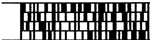
Fig. 10.7.8 Code 16K with human-readable interpretation. ( Uniform Symbology Specification Code 16K, Copyright© 1993 Automatic Identification Manufacturers, Inc. )
