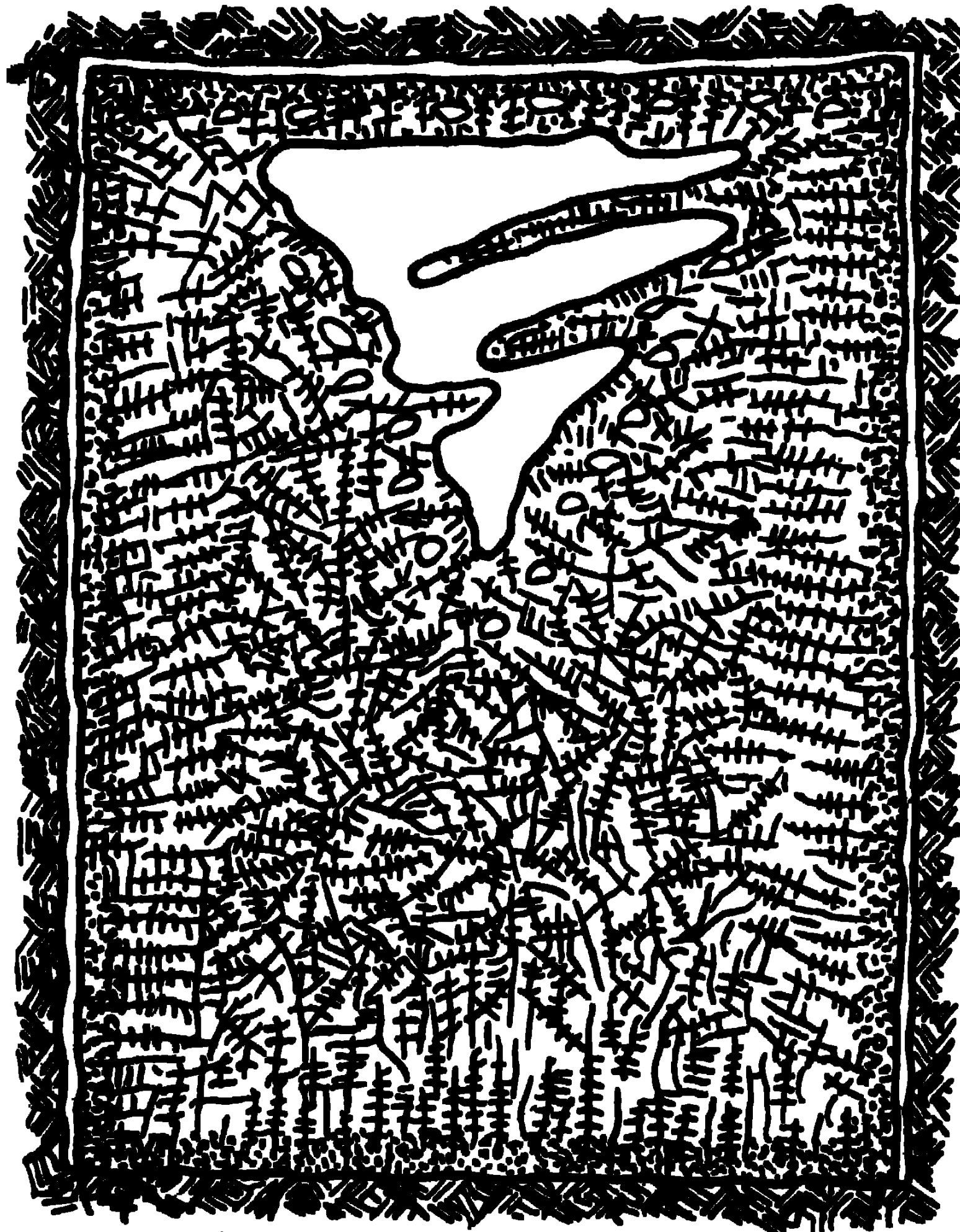
Fig. 29. Concentrated shrinkage cavity in a steel casting
