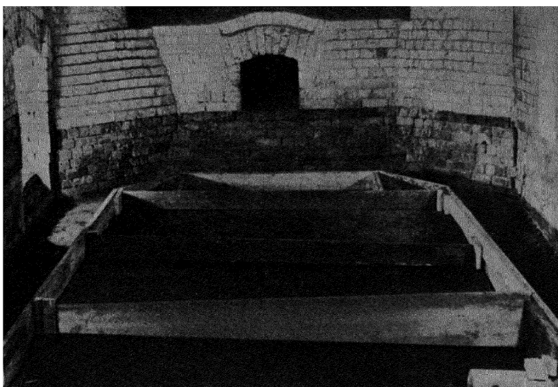
FIG. 108. Ramming a basic hearth.
