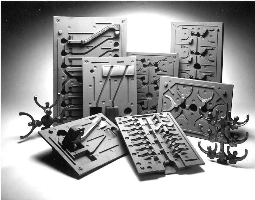
Figure 9.5 Range of shell moulds used to produce automobile castings (courtesy of Hepworth Minerals and Chemicals Ltd.) (see also References 19 and 20)
