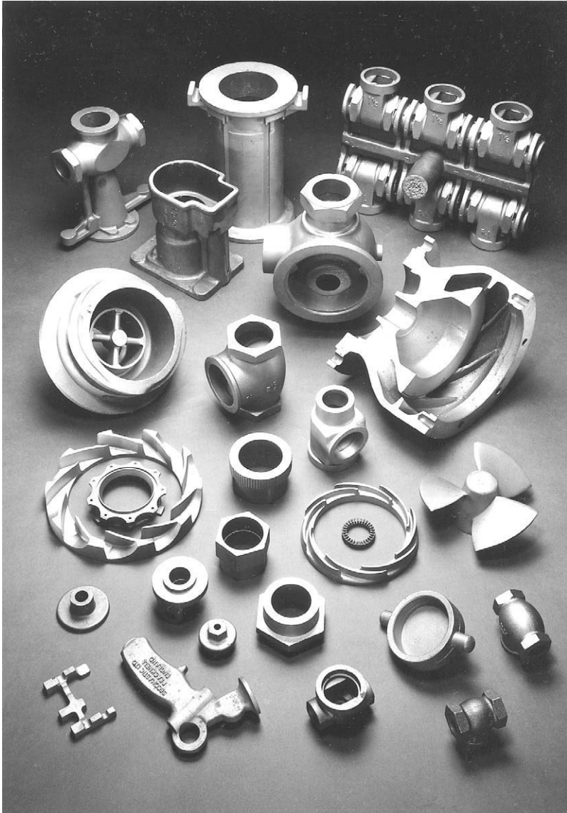
Figure 9.13 Shell moulded castings in non-ferrous alloys (courtesy of Hepworth Minerals and Chemicals Ltd.)
