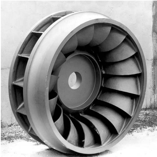
Figure 8.34 Francis runner casting for water turbine, illustrating typical application of cold setting cores to form water passages
