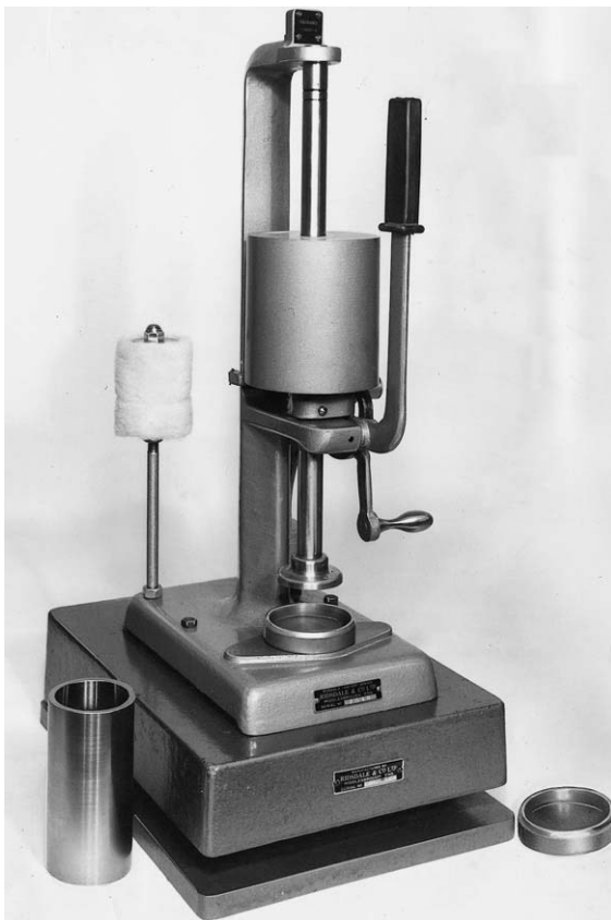
Figure 4.1 Standard rammer for specimen preparation (courtesy of Ridsdale & Co. Ltd.)
