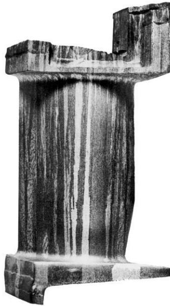
Figure 9.26 Unidirectionally solidified gas turbine blade showing columnar structure (courtesy of Pratt & Whitney Aircraft, Division of United Aircraft Corporation)
