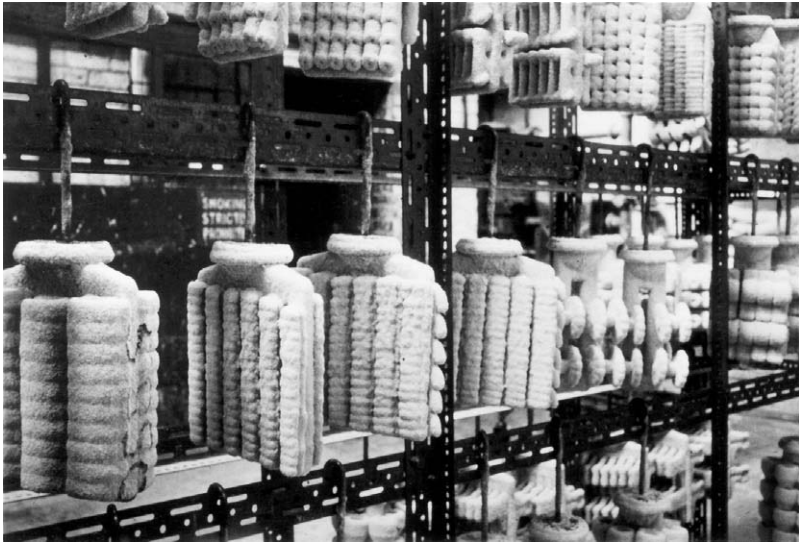
Figure 9.18 Ceramic shell moulds for investment casting (courtesy of B.S.A. Precision Castings Ltd.)
