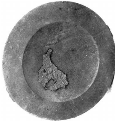
Figure 5.3 Expansion scab (courtesy of Editions Technique des Industries de la Fonderie)
