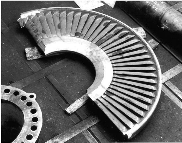
Figure 7.19 Turbine half ring with cast-in wrought blade sections (courtesy of Reyrolle-Parsons & Co. Ltd.)
