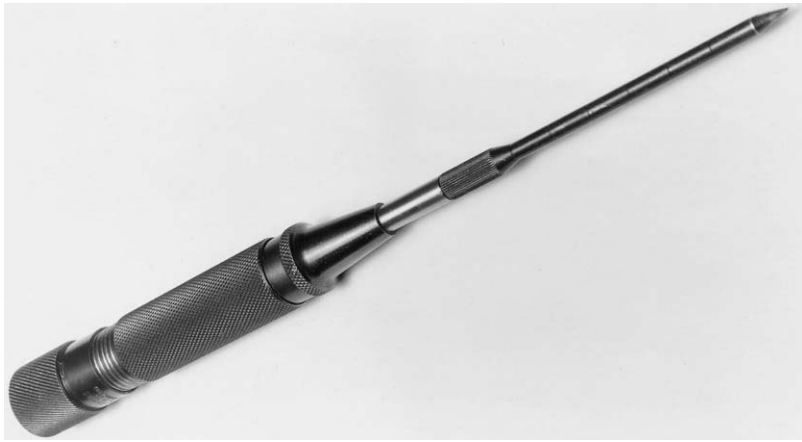
Figure 4.8 Impact penetration tester with internal spring loaded hammer (courtesy of Ridsdale & Co. Ltd.)
