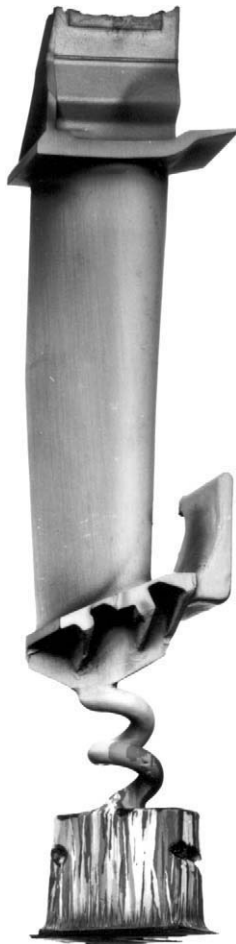
Figure 9.27 Example of cast metal geometry used for production of a single crystal turbine blade casting, embodying a spiral mould constriction (courtesy of Rolls Royce plc)
