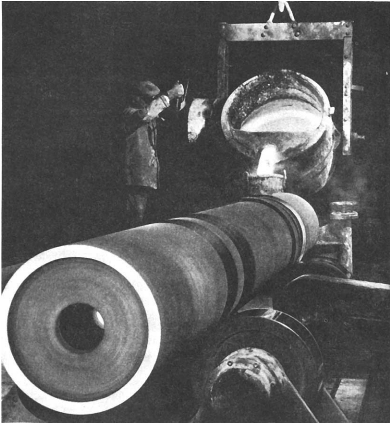
Figure 10.6 Free roller centrifugal casting machine (courtesy of Sheepbridge Alloy Castings Ltd.)
