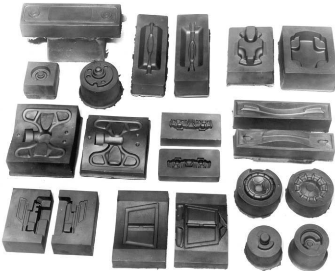
Figure 9.33 Cast dies manufactured by the Shaw process, for forming and die casting (courtesy of Avnet-Shaw & Co. Ltd.)
