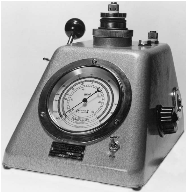
Figure 4.6 Compact direct reading permeability meter (Ridsdale–Dietert electric Permmeter, courtesy of Ridsdale & Co. Ltd.)
