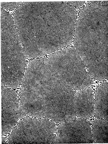
Figure 2.15 Cellular structures in impure eutectic grains. (a) Transparent organic system: camphor–succinonitrile. \times 410 (from Hunt and Jackson 25 ) (courtesy of Metallurgical Society of A.I.M.E.), (b) Al–Zn alloy. \times 130 approx. (from Kraft 27 ) (courtesy of Metallurgical Society of A.I.M.E., Journal of Metals)
