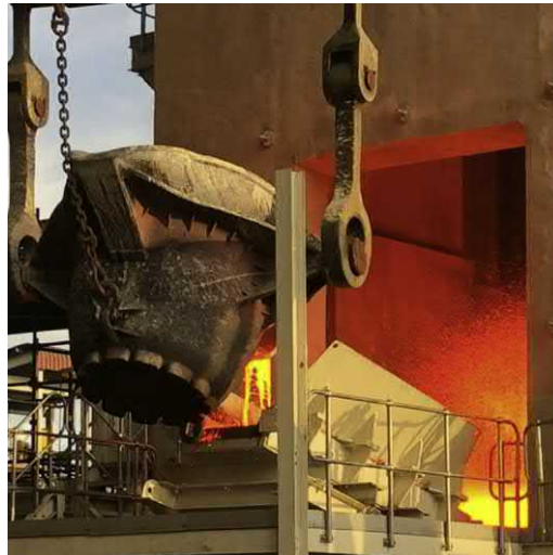
FIGURE 58.11 The air granulation process. Source: Courtesy of Hatch Ltd. (Faucher S, et al. Recent developments in commercial dry slag granulation and energy recovery. In: AISTECH 2016, association of iron and steel technology proceedings, May 2016, Pittsburgh; 2016. p. 137–44). 16
