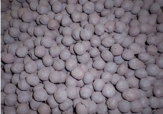
FIGURE 4.2 Hematite (Fe 2 O 3 ) iron ore pellets ready for charging to an iron blast furnace. They are approximately 8–16 mm diameter. Source: Photo courtesy: Midrex Technologies Inc.
