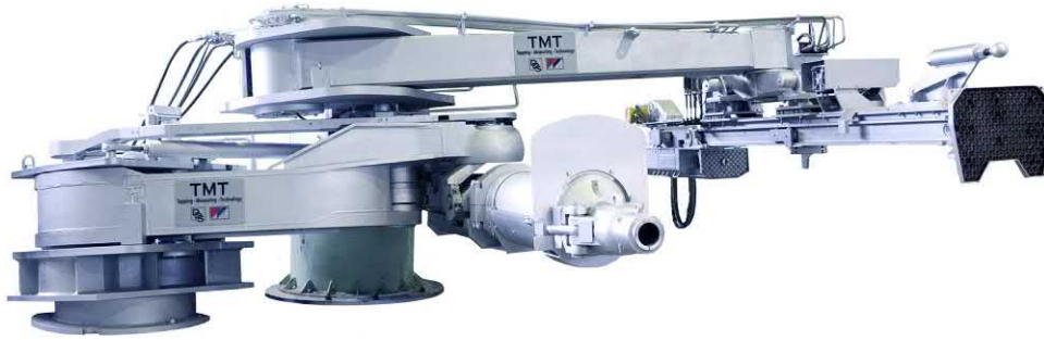
FIGURE 57.10 Arrangement of mud gun and taphole drill when located on the same side of the iron trough. Source: Courtesy of TMT—Tapping Measuring Technology S.à. r.l & G.m.b.H.
