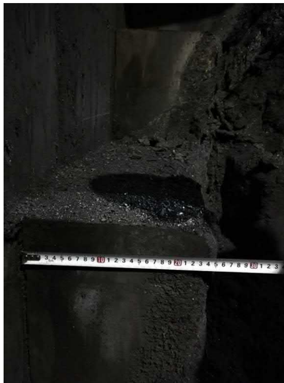
FIGURE. 53.3 Direct measurements of the brick thickness at the sidewall of an off-line blast furnace. Source: Photo courtesy: Dr. Afshin Sadri, Hatch Ltd.
