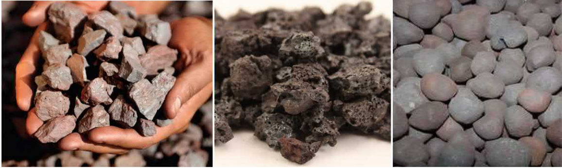
FIGURE 54.1 Blast furnace ferrous charge materials: lump ore (left), sinter (center), and pellets (right). Source: Photo courtesy: Manuel Huerta, Hatch Ltd.
