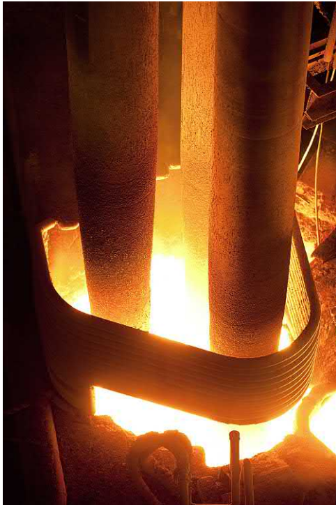
FIGURE 3.7 Ladle metallurgy furnace reheating liquid steel in preparation for continuous casting. Graphite electrodes heat the steel from the top, while the liquid steel is argon stirred from the bottom. Alloys are added by gravity through drop chutes and using solid metal and powder filled wires added at high speed. Source: Photograph courtesy of SMS Group.
