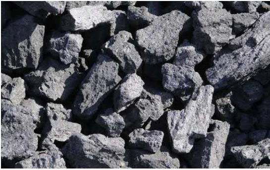
FIGURE 55.1 Metallurgical coke produced using SunCoke Energy's heat recovery coking process. Source: Photograph courtesy of SunCoke Energy Inc.
