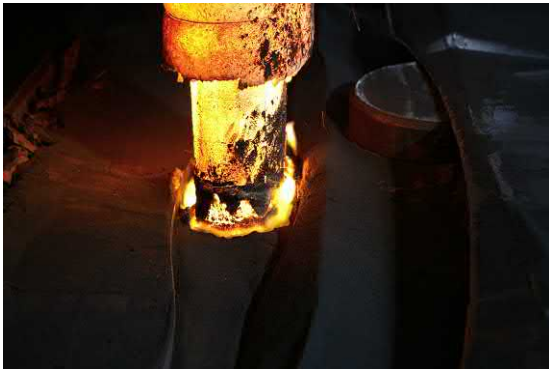
FIGURE 3.9 Steel being cast via a submerged nozzle located into a thin slab caster copper mold. The molds are made of high purity copper—due to its very high thermal conductivity. Cooling and solidification is obtained by rapid extraction of heat from the molten steel through copper and into sprays of cooling water. Source: Photograph courtesy of SMS Group.
