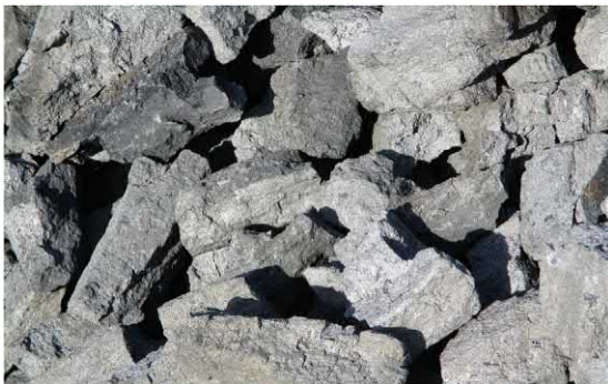
FIGURE 1.4 Metallurgical coke, about 70–100 mm long. Coke is made by high-temperature vaporization of volatiles, (e.g., \text{CH}_4 ) from coal heated in the absence of air, Chapter 55, Metallurgical Coke—A Key to Blast Furnace Operations. “Met” coke contains 87–91% carbon and 9–13% oxide ash; mostly silica and alumina from the original coal. The coke burns with blast air near the bottom of the blast furnace and in front of the tuyeres to (1) provide heat for the ironmaking process, and (2) carbon monoxide for iron oxide reduction. Source: Photograph courtesy of SunCoke Energy Inc.
