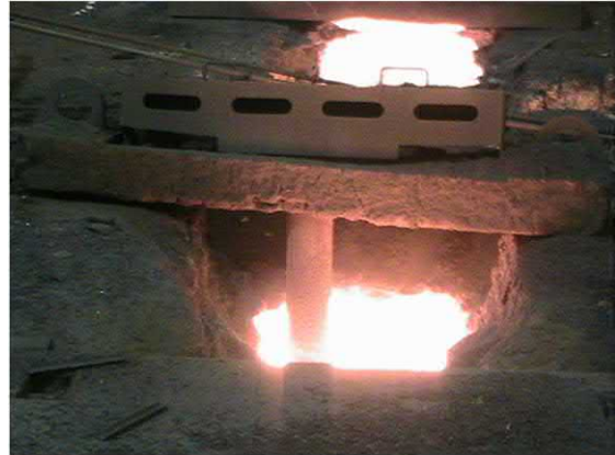
FIGURE 1.10 Pt–Rh thermocouple in flowing-tapped molten iron stream. It is inside the vertical refractory probe (bottom end closed) to give a continuous measure of hot metal temperature. Source: Photo courtesy of Algoma Inc.
