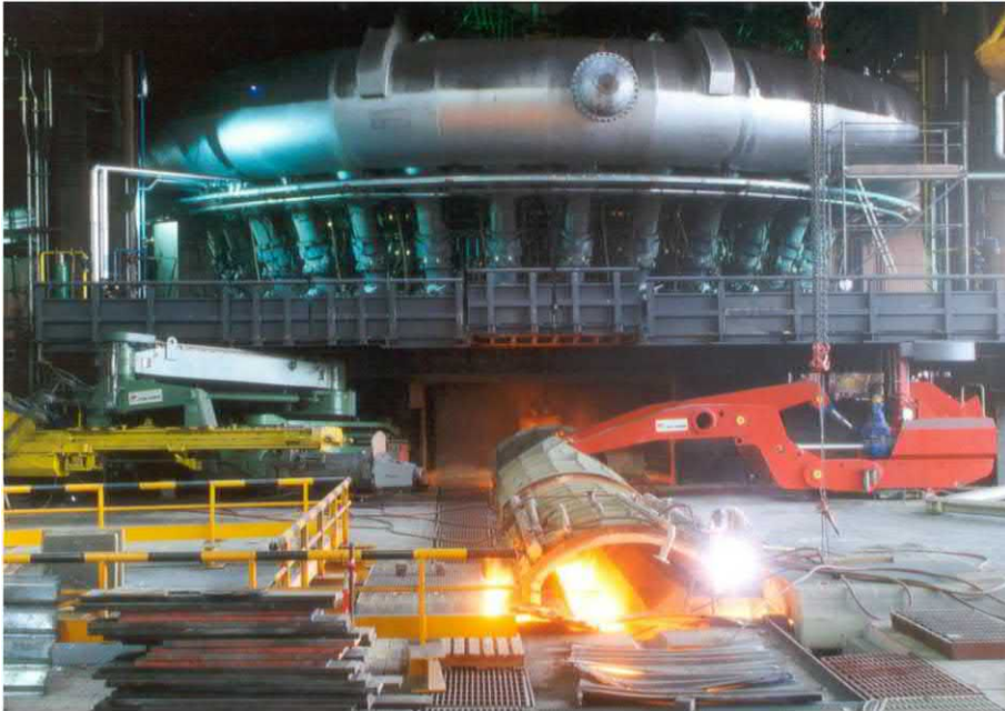
FIGURE 1.9 Molten iron and slag being tapped from a blast furnace. They are separated in the main trough by allowing dense molten iron ( 6.8 \text{ t/m}^3 ) to flow under a refractory skimming block while forcing the less dense molten slag ( 2.7 \text{ t/m}^3 ) to collect above the iron and flow into a slag runner. The molten iron flows continuously into a torpedo-shaped rail car ladle used to transport the hot metal to steelmaking. The molten slag flows to a granulation machine or is solidified in pits-then sold. Notice the huge bustle pipe that distributes blast air to individual tuyeres. Source: Photograph courtesy of TMT—Tapping Measuring Technology S.à. r.l & G.m.b.H.
