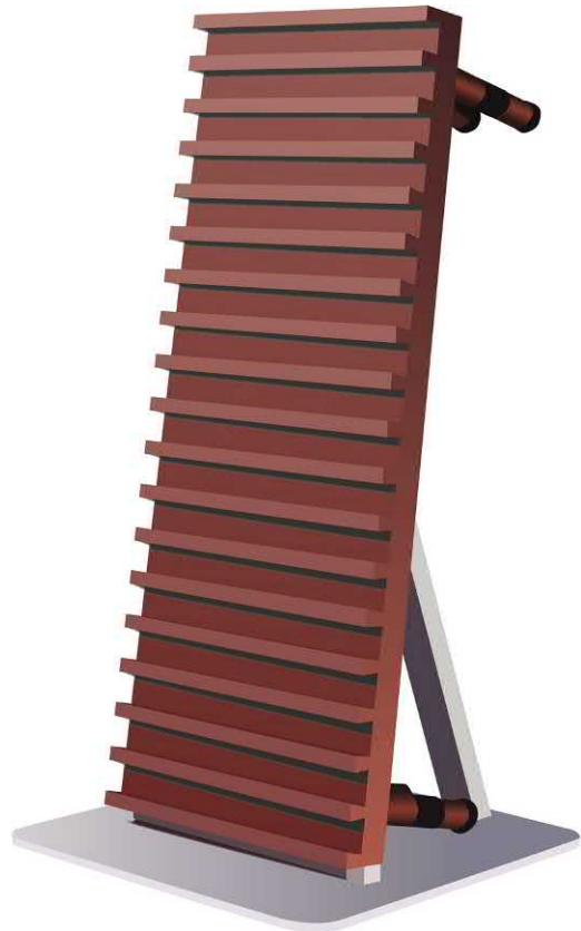
FIGURE 5.2 Water-cooled blast furnace cooling element - called a stove. These staves are attached to the inside of the blast furnace walls. Cooling staves can be made from copper or cast iron. Their job is to maintain the structural integrity of the furnace by cooling the walls. Cool water is pumped into, around, and out of a hollow flow pattern or pipe inside the stove - removing heat from the furnace wall. In service, the grooved interior face (left) is packed with refractory bricks. Many other water cooling shapes are used as needed. 6
