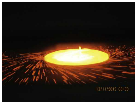
FIGURE 58.12 Spinning ceramic cup air granulation process developed by Primetals. Source: Courtesy of Primetals Technologies Austria GmbH (Fenzl T, et al. Installation of a dry slag granulation pilot plant at blast furnace A of voestalpine. Vienna: European Steel and Technology Application Days (ESTAD); 2017. p. 1763–72.).
