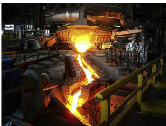
FIGURE 4.4 Molten iron 1500°C flowing out of an iron blast furnace. Excluding other impurities, for example, Si, it contains ~95.5 mass% Fe and 4.5 mass% C. In practice, molten iron and molten slag are tapped together. Source: Photograph courtesy: TMT—Tapping Measuring Technology S.à. r.l & G.m.b.H.
