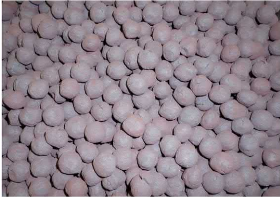
FIGURE 1.3 Fired hematite ( \text{Fe}_2\text{O}_3 ) pellets ready for charging to an iron blast furnace. They are 8–16 mm in diameter and contain ~64 mass% Fe as compared to 70 mass% Fe in pure \text{Fe}_2\text{O}_3 . Source: Photograph courtesy of Midrex Technologies Inc.
