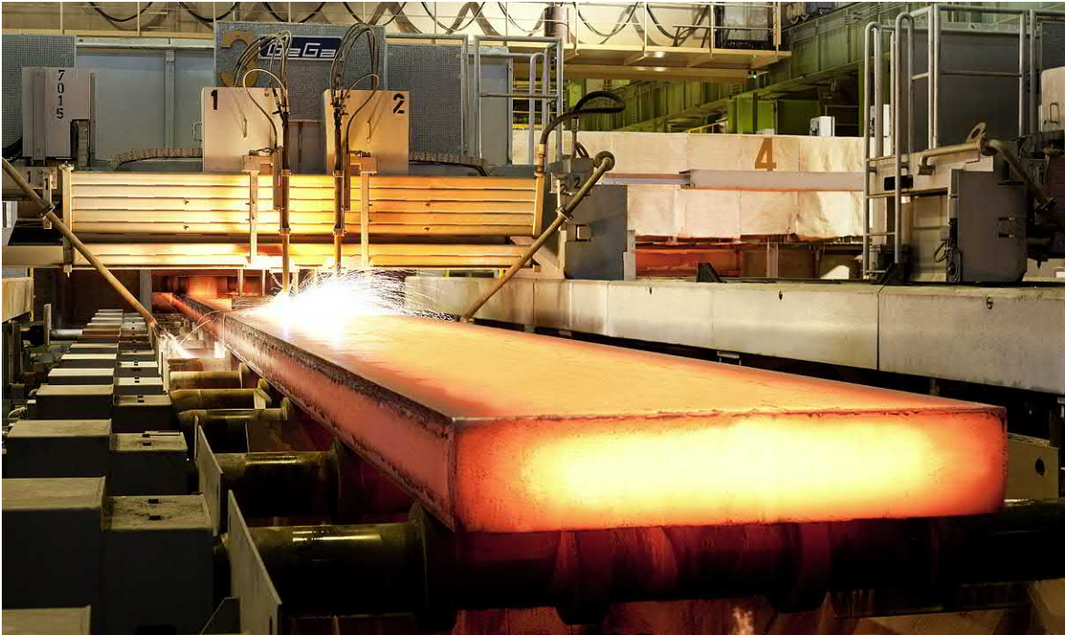
FIGURE 3.11 A continuously cast solid steel slab being cut for hot rolling and subsequent manufacturing processes. The slabs are about 2 m wide and 0.8 m thick. They are being cut into 10 m lengths for rolling by flying gas torches that clamp onto and move forward at the same speed as the steel, \sim 1\text{--}2 m/min. Source: Photograph courtesy of SMS Group.
