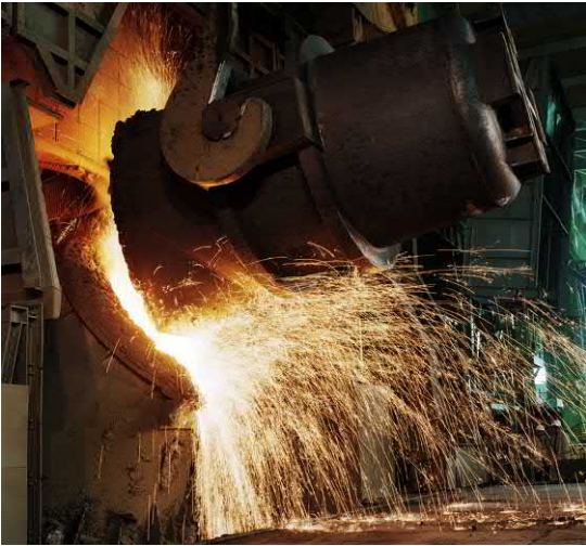
FIGURE 3.4 Charging hot metal to a BOF converter. About 80–90% of the ferrous charge to make a heat of steel is hot metal produced by adjacent blast furnaces. The balance is scrap used as a coolant to mitigate the exothermic oxidation of silicon and carbon in the hot metal. Iron ore pellets can also be used as a coolant. BOF, Basic oxygen furnace. Source: Photograph courtesy of SMS Group.
