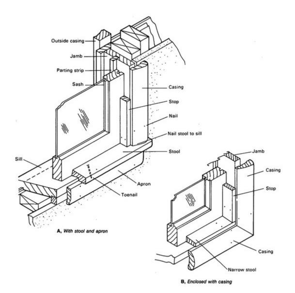
The casing is applied and nailed as described for door frames except that the inner edge is flush with the inner face of the jambs so that the stop covers the joint between the jamb and casing. The apron is cut to a length equal to the outer width of the casing line. It is nailed to the window sill and to the 2- by 4inch framing sill below.
