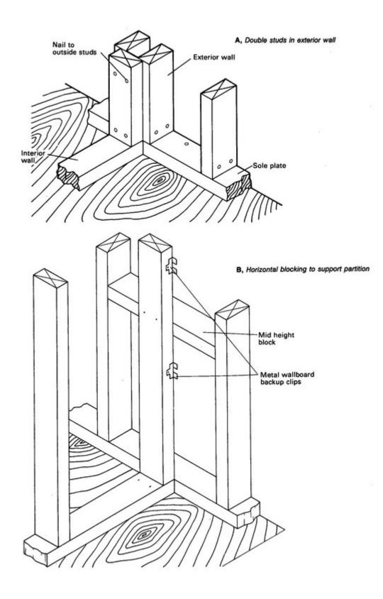
Figure framing for platform construction.
