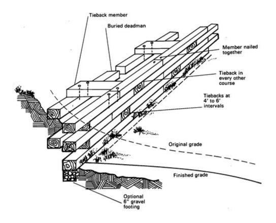
**<u>Figure</u>** timber and rough-sawn dimension lumber retaining
