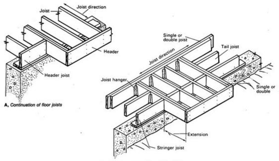
B, Projection perpendicular to floor joists
