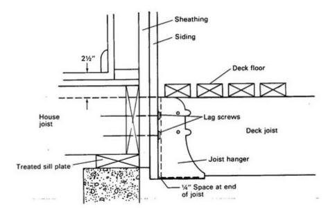
Figure attachment to house with header joist.
