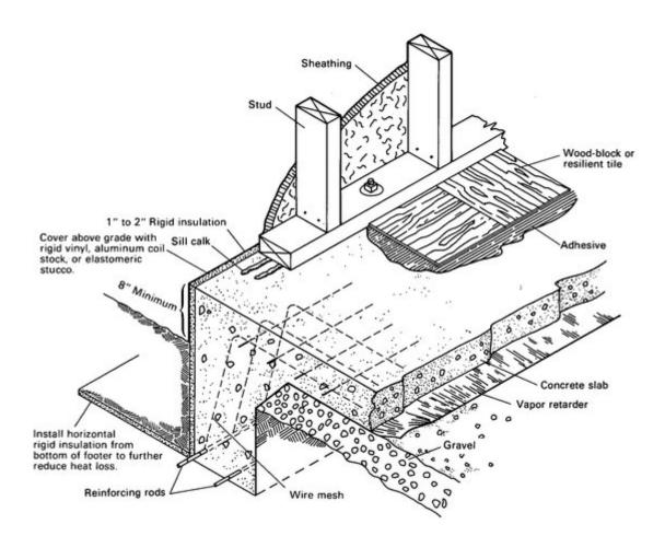
**Figure** grade beam for concrete slab giving moderate resistance to frost heave when piers are used.
