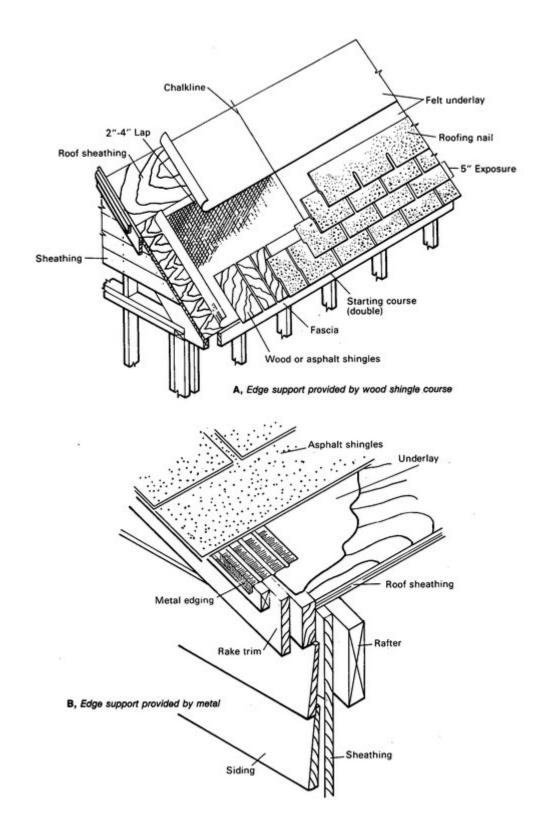
Metal edging is often used around the entire perimeter of the roof. A starter course is used under the first shingle course. This starter course should extend downward about ½ inch beyond the
