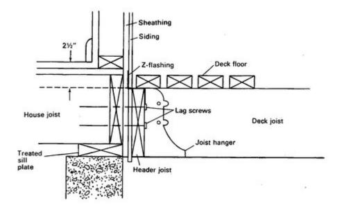
**<u>Figure</u>** attachment to house using ledger.
