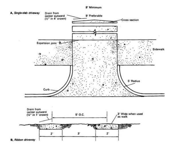
The concrete strips in a ribbon driveway should be at least 2 feet in width and located so that they are 5 feet on center (fig. 148B). When the ribbon is also used as a walk, the width of strips should be increased to at least 3 feet.
