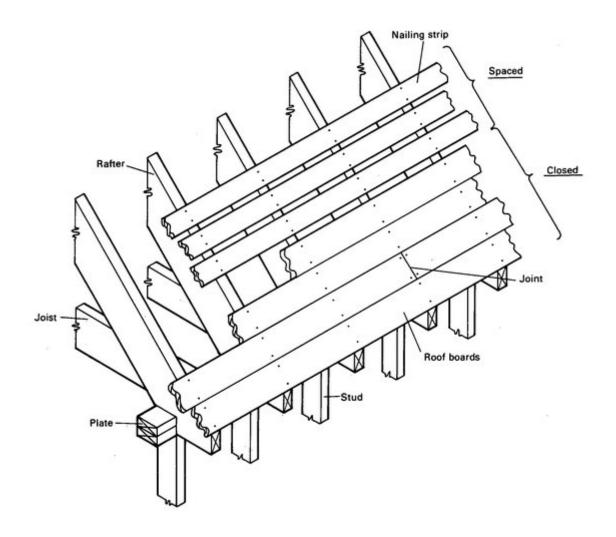
**<u>Figure</u>** roof decking common in post and beam construction.
