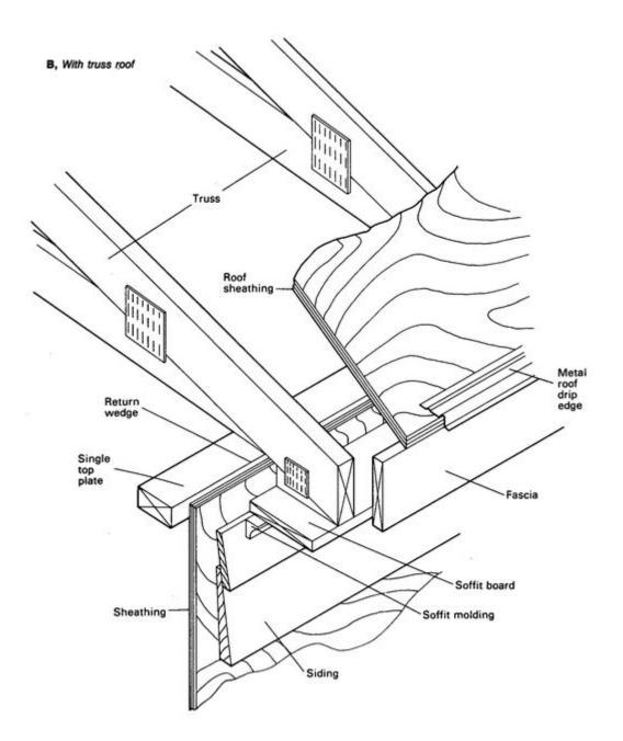
**Box cornice without returns.** A wide boxed cornice without horizontal returns or lookouts, providing a sloped soffit, is sometimes used for houses with wide overhangs (figs. 119A and 119B). The soffit material is nailed directly to the underside of the rafter extensions. Inlet ventilators, singly or in a continuous strip, are installed in the soffit area.
