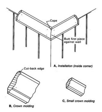
A cutback edge at the outside of the molding partially conceals any unevenness of the finish and makes painting easier where there are color changes Finish nails should be driven and set into the upper wall plates and, for large moldings, also into the ceiling joists, when possible.
