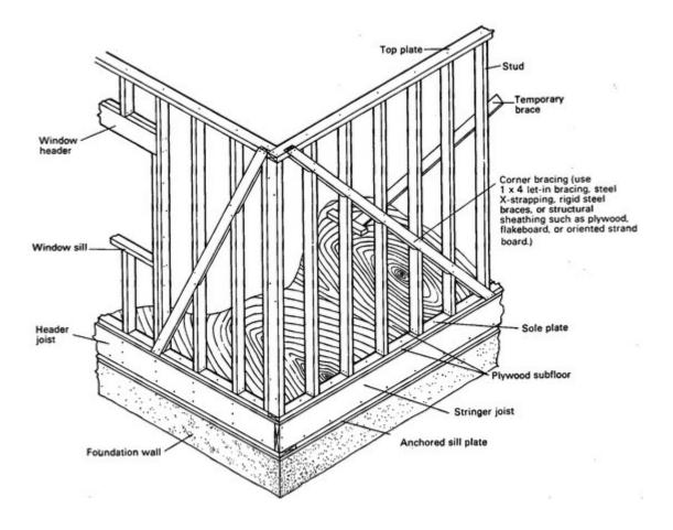
**<u>Figure</u>** alignment of framing members simplifies framing and transmits loads directly down through structural members.
