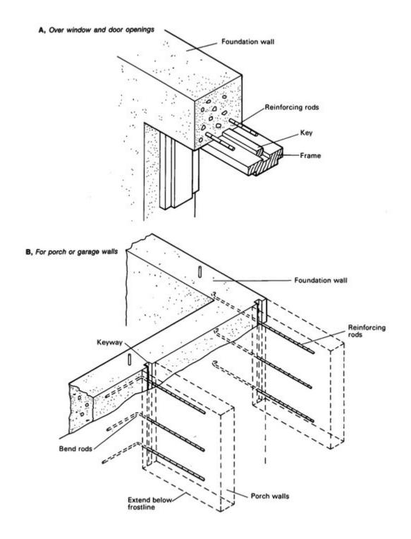
Poured or precast concrete foundation walls.
