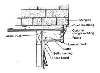
**<u>Figure</u>** rake extension with fly rafter:
