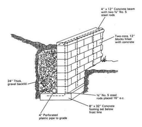
**<u>Figure</u>** Reinforced concrete retaining wall (4 feet high above grade).
