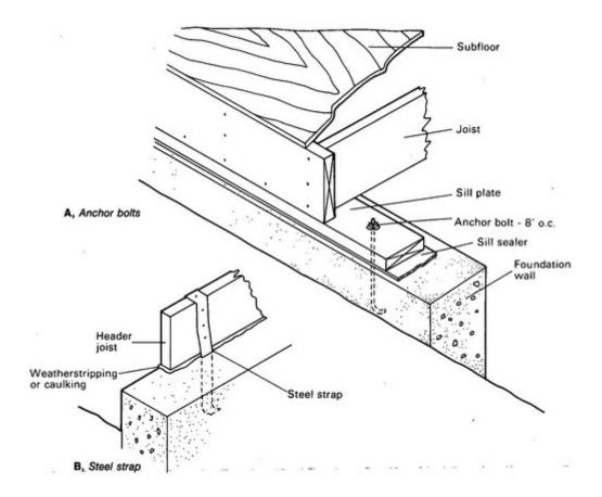
A sill sealer is often used under the sill plate on cast-in-place walls to fill any irregularities between the plate and the wall. Anchor bolts should be embedded 8 inches or more in poured concrete walls and 16 inches or more in block walls with concrete-filled cores. The bent end of the anchor bolt should be hooked under a block and the core filled with concrete. If termite shields are used, they should be installed under the plate and sill sealer.
