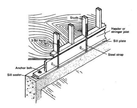
Figure\_wall framing to floor framing.
