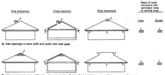
B, Inlet openings in eave soffit and outlet vent at ridge. Ratios of total minimum net ventilator area to ceiling area may be specified in local building codes
