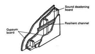
**Figure** wall on separate plates has an STC rating of 42 to 44. If insulation is added to the stud cavities on one side, the STC rating is increased to 50 to 53.
