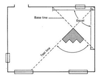
**Building the pattern.** Use a cold, cut-back asphalt mastic spread at the minimum rate of 50 square feet per gallon. Use the notched edge of the trowel. Allow to harden a minimum of 2 hours or up to 48 hours as directed by the manufacturer. The surface will be solid enough after 12 hours to allow you to snap working chalk lines on it. Use blocks of the flooring as stepping stones on the mastic to snap lines and begin the installation.
