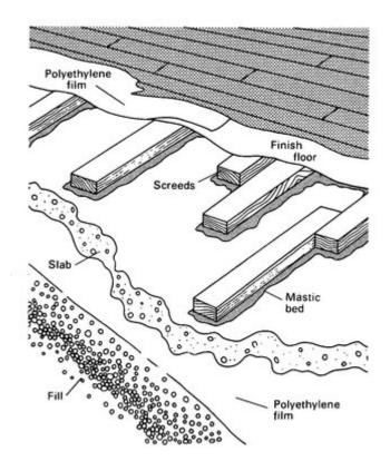
Over the screeds spread a vapor retarder of 4- or 6-mil polyethylene film with edges lapped 6 inches or more. It is not necessary to seal the edges or to affix the film with mastic but avoid bunching or puncturing it, especially between screeds. The flooring finish is nailed through the film to the screeds.
