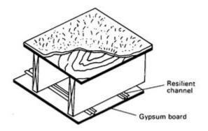
**<u>Figure</u>** floor-ceiling structure having carpet, pad, plywood subfloor, and ceiling gypsum board supported on separate ceiling joists has an STC
