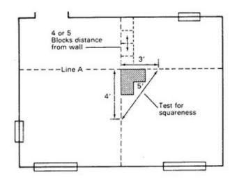
*Herringbone pattern.* Most existing parquet patterns can be laid out with these two working lines. Herringbone, however, requires two test lines: one is at the 90 ° line already described; the other crosses the intersection of the first two lines, but at a 45° angle to both.
