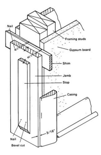
**<u>Figure</u>** closet door mounted directly on finished wall with hinges secured to wall framing.
