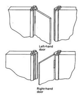
The frame is set in place and jambs are nailed to the rough framing. Where there is a gap between jambs and rough framing, place shims in the gap before nailing. Use two 8d finishing nails about 16 inches apart over the length of the jambs Folding closet doors can be installed by mounting hinges on the gypsum board at the opening with screws secured into the framing behind the gypsum board
