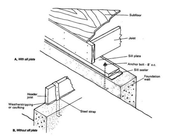
**Figure** floor system to concrete block foundation wall:
