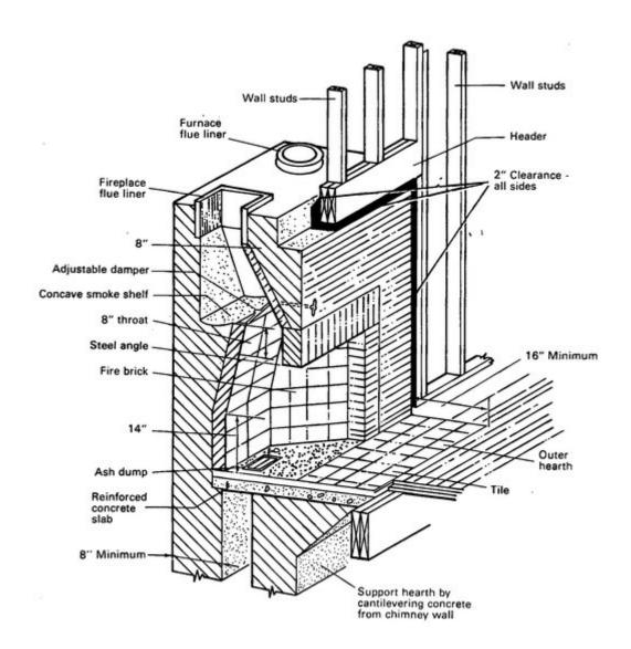
The firebox form is set on a firebrick floor laid on reinforced concrete. The chimney flue is begun at the top of the form, and, facing the room, decorative masonry is laid around the unit opening. Small fans are often installed to increase the heating efficiency of the unit, and the inlets and outlets are covered with decorative grates.
