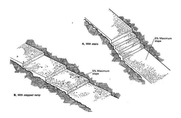
For a moderately uniform slope, a stepped ramp may be satisfactory (fig. 149B). Generally, the rise should be about 6 inches to 61/2 inches and the length between risers sufficient for two or three normal paces.
