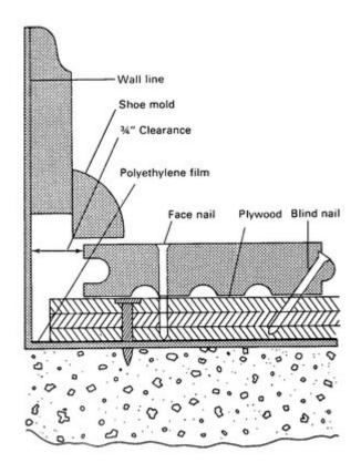
Fasten the plywood to the concrete with a power-actuated concrete nailer or hammer-driven concrete nails. Use a minimum of nine nails per panel, starting at the center of the panel and working toward the edges to be sure of flattening out the plywood and holding it securely. An alternative method is to cut the plywood into 4- by 4-foot squares, score the back, and lay in mastic. However this requires the use of moisture retarders laid in mastic.
