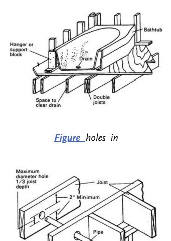
*Figure* joists to allow installation of ductwork in load-bearing partitions.
