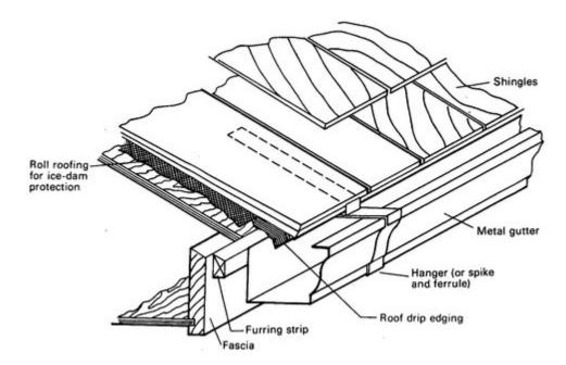
The roof framing at the wall line should not block ventilation to the attic area. Blockage can be avoided by use of a "ladder" frame extension (see fig.
