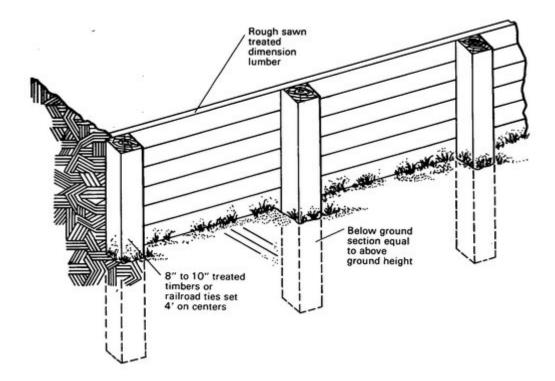
**<u>Figure</u>** Pressure-treated post and plywood retaining wall.
