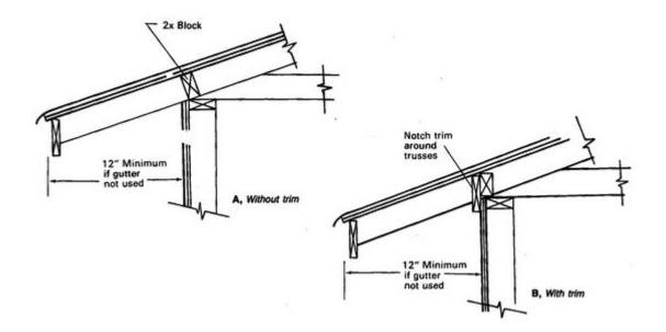
On cornices without horizontal lookout members, the soffit continues its slope up the rake overhang
