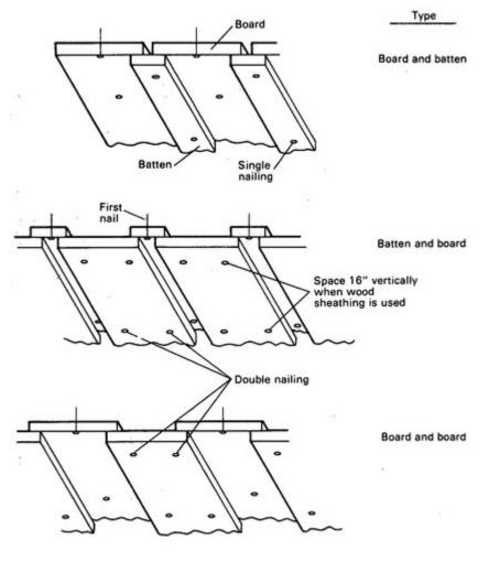
Note: Nail for first board - 8d or 9d Nail for second board - 12d
