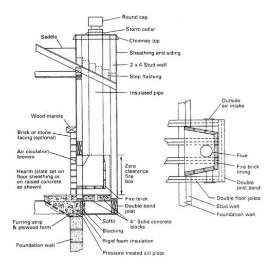
**Safe distance from ceiling.** Uninsulated steel flue pipes should not be closer than 3 feet from ceilings.
