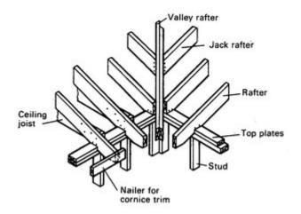
Frequently, one end of the rafter bears on exterior walls and the other end bears on a ridge beam. Sometimes intermediate beams are also used. There is no need for horizontal ties because the rafters are supported on both ends and the weight from the roof is carried to beams and posts in the center of the house as well as to the outside walls. Ceiling joists and collar ties can be eliminated.
