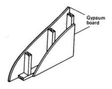
**Figure** wall with gypsum board on both sides has an STC rating of 32 to 36. Adding a second layer of gypsum board to each side
