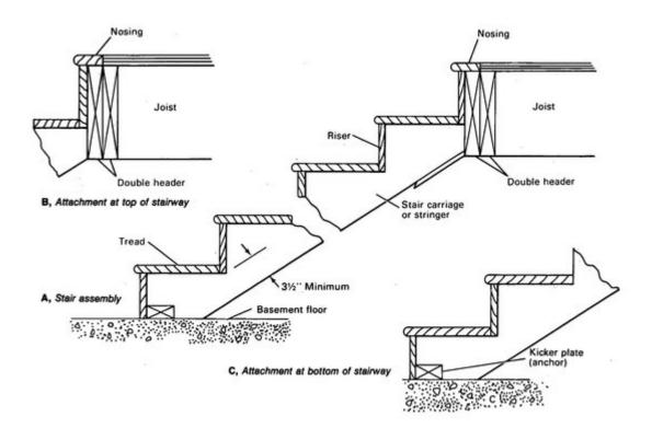
Both of these stringer layout methods presume that the stringer is to be cut so that the treads can be placed directly on the cuts. This type of stairway is referred to as an open stringer design, The alternative is the closed stringer stairway in which the stringer is not cut.
