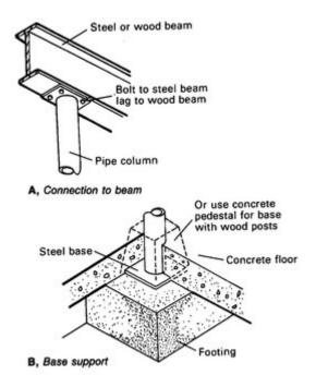
Figure post support for wood beam:
