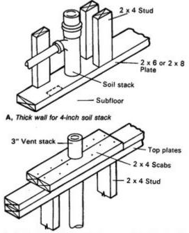
B, Reinforcing scabs for 3-inch vent stack in 2 by 4 wall
