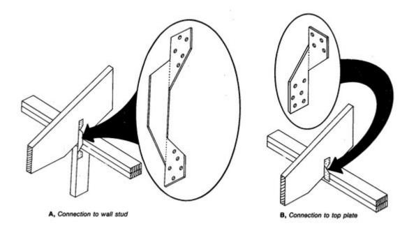
Figure used to attach trusses or rafters to the wall:
