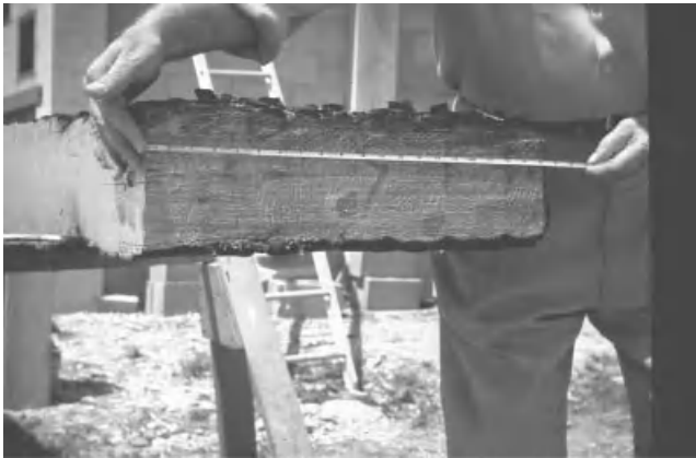
Figure 20.5-2 Char measured approximately \frac{3}{4} in. on each of three exposed sides after 30-minute fire.
