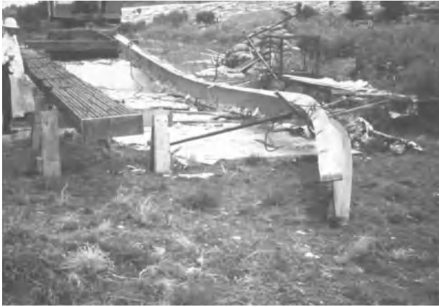
Figure 20.5-1 After 30 minutes, glulam remained straight and supported its load while steel beam collapsed.
