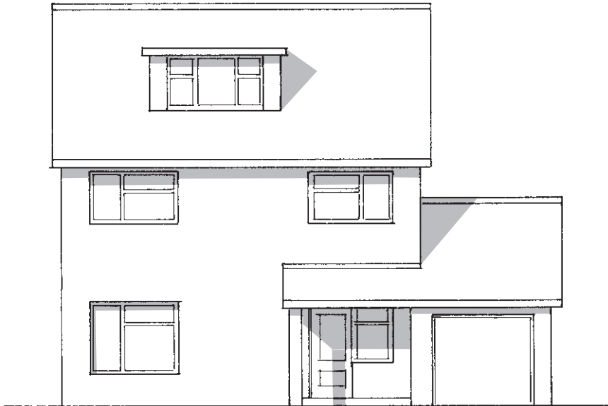
Fig.10.1 Poor dormer design.
