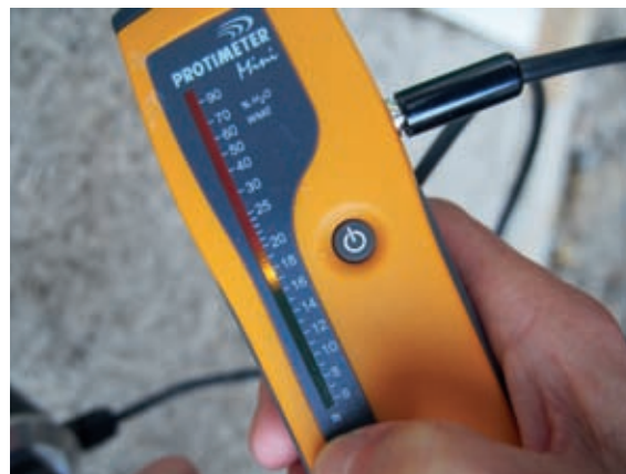
Moisture reading for a pretty dry hempcrete wall.
