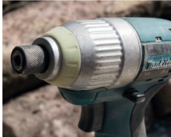
Impact drivers are useful for framing and erecting shuttering.
