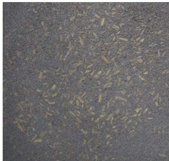
A lime–hemp basecoat plaster created from raw materials on-site.
