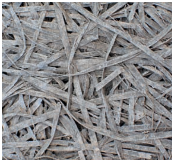
Wood wool board's open structure provides good breathability and an excellent key for lime plaster, just like hempcrete.
