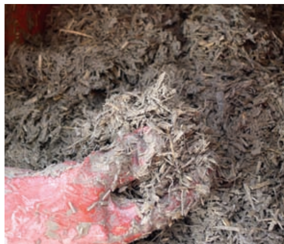
Freshly mixed hempcrete should not be too wet. The method of testing for the correct water content is discussed in Chapter 15.
