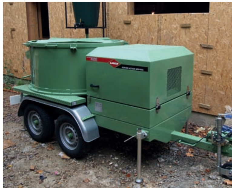
A large pan mixer is ideal for mixing hempcrete.
