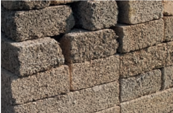
Hempcrete blocks waiting to be laid.
