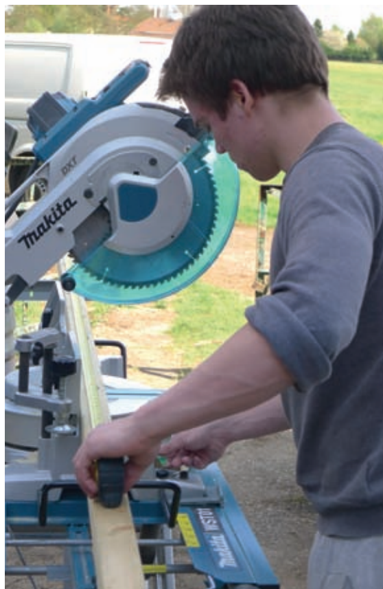
A large slide mitre saw can speed up the work considerably.
