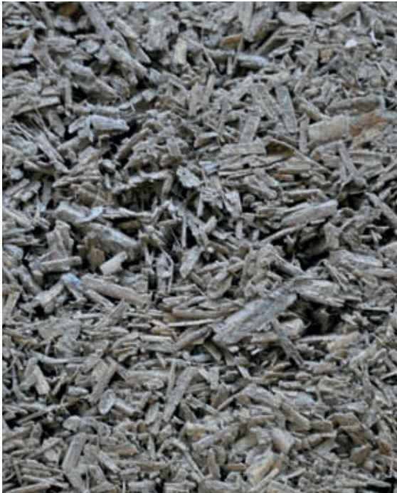
The open matrix structure of hempcrete assists vapour permeability.
