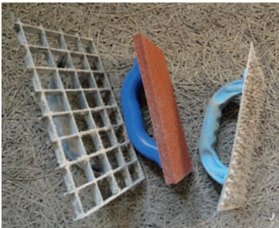
Grid, sponge and nail floats: used for finishing plaster and shaping hempcrete.
