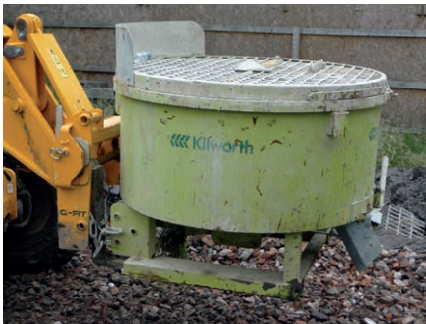
A pan mixer on a telehandler is convenient, as it can be used at different heights.
