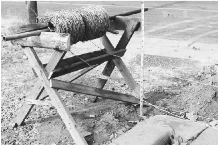
2.19: Buck stand converted into a barbed wire dispenser.
