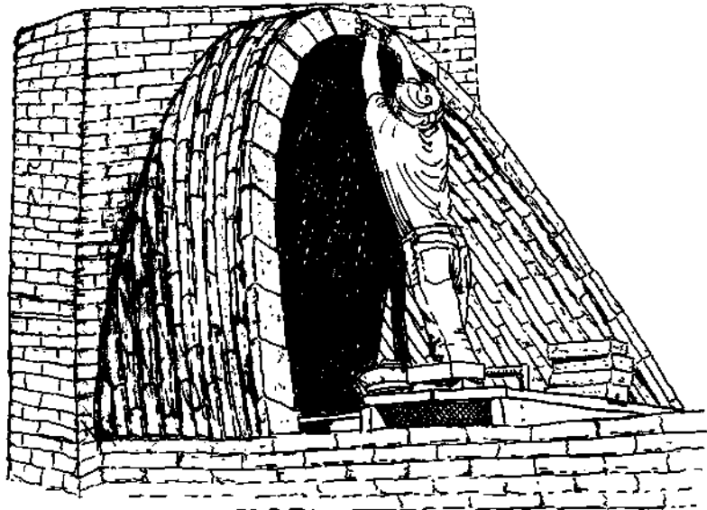
10.14: Nubian masons incorporated the catenary curve in the construction of leaning vaults.
