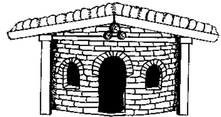
9.26: Low profile square roof supported on exterior post and beam framework with optional straw bale "living roof."
