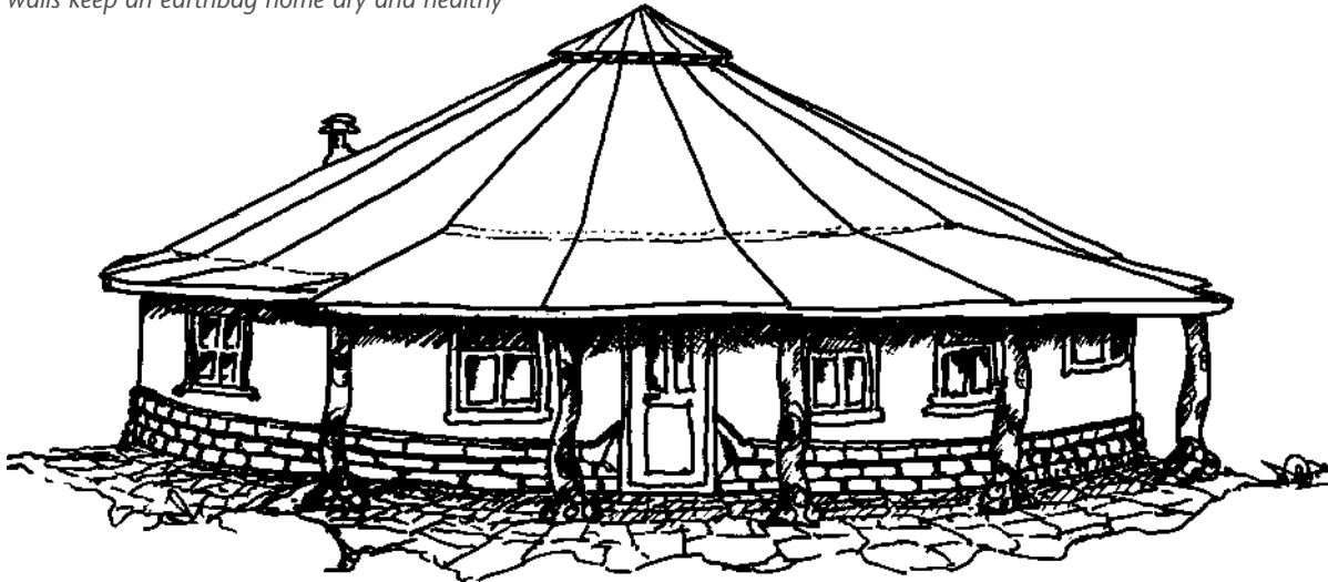
17.4: Long overhangs, porch roofs and tall stem walls keep an earthbag home dry and healthy
