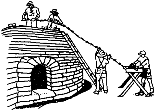
12.27: Laying barbed wire at this height is easiest done with the reel safely located on the ground.
