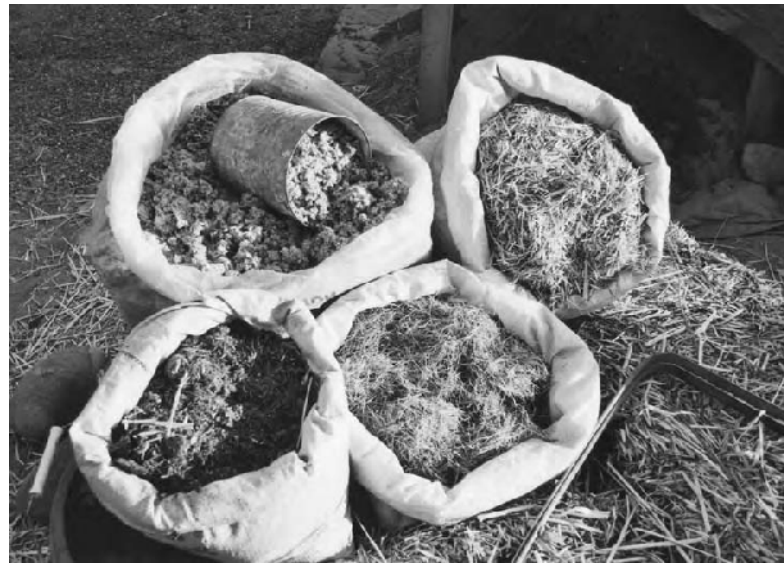
14.4: A variety of well-graded fibers for making plaster: clockwise from upper left; paper cellulose, chopped straw, long straw (on ground), sun-bleached grass clippings, and horse manure.
