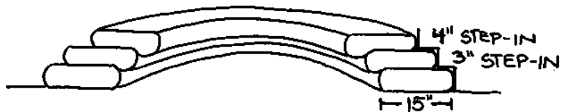
12.1: Corbelling simulation test done on the ground with 15-inch working-width tubes. Get a feel for the corbelling technique and test the behavior of your soil.
