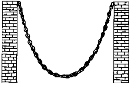
10.11a (above): A chain hung between two points creates a catenary curve, an arc in complete tension.
