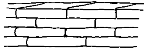
vertical seams secure a tight fit during tamping EQSS!
