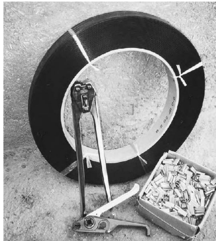
9.12: Assembly of banding (strapping) tools. Tensioner, 1,300 feet (390 m) of strapping (600 lb capacity), crimps, and crimping tool cost about $130. Compare this to the cost of a concrete beam.
