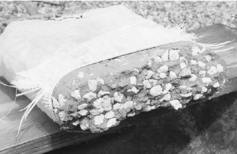
4.16: The pumice/earthbag cures hard and flat and holds together like a typical rammed-earth mix.
