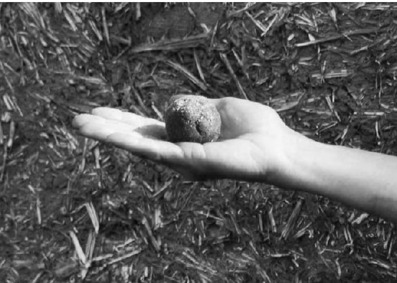
2.6: Squeeze a sample of the earth in your hand. There should be enough moisture that the soil compacts into a ball.
