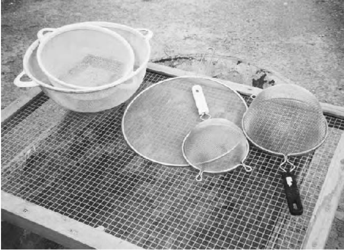
15.6: We practice a fairly rustic style of plaster, using mostly a 1/8-inch to 1/16-inch wire mesh kitchen colander for screening our finish plasters.
