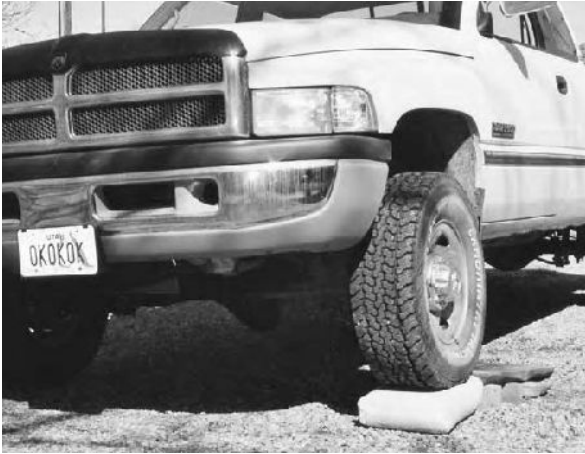
2.10: (top) This informal test demonstrates the weight of a 3/4-ton truck on top of a fully cured earthbag, resulting in no deformation whatsoever.
