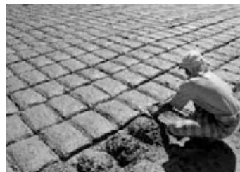
For thousands of years, mud bricks have been shaped by hand and allowed to dry in the sun to create a durable and long-lasting building unit.
