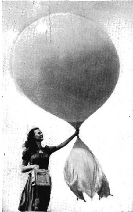
Fig. 19.8. Observer is ready to release balloon with parachute and radiosonde attached. (Courtesy U. S. Weather Bureau)
