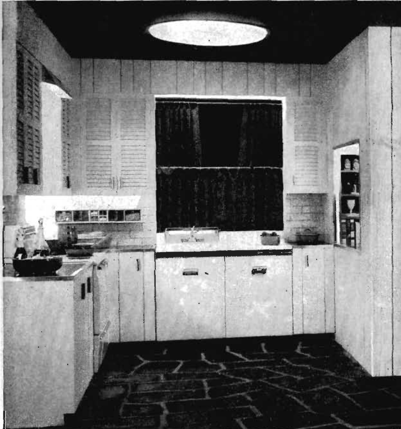
Fig. 37.11. This kitchen has a ceiling fixture, 36 inches in diameter, to give over-all lighting throughout the room. (Courtesy General Electric Company)
