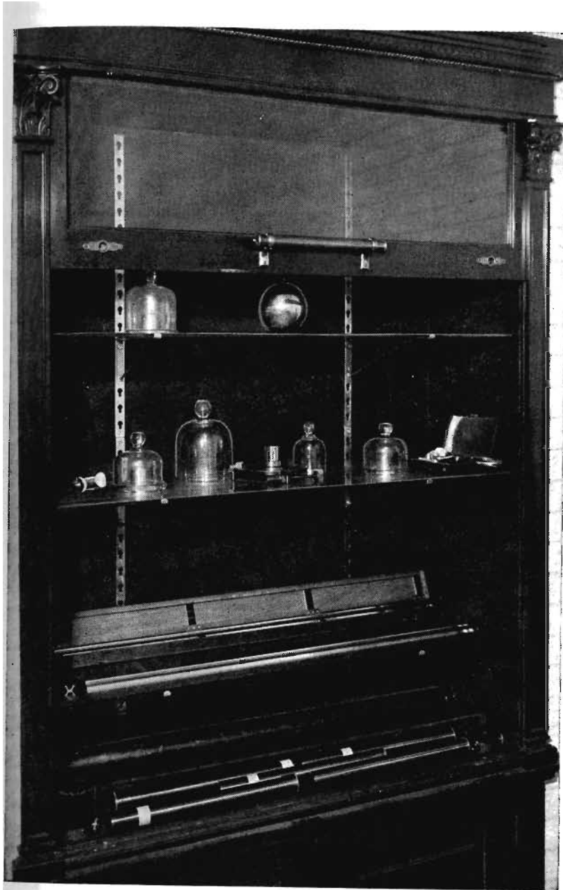
Fig. 1.2. View in the vault at the National Bureau of Standards, showing the standards of length and mass of the United States. (Courtesy National Bureau of Standards, U.S. Department of Commerce)
