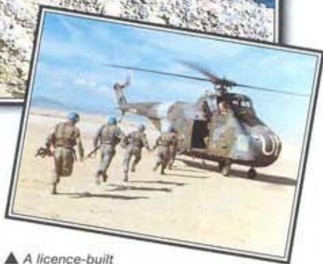
▲ A licence-built Sikorsky design, the WS-55/Whirlwind served the British armed forces for many years, mainly in transport, anti-submarine warfare and rescue roles.
