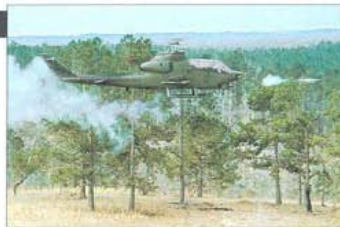
The HueyCobra unleashes a deadly BGM-71 TOW (Tube-launched Optically-tracked Wire-guided) missile towards an unsuspecting tank. It is guided to the target by a trailing wire.
