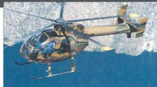
Military interest in the NOTAR system remains limited. However, the US Army conducted experiments with the concept for special operations, where its low noise was a useful asset.
