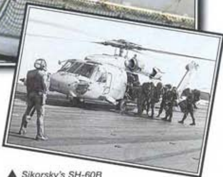
▲ Sikorsky's SH-60B filled the US Navy's LAMPS (light airborne multi-purpose system) III requirement for a helicopter with over-the-horizon search-and-strike capability.
