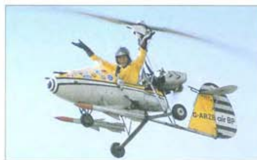
Left: The WA-122 was a two-seat design with dual controls, making it suitable as a trainer. It is powered by a larger Rolls-Royce Continental 119-kW (160-hp.) flat-four engine.
