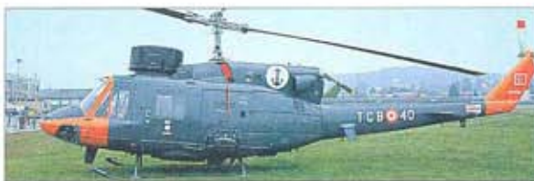
Left: The Turkish navy bought 12 AB.212ASWs, which serve aboard 'Yavuz'-class frigates. These are fitted with British-built Sea Spray radar and Sea Skua air-to-surface missiles.
