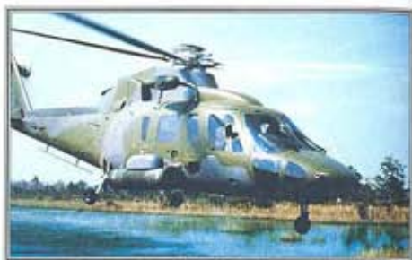
◀ New York bird This Heli Union S-76C is powered by Turboméca Arriel turboshafts. The S-76C first flew in 1990, and has also been sold to the Spanish air force.
