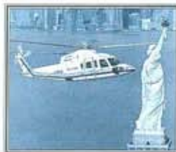
◀ New York bird This Heli Union S-76C is powered by Turboméca Arriel turboshafts. The S-76C first flew in 1990, and has also been sold to the Spanish air force.
