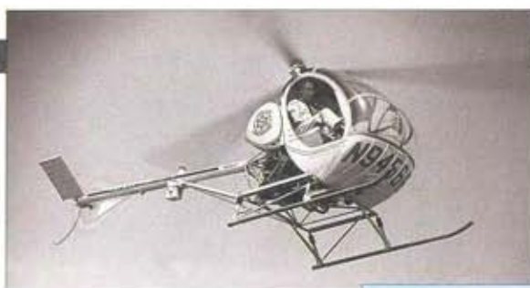
Above: This Hughes 300, based at Lakewood, Los Angeles, is fitted with a searchlight, a siren and warning light. Police versions often carry armour.
