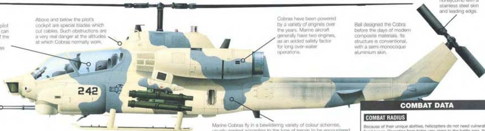
The stub pylons provide not only the means to carry a large weapon load but also act as miniature wings, providing valuable extra lift when the Cobra is in forward flight.
