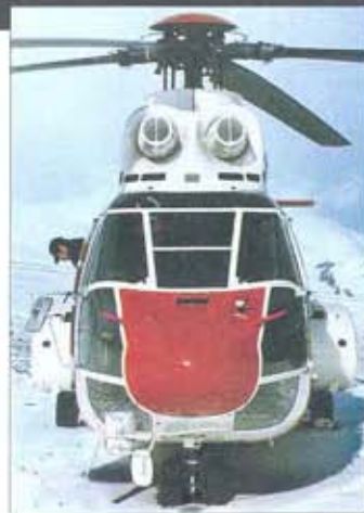
Right: An increase in the nose volume of the Super Puma has allowed the type to be fitted with a weather radar.
