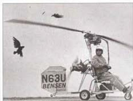
Bird strike tests: What happens when a bird flies into the rotor of a B-8M Gyro-copter? The bird comes out second best! Although this picture may appear rather brutal, tests conducted by Bensen Aircraft showed that, on average, three out of four birds would survive such an incident unscathed. Bensen made it clear that no live birds were used during the experiments. The primary objective was to test the strength of the rotor blades.
