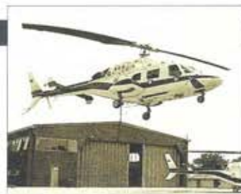
The Bell 222 is an excellent choice for a police helicopter, having twin-engined clearance for work over crowded cities, and enough capacity to carry dog teams or special firearms officers if needed.
