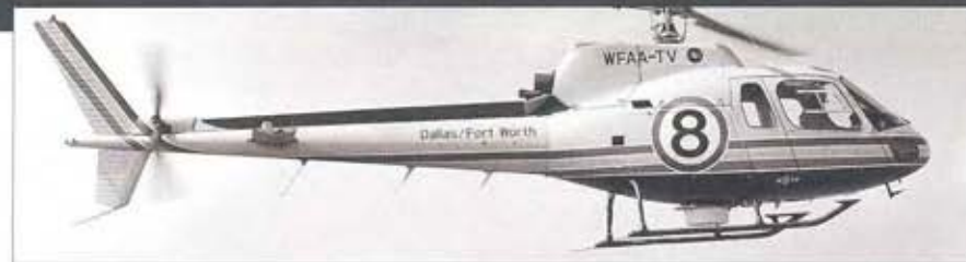
Above: Some TV broadcasters use their helicopters as relays for signals transmitted from the ground. This system is especially useful for live broadcasts from built-up areas.
