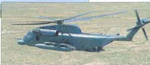
Above: With weapons fitted in all positions, this 'Super Jolly' shows a typical configuration for special forces operations. MH-53Js often fly alone on such missions.
