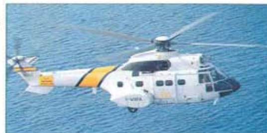
Above: The AS 332M incorporated a .76-m (30-in.) fuselage stretch, allowing it to carry four additional passengers.
