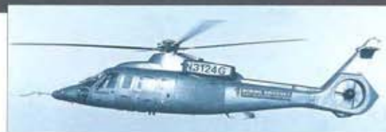
Above: This 'fantail' variant was fitted with a fenestron-type tail rotor in trials for the Light Helicopter Experimental programme.
