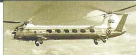
Above: British European Airways evaluated the Alvis Leonides-powered Type 173. The dihedral tailplanes were a feature of the early prototypes.
