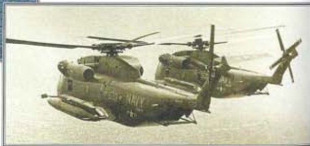
▶ Joint exercises Operating with the Spanish navy on joint minesweeping duties, these two examples are fitted with additional fuel tanks on pylons to increase their sweep area.
