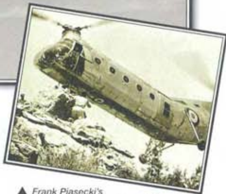
▲ Frank Piasecki's H-21/HRP made use of the designer's well-known tandem rotor layout, perpetuated in the later Vertol H-25/HUP, H-46 and H-47 designs.
