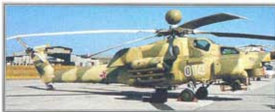
▲ Production version Mil upgraded the equipment fit of the Mi-28 to produce the much more capable Mi-28N. This has improved avionics and weaponry and an all-weather capability.
