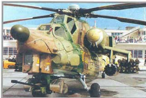
▲ Turret-mounted gun The Mi-28's 30-mm NPPU-28 cannon has air-to-air capability and can fire up to 900 rounds per minute. Its ammunition is compatible with Russian armoured vehicle weapons.
