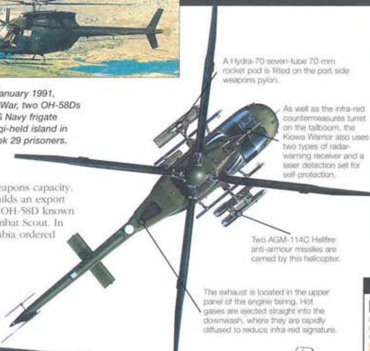
The OH-58D's key sensors are located in the mast-mounted sight. Behind the two windows are a TV sensor and an imaging infra-red, which provide targeting and navigational information in all light and weather conditions.
