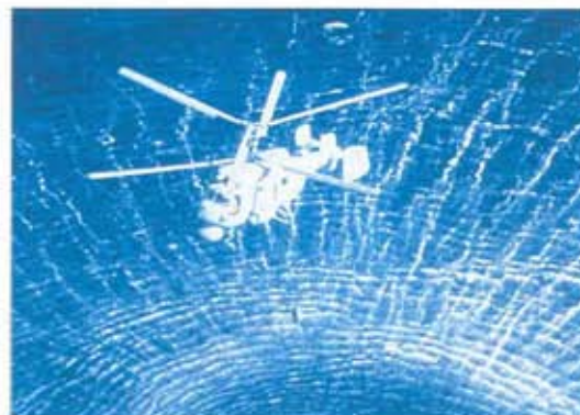
The Ka-25 lowers its dipping sonar into the sea for an 'active' search. The 'Hormone' uses its passive sonobuoys for a first search, and then active sonar and magnetic anomaly detection in the closing stages of an attack.
