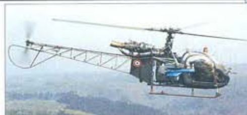
Above: In the military role, Alouette IIs can be fitted with a variety of rockets, missiles and guns. This machine carries SS.11 anti-tank missiles.
