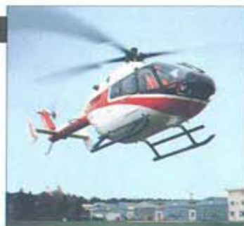
Above: Eurocopter added an advanced fenestron anti-torque system to the MBB BO 108.
