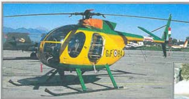
▲ Italian patrol The Italian air force also uses the OH-6. This one has a bubble-type observation window on the port side.
