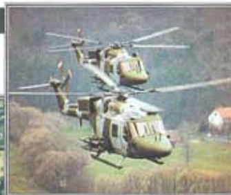
▲ Combat ready Infra-red exhaust suppressors, a roof-mounted sight and TOW missiles make the Lynx AH.Mk 7 a formidable weapon system.
