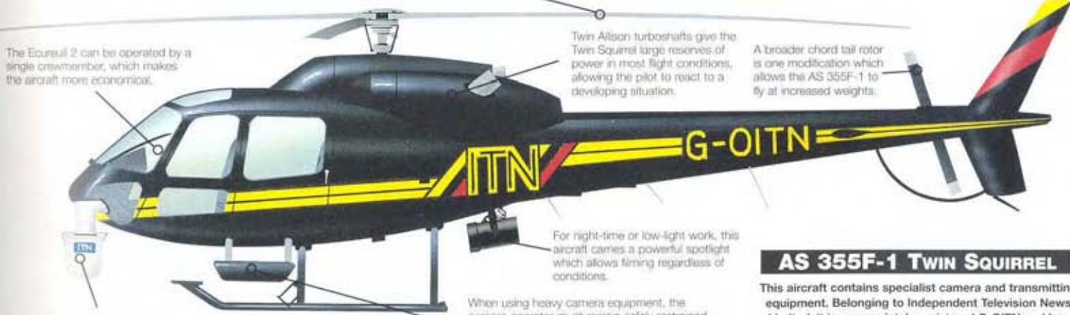
Above: This is ITN's AS 355F-1 in action. A special seat is installed to allow the camera operator to work in safety from the open door.
