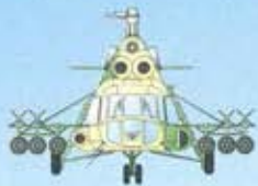
Mi-8 'HIP-E': Probably the most heavily armed helicopter in service, the 'Hip-E' carried up to six pods of 32 rockets.
