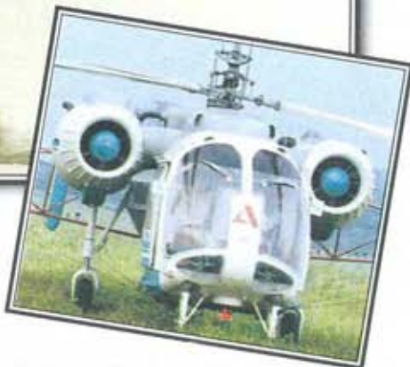
▲ The layout of the Ka-26 'Hoodlum' has resulted in a practical helicopter which has sold well in at least 15 countries. It has a capacious fuselage and is easily adapted to different roles
