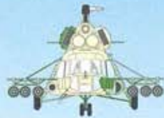
Mi-17 'HIP-H': The Mi-17 featured new engines, gearbox and rotor shaft and was a lot more powerful and economical than the Mi-8.
