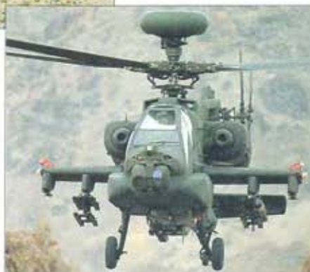
Below: An AH-64A test helicopter was equipped with the Longbow radar to undertake flight handling characteristics tests.
