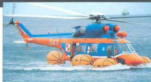
Above: With flotation gear inflated, this Anakonda demonstrates its amphibious abilities in the rescue role.
