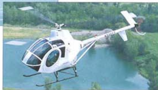
Left: An interesting and practical feature of the 330 is its ability to run on turbine fuel instead of Avgas if the operator wishes.
