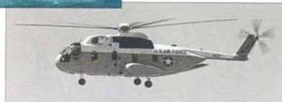
Above: CH-3Es also carried a winch above the starboard forward door, adding extra flexibility and giving the helicopter a secondary SAR role.
