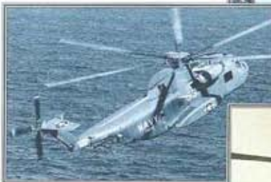
▶ Joint exercises Operating with the Spanish navy on joint minesweeping duties, these two examples are fitted with additional fuel tanks on pylons to increase their sweep area.
