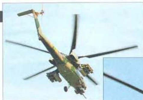
Above: The Klimov TV3-117 turboshafts power a five-bladed composite main rotor and a scissor-type tail rotor. This system, and a fenestron tail rotor, were both first tested on an Mi-24 'Hind' development aircraft.
