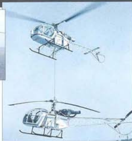
Above: Here a Lama demonstrates its ability to lift the weight of an Alouette II (around 895 kg/1,970 lb. empty). The Lama can be distinguished from the earlier machine by its three-bladed tail rotor.
