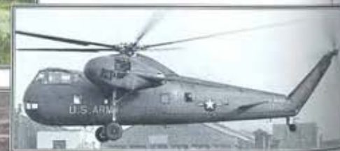
◀ Early warning variant Two HR2S-1Ws, with APS-20E radar scanners fitted, were evaluated by the US Navy. However, airframe vibration badly degraded radar performance.
