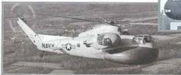
◀ Early warning variant Two HR2S-1Ws, with APS-20E radar scanners fitted, were evaluated by the US Navy. However, airframe vibration badly degraded radar performance.
