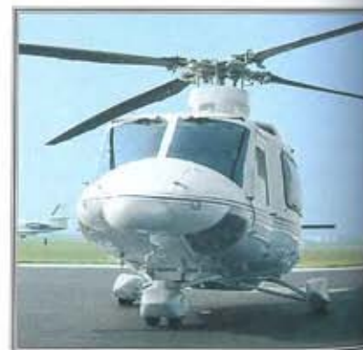
▲ Fire fighter For the fire-bombing role, the Model 212 may be fitted with high ground-clearance skids to accommodate an under fuselage water tank.
