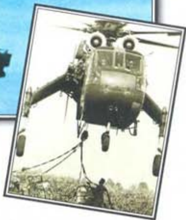
▲ Groundcrew prepare the Tarhe to lift another massive load. A cargo net is used to gather lots of items together so that they can all be lifted at once.
