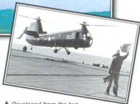
▲ Developed from the two XHJP-1 prototypes (Piasecki's Model PV-14), the HUP Retrievers earned their keep as 'planeguards' and rescue craft aboard the US Navy's carriers.
