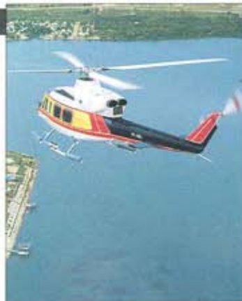
Above: Differing from the military 212 in cabin furnishing and avionics, the 14-seat commercial version is also known as the Twin Two-Twelve.
