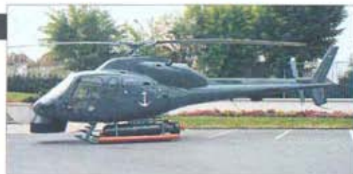
The naval AS 355M2 has a chin-mounted 360° radar and can be armed with a pair of lightweight homing torpedoes. This version is in use with the Brazilian navy, which operates 11 UH-12Bs.
