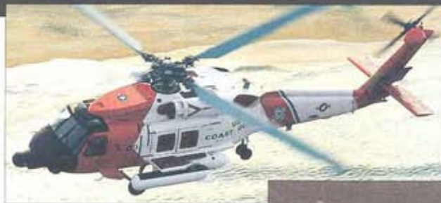
Above: HH-60Js have somewhat larger sponson tanks because of their greater endurance requirements.
