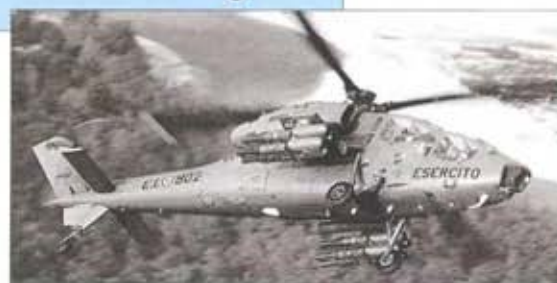
Right: Although fully armed, the second prototype did not represent the final production standard. Current aircraft carry a Saab/ESCO HeliTOW sight above the nose.
