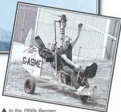
▲ In the 1950s Bensen Aircraft of Raleigh, North Carolina developed the concept of a low-cost, home-built gyrocopter which did not require a pilot's licence to be flown.
