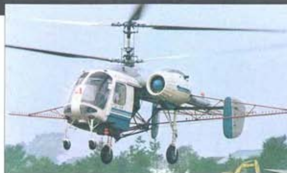
For crop-spraying the Ka-26 can carry 900 kg (200 lb.) of liquid, and when used as a duster capacity increases by 165 kg (360 lb.). Most Russian Ka-26s are used to treat orchards and vineyards.
