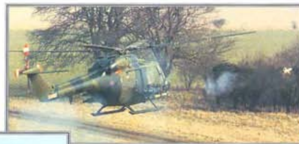
▲ TOW attack Using natural cover as its only defence, a Lynx AH.Mk 1 unleashes a TOW missile at an unsuspecting tank. The missile's guide wires can just be seen at the mouth of the launch tube.
