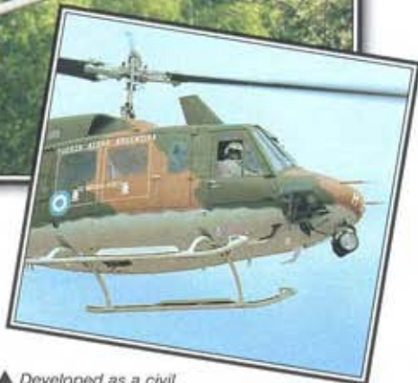
▲ Developed as a civil version of the UH-1N, the twin-turboshaft Model 212 has found military operators, too, and has been successfully followed by the more powerful single-engined Model 214.
