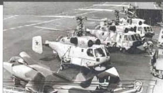
The flight deck of the Russian carrier Kuznetsov accommodates (left to right) a Yak-38 strike fighter, Ka-27PL ASW helicopter, Ka-29 assault transport and an electronic warfare Ka-31.
