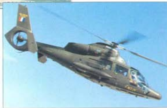
Above: Most armed Panthers are naval aircraft, but army versions can carry GIAT 20-mm cannon pods, MATRA Mistral missiles or unguided Thomson-Brandt 68-mm rockets.
