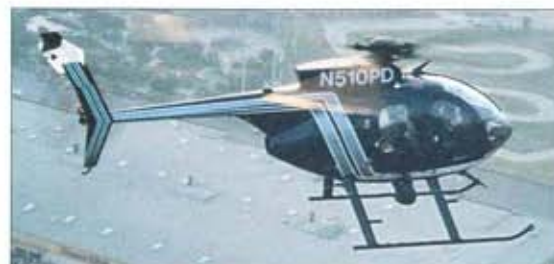
Below: A major user of the 500 family have been police forces. This MD500E belongs to Oakland, California's Police Department and carries a spotlight under the cabin and wire cutters above and below the windscreen. Military MD500s are used in Colombia, Japan, Kenya, the Philippines and South Korea.
