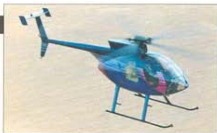
Above: Another popular use is that of executive transport, like the rival Bell 206. This smartly painted MD500E has extra clearance 'tall' skids.
