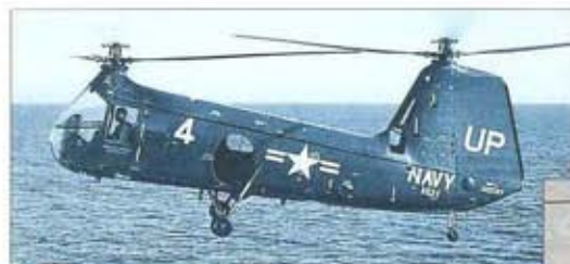
Above: Several US Navy HUP-2s had dunking sonar fitted for anti-submarine operations and were designated HUP-2S.
