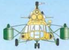
AWACS HIP: The Mi-17 was even converted to act as an airborne early warning and control machine with side-mounted radar aerials.
