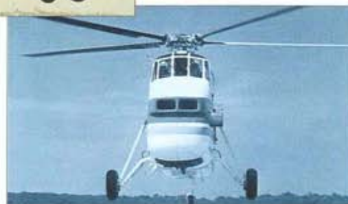
Above: The S-58T conversion is powered by a Pratt & Whitney Canada PT6T-3 Twin Pac coupled-turbine engine. Only a small number of customers have been found.
