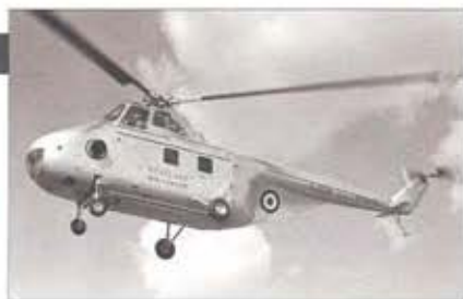
Left: XJ398 was one of three Whirlwind Mk 3s used by Westland to develop a turboshaft-powered WS-55 with considerably improved performance.
