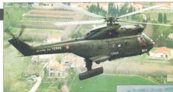
Left: The French Orchidée battlefield surveillance radar program was shelved in 1990, but was revived during Operation Desert Storm. The system was carried aboard a Puma.
