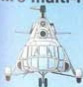
Mi-8 'HIP-A': The first Mi-8 was the single-engined prototype that lacked power and only had a four-bladed main rotor.
