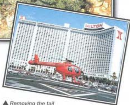
▲ Removing the tail rotor helps the NOTAR helicopter to operate from confined spaces. This has proved to be very convenient for commercial flight operations within large cities.
