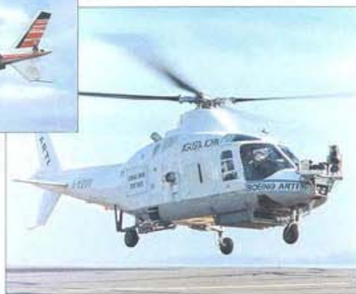
Above: A modified A 109 was used as Boeing's Advanced Rotorcraft Technology Integration (ARTI) testbed. The pilot was situated in the passenger cabin and had no external view; he used the cameras on the nose to fly the aircraft.
