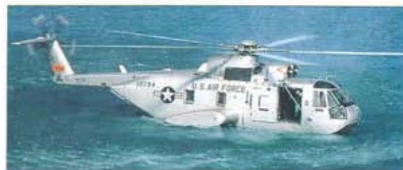
Above: CH-3Es also carried a winch above the starboard forward door, adding extra flexibility and giving the helicopter a secondary SAR role.
