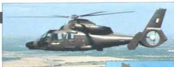
Left: Survivability was a high priority. Seats were designed to withstand a 20g impact and the fuel system a crash at 14 m/sec (45-f.p.s.).
