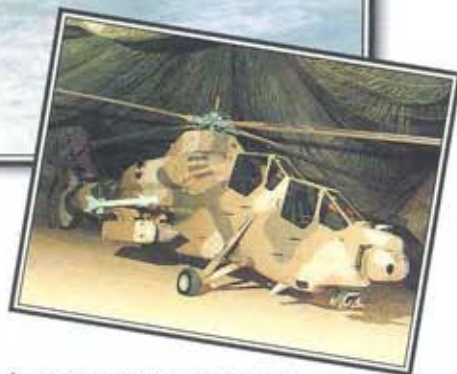
▲ A fully armed Rooivalk carries V3C Darter air-to-air missiles, pods of 68-mm unguided rockets, enclosed four-round 80-mm anti-tank missile pods and a chin-mounted cannon.
