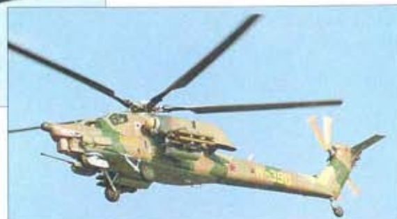
Above: For longer range missions the Mi-28 can carry up to four external fuel tanks. Designed to be capable of autonomous battlefield operations, it also has an internal weapons hoist.
