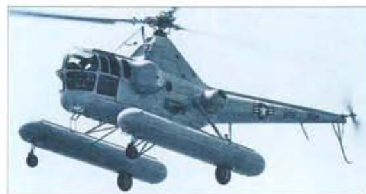
Above: The first amphibious helicopter for US service, the new wheel/float combination of the Sikorsky design greatly improved its capabilities.
