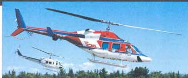
Left: The 230 is distinguished from the 222 by its revised engine air intakes and repositioned exhausts.
