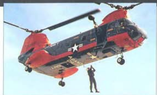
Painted in a high-visibility orange paint scheme, this Sea Knight is an HH-46 variant; 38 of these aircraft were modified to this standard. Many are based at Point Mugu, California, for search-and-rescue duties.
