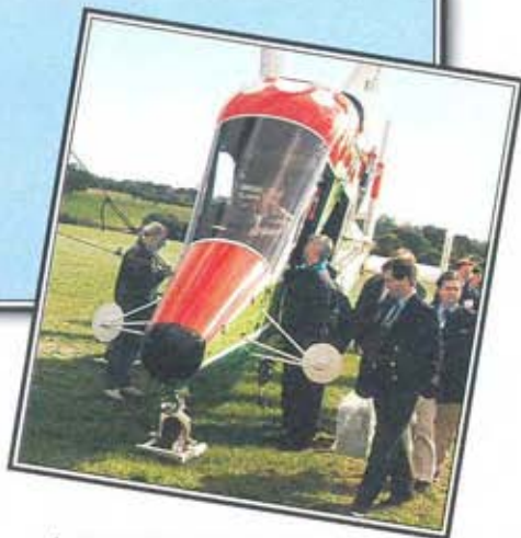
▲ 'WARNING: APPROACH FROM FRONT' reads the legend below the aircraft's rotor. While on the ground, the intermeshed rotors pass much lower than those on conventional helicopters.
