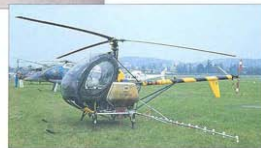
The Hughes 300 series tail rotor is of the teetering type, with just two blades freely pivoted as one unit. Each comprises a steel tube spar with glass-fibre skin. A spring-mounted bumper protects the blades.
