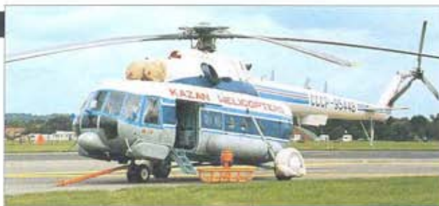
Left: Kazan Helicopters build the standard Mi-17M. This one contains a weather radar in the nose.
