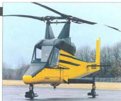
Above: Kaman's helicopter designs have been intended to fill market niches. The company's vast experience with intermeshing rotors benefited the K-MAX design.
