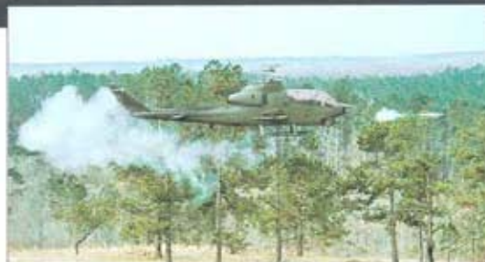
Helicopter killer – the HueyCobra can carry the Sidewinder missile on its stub pylons to shoot down other helicopters.
