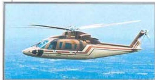
◀ New York bird This Heli Union S-76C is powered by Turboméca Arriel turboshafts. The S-76C first flew in 1990, and has also been sold to the Spanish air force.
