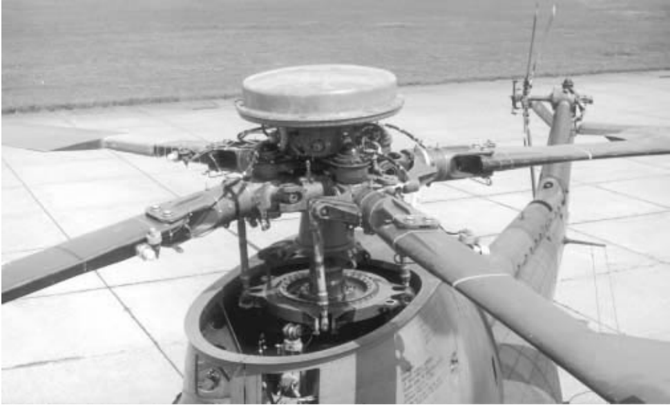
The instrumented rotorhead of the DRA (RAE) research Puma (Photograph courtesy of DRA Bedford)
