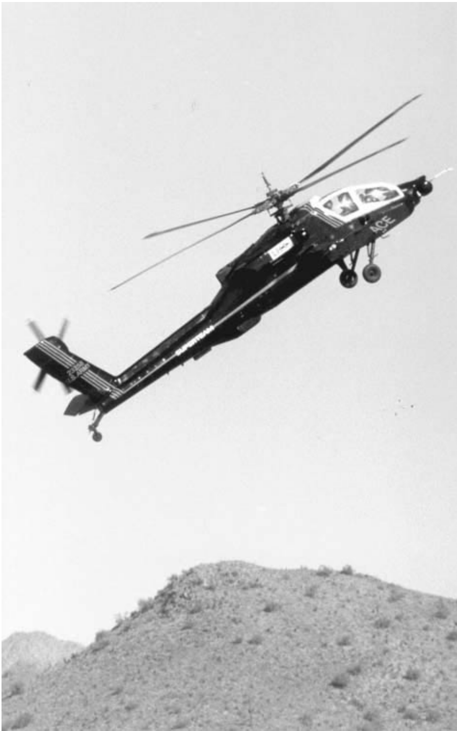
The MDHC variable stability (fly-by-wire) Apache AV05 during a handling qualities evaluation over the Arizona desert (Photograph from the author's collection)
