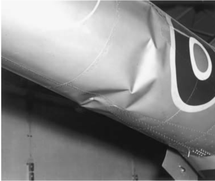
Fig. 2.38 Fuselage failure on Sikorsky S-51 (Ref. 2.31)
