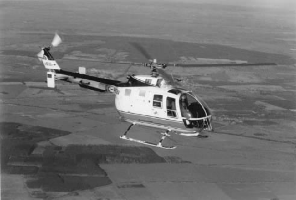
The German DLR variable stability (fly-by-wire/light) Bo105 S3 (Photograph courtesy of DLR Braunschweig)
