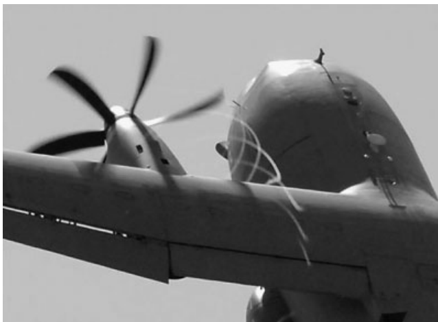
Figure 1.19 Propeller tip vortices
