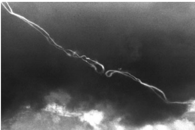
Figure 1.21 Wing tip vortices (BAE Hawk 200)
