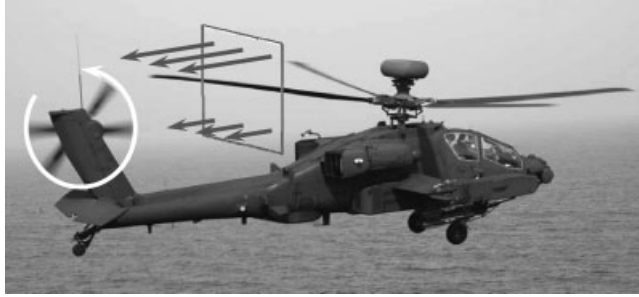
Figure 6.15 Incident flow over tail rotor (Courtesy US Navy)
