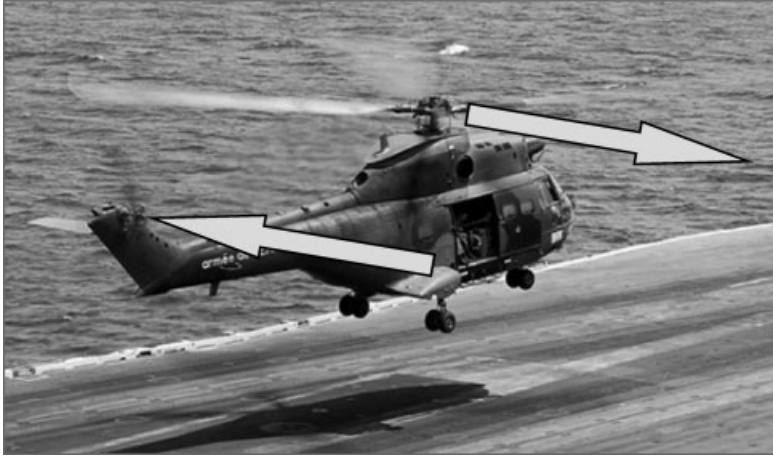
Figure 6.13 Puma hovering showing tail rotor thrust direction and opposing main rotor side force (Courtesy US Navy)
