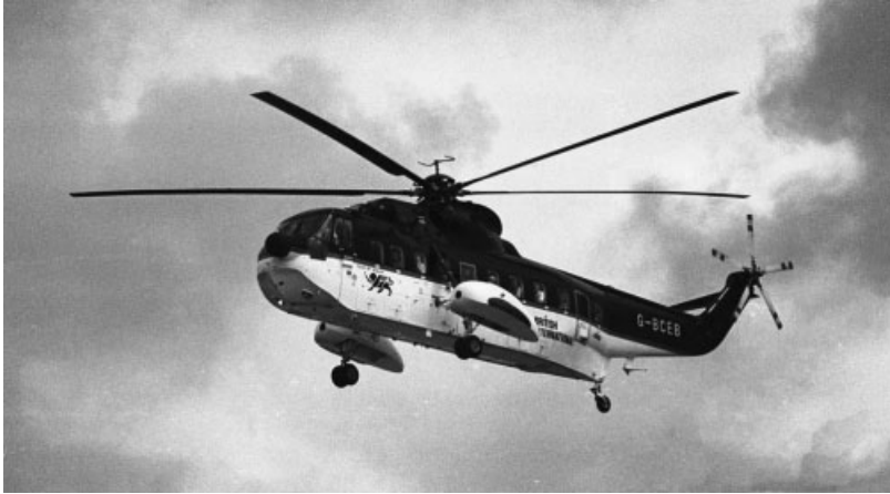
Figure 6.6 Rectangular blade planform of S61NM helicopter
