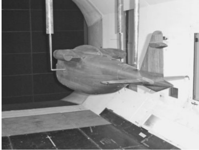
Figure 6.30 Pathfinder fuselage model in University of Southampton 11 ft by 8 ft wind tunnel
