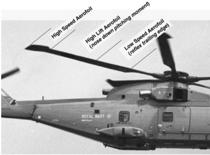
Figure 6.3 Spanwise variation of the aerofoil sections on the Merlin main rotor blade
