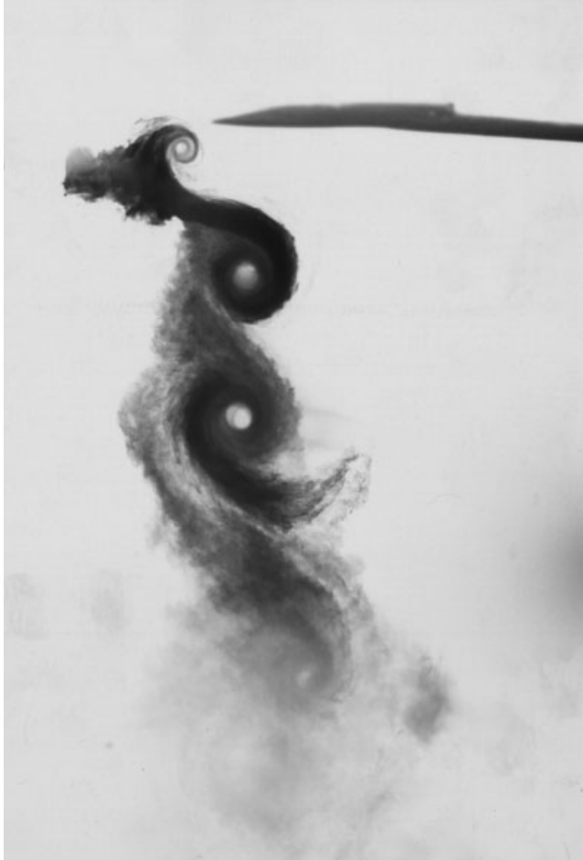
Figure 2.26 Real rotor wake
