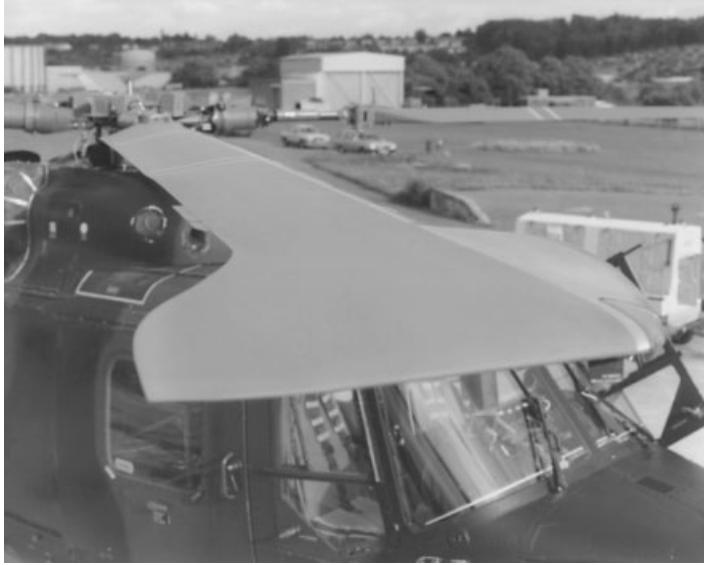
Figure 7.8 BERP rotor blade on world speed record helicopter (G-LYNX) (Courtesy Agusta Westland)
