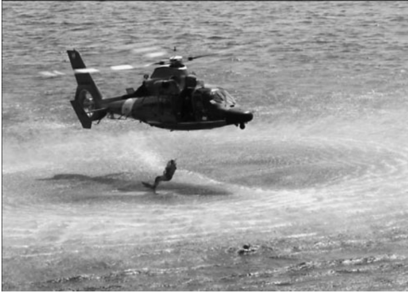
Figure 2.31 Hovering close to water surface showing wake impingement (Courtesy US Navy)
