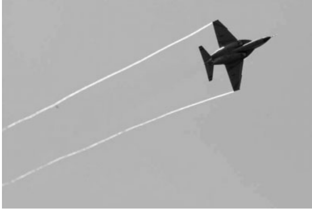
Figure 1.18 Tip vortices generated by a fixed-wing aircraft
