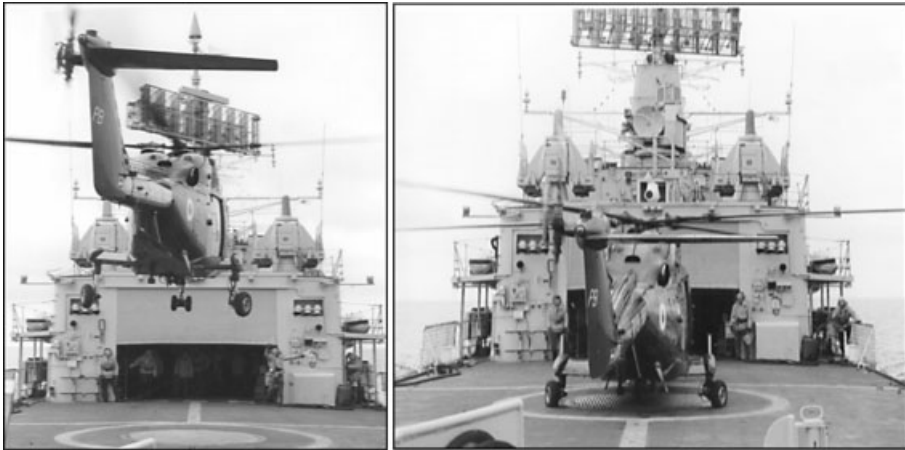
Figure 7.11 A Lynx landing on deck showing the operation of the undercarriage (Courtesy Agusta Westland)
