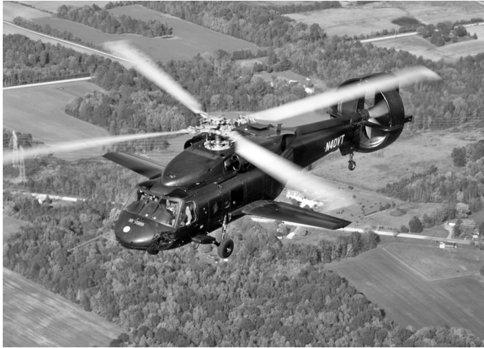
Figure 9.2 S-70 Blackhawk compound development aircraft (Courtesy Piasecki Corp.)
