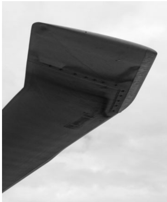
Figure 6.7 Simply swept rotor blade tip
