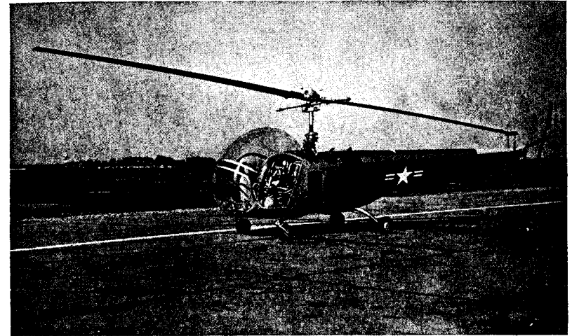
Fig. 2-1 Bell H13-B single-rotor helicopter. Courtesy NACA.
