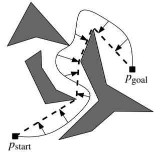
**Lemma 15.1** Any shortest path between  $p_{\text{start}}$  and  $p_{\text{goal}}$  among a set  $S$  of disjoint polygonal obstacles is a polygonal path whose inner vertices are vertices of  $S$ .
