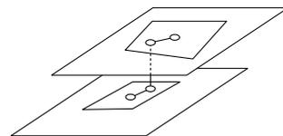
$\mathcal{G}_0$  in the same way. Note that paths in the graph  $\mathcal{G}_{\text{road}}$  correspond to paths of the robot that are composed of purely translational motion (when we move along an arc connecting nodes in the same slice) and purely rotational motion (when we move along an arc connecting nodes in different slices).
