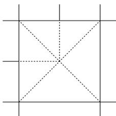
coordinates, and the polygon edges have one of four possible orientations: the angle that any edge makes with the positive  $x$ -axis is  $0^\circ$ ,  $45^\circ$ ,  $90^\circ$ , or  $135^\circ$ . The goal is to compute a triangular mesh of the square (both outside and inside the components) that is conforming, respects the input, has well-shaped triangles, and is non-uniform.
