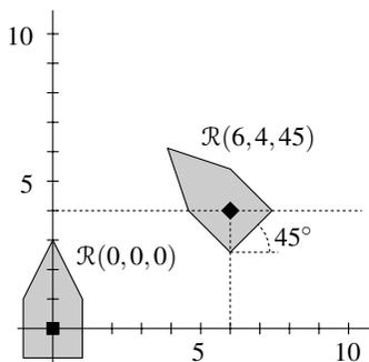
Now suppose the robot can change its orientation by rotation, say around its reference point. We then need an extra parameter,  $\phi$ , to specify the orientation of the robot. We let  $\mathcal{R}(x, y, \phi)$  denote the robot with its reference point at  $(x, y)$  and rotated counterclockwise through an angle  $\phi$ . So what is specified initially is  $\mathcal{R}(0, 0, 0)$ .
