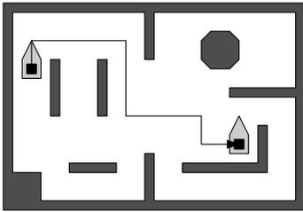
obstacles, and the robot itself will also be polygonal. We also assume that the environment is static—there are no people walking in the way of our robot—and known to the robot. The restriction to planar robots is not as severe as it appears at first sight: for a robot moving around on a work floor, a floor plan showing the location of walls, tables, machines, and so on, is often sufficient to plan a motion.
