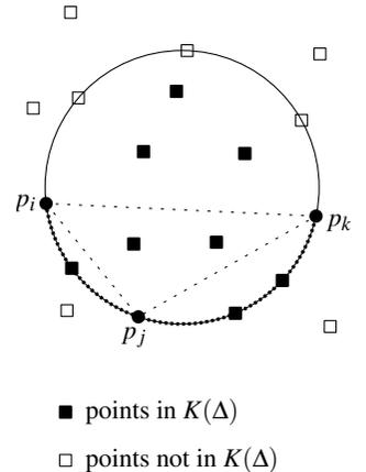
Now Theorem 9.15 applies. How many Delaunay corners are there in the Delaunay graph of  $S \cup \Omega$ ? The worst case is when the Delaunay graph is a triangulation. If  $S$  contains  $r$  points, then the triangulation has  $2(r+3) - 5$  triangles, and therefore  $6(r+3) - 15 = 6r + 3$  Delaunay corners. It follows from Theorem 9.15 that
