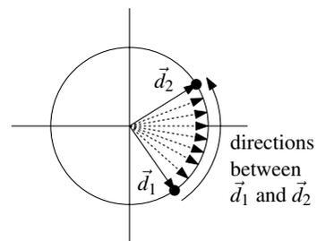
**Observation 13.7** *Let  $\mathcal{P}_1$  and  $\mathcal{P}_2$  be convex polygons with disjoint interiors. Let  $\vec{d}_1$  and  $\vec{d}_2$  be directions in which  $\mathcal{P}_1$  is more extreme than  $\mathcal{P}_2$ . Then either  $\mathcal{P}_1$  is more extreme than  $\mathcal{P}_2$  in all directions in the range from  $\vec{d}_1$  to  $\vec{d}_2$ , or it is more extreme in all directions in the range from  $\vec{d}_2$  to  $\vec{d}_1$ .*
