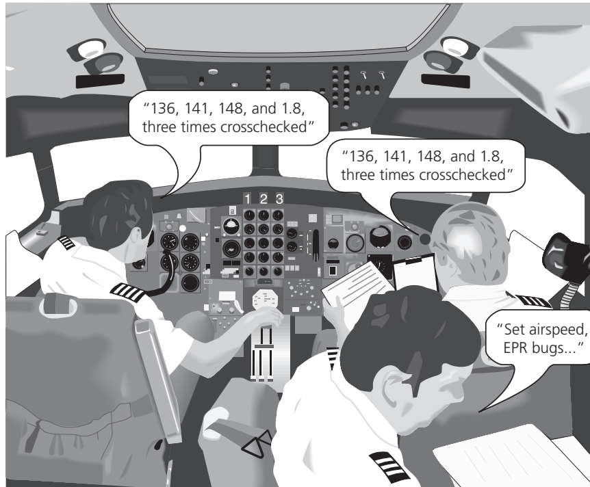
In a three-pilot cockpit the flight engineer reads the checklist, and the flying pilot and nonflying pilot respond accordingly.
