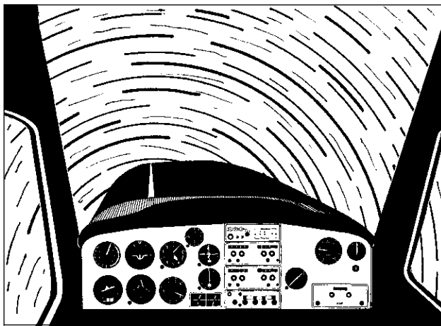
Figure 12-19. The spin as it will probably be seen from the cockpit your first time. The ball in the turn coordinator is to the left side of the instrument, you will notice, not to the right as might be assumed by theory. (You are holding full left rudder, which under normal flying conditions would put the ball to the right—but not in a developed spin with the instrument mounted on the left side of the panel, as shown.)
