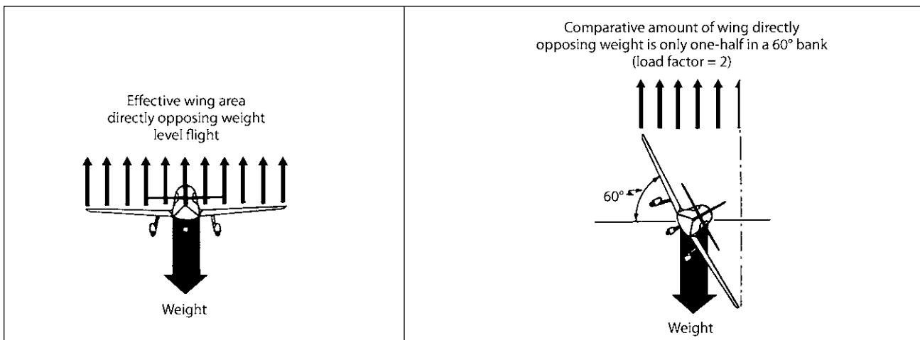
Figure 9-3. The effects of bank angle on the amount of lift that is directly opposing weight.
