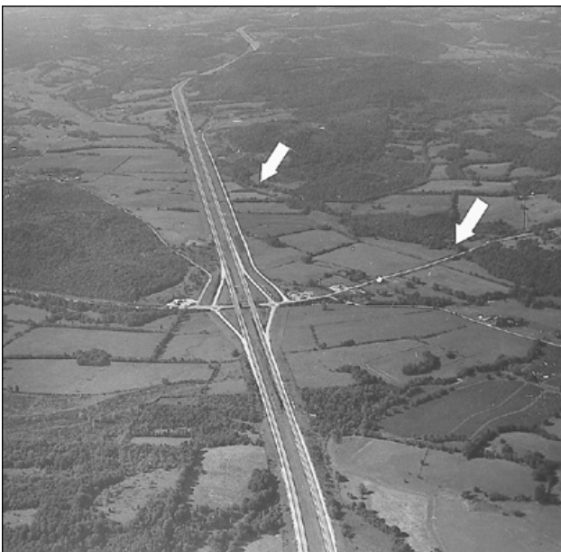
Figure 24-5. An intersection to I-65 and a secondary road 1 mile to the left (south) of the course. Note the stream in the right side of the photo (the secondary road crosses it). The stream (arrows) is not shown on the chart, but, again, you'd see it on the dual flight and make a mental note for your solo trip.
