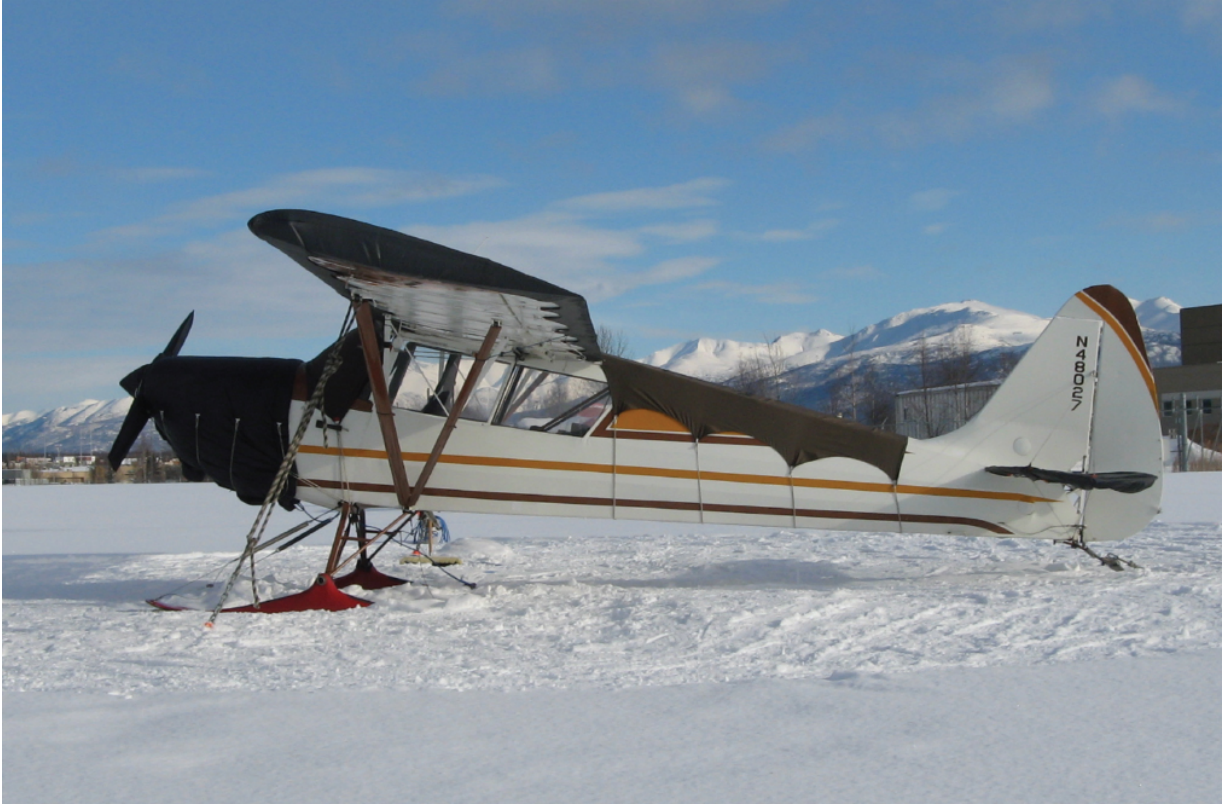
Nylon covers on the Arctic Tern at Merrill Field. Note the sculptured wing and fuselage covers. This prevents the wind from bellowing the covers. The cover over the cowling has to be wellinsulated. Insulated covers are also necessary for the propeller and nose cone. (February 23, 2013)
