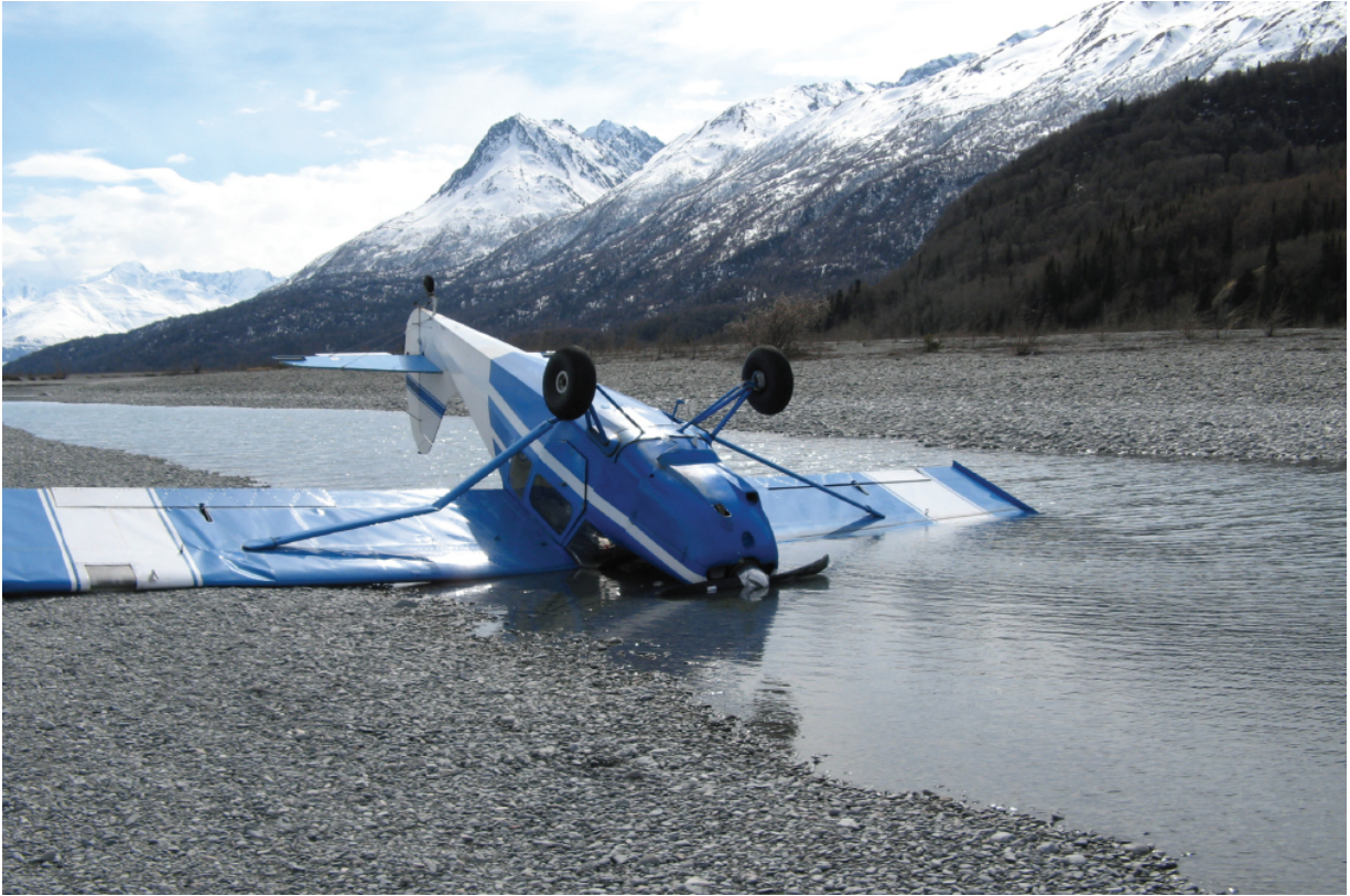
The first flight for this rebuilt and recovered Aeronca Sedan ended in an upside down airplane in the Knik River. I hope this book will help pilots to avoid this type of preventable accident—coming in for a landing too fast with the airplane abundantly overloaded with kinetic energy. (May 3, 2007)
