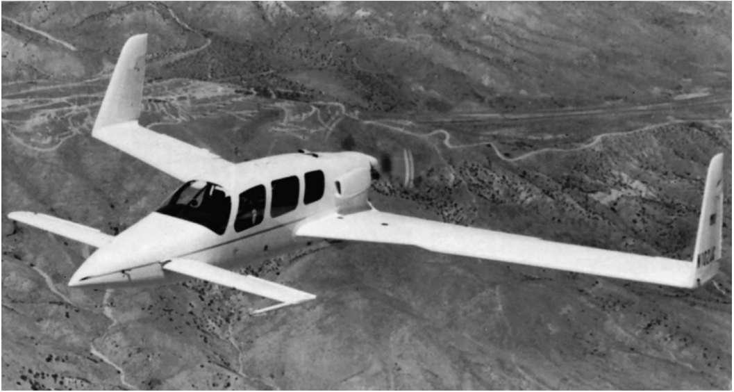
Figure 17.2 The canard six-place Jetcruzer, the first airplane to be granted a spin-resistant certification under FAA Part 23. Numerous attempts to spin the airplane were unsuccessful. (From AOPA Pilot , Aug. 1994)
