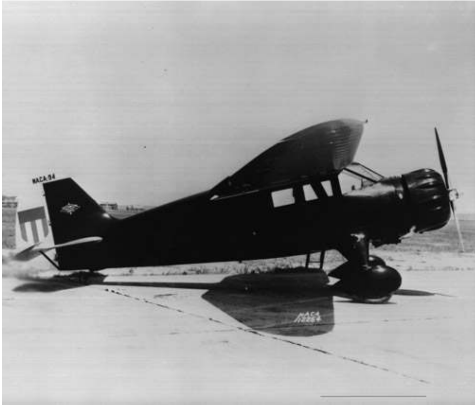
Figure 3.4 The Stinson SR-8E airplane used in Hartley Soulé's pioneering stability and control flight test measurements. (From NACA Rept. 700, 1940)
