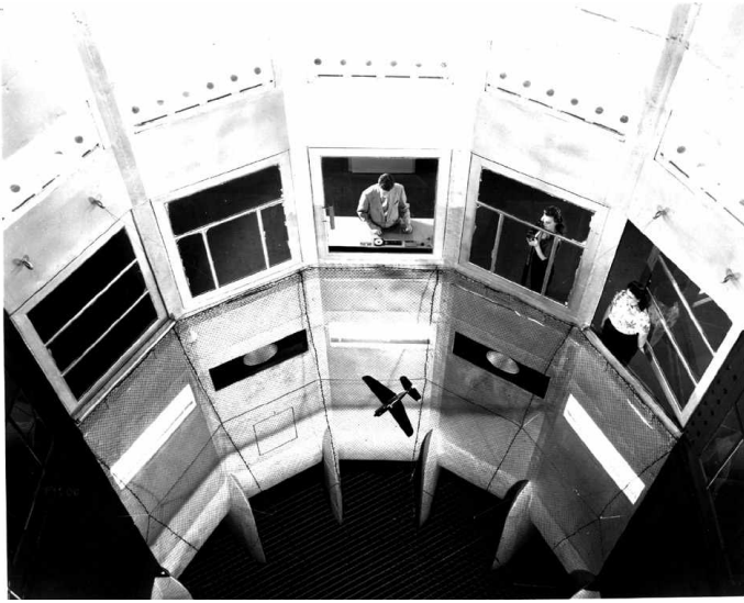
Figure 9.2 Model spinning in the test section of the NASA 20-Foot Free-Spinning Wind Tunnel. (From Neihouse, Klinar, and Scher, NASA Rept. R-57, 1960)
