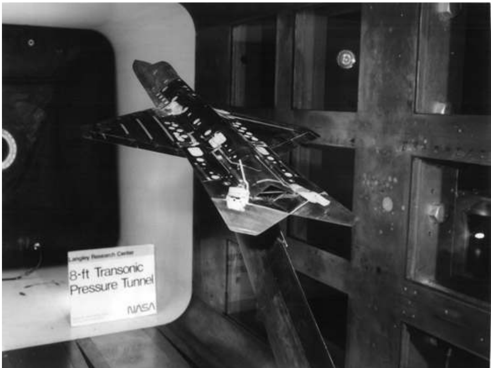
Figure 22.4 NASA 8-Ft. Transonic Wind-Tunnel model of a U.S. Air Force Multirole fighter concept, designed to have no vertical tail. Directional stability and control would be provided by thrust vectoring and low-radar-return control surfaces. (NASA photo 93-01934)
