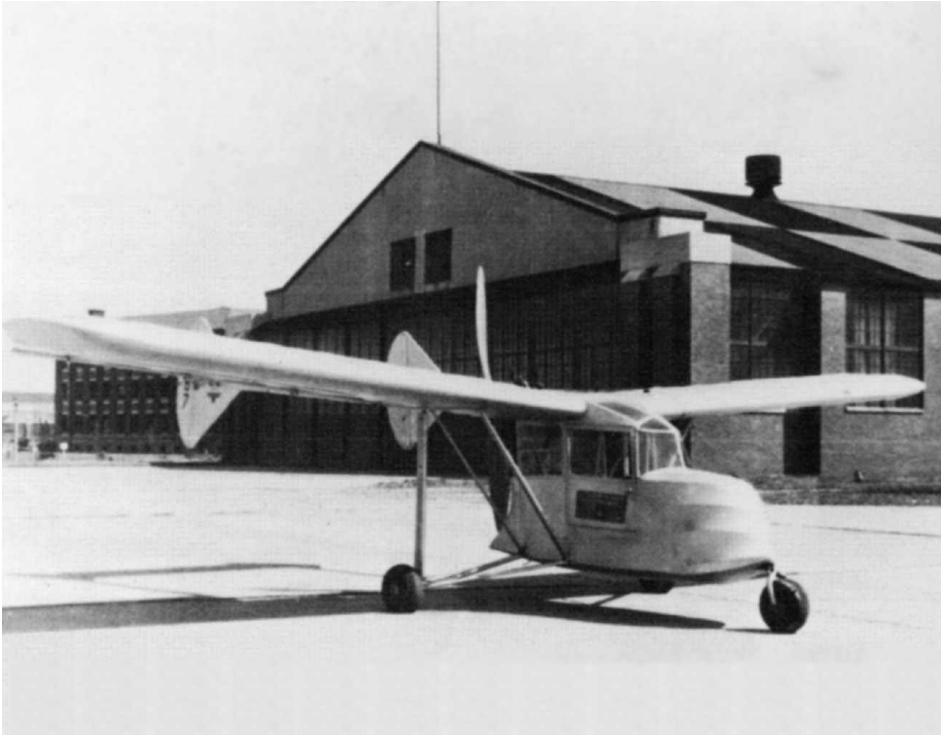
Figure 15.2 The 1935 Weick W-1A airplane, photographed in front of an NACA Langley Field hangar. This innovative airplane had full-span flaps and spoiler ailerons, limited up-elevator travel, and two-control operation. (From Weick, From the Ground Up , 1988)
