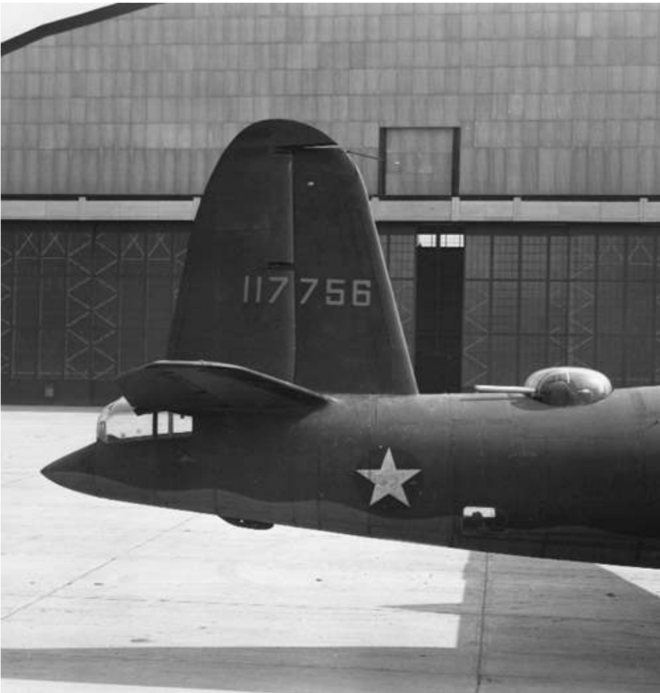
Figure 4.2 Experimental rudder horn balance-fitted to the Martin B-26 Marauder. This design reduced the rudder forces required for flight after failure of one engine. It was never put into production. (From U.S. Army Air Corps photo 108769, 1942)
