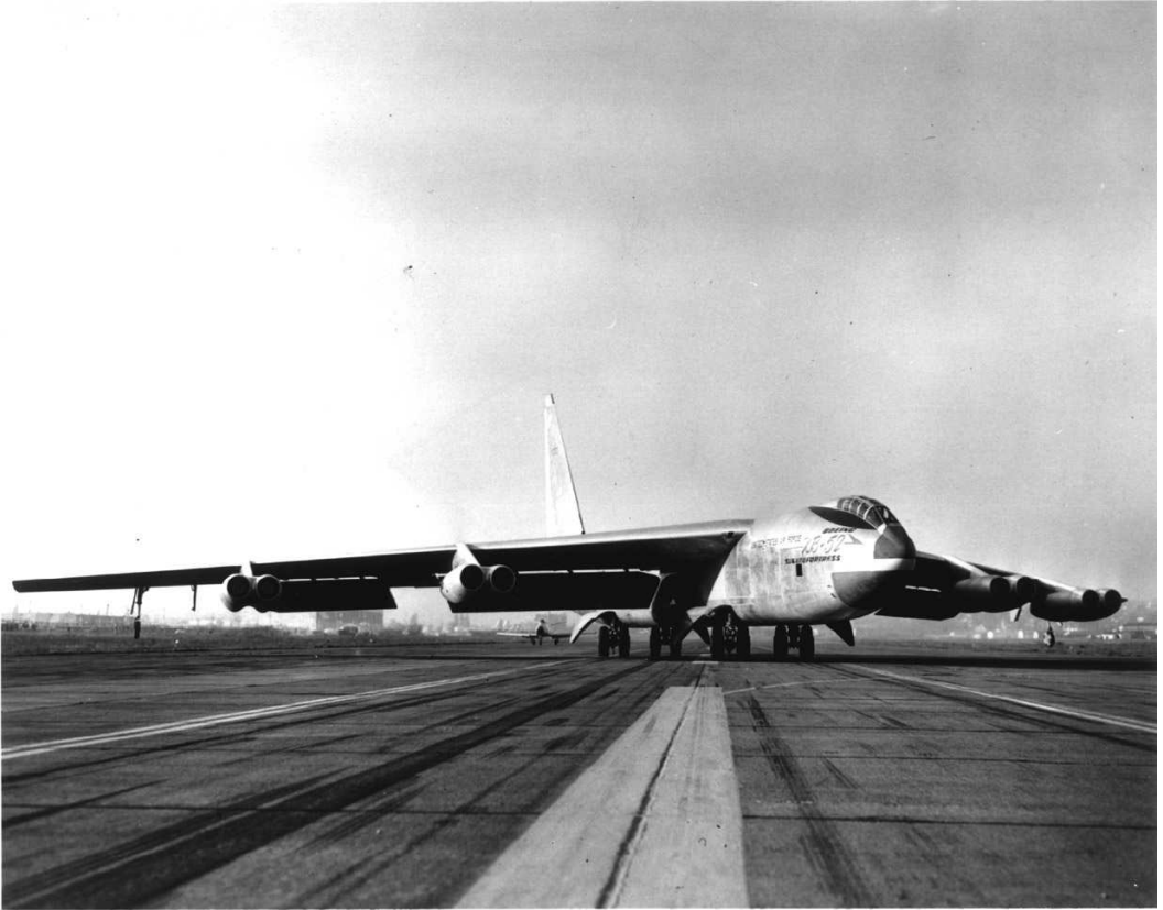
Figure 7.5 B-52 Stratofortress in a crosswind landing attitude. The landing gears are pointed down the runway while the airplane is yawed to the left, presumably into the relative wind. Crosswind landing gear reduces the need for rudder power. (From Loftin, NASA SP-468, 1985)
