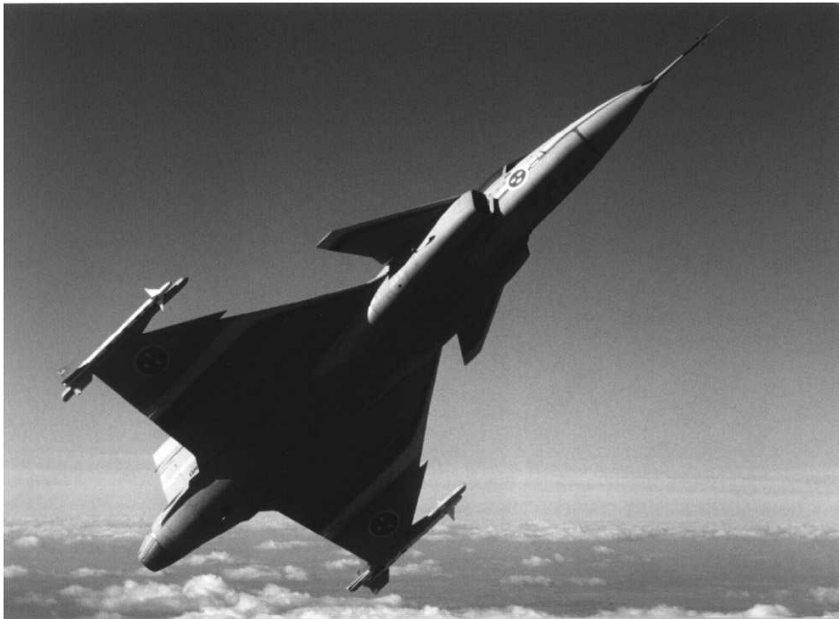
Figure 17.3 A modern canard airplane, the SAAB JAS 39 Gripen. (From Jane's All the World's Aircraft , 1987–1988)
