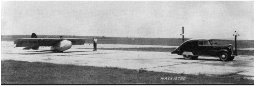
The Franklin PS-2 glider, towed behind a car for ground effect tests.
