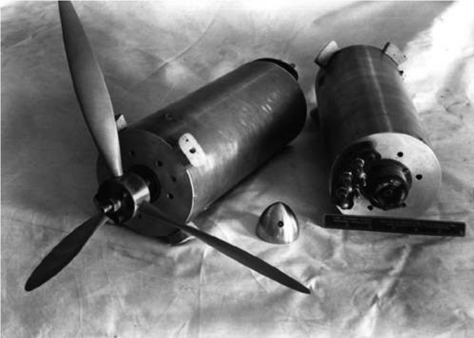
Figure 4.1 A typical compact electric induction motor developed in the late 1930s for powered wind-tunnel models. These motors developed 5 to 12 horsepower at 18,000 RPM. (From Millikan, Jour. of the Aeronautical Sciences , Jan. 1940)
