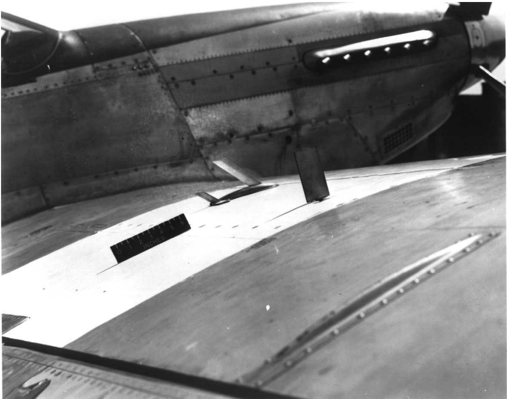
Figure 11.6 A sweptback-wing half-model mounted on the upper wing surface of a North American P-51, for wing flow testing during dives. The model is transonic, while the airplane is not. (From Phillips, Jour. of the Amer. Avia. Histor. Soc. , 1992)
