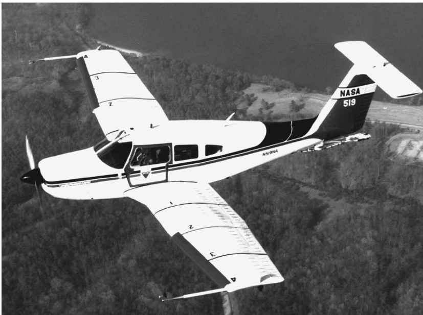
Figure 9.8 Discontinuous wing leading-edge extensions tested by NASA on the modified Grumman/American AA-1B Yankee ( above ) and the modified Piper PA-28R Arrow ( below ). (From DiCarlo AIAA Paper 80-1843 and Jane's All the World's Aircraft (1987–1988))
