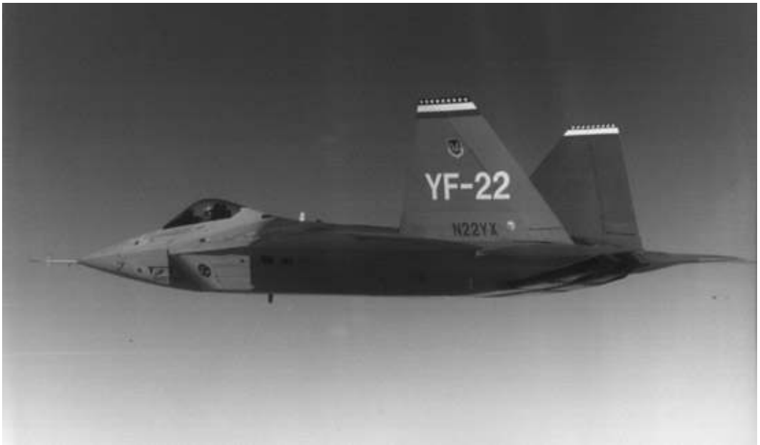
Figure 22.3 The Lockheed F-22, showing its vertical tail intersections with the wings that are shielded from ground radars. The vertical tail tips are canted outward to retain some effectiveness at high angles of attack. (From Lockheed Martin Corporation)
