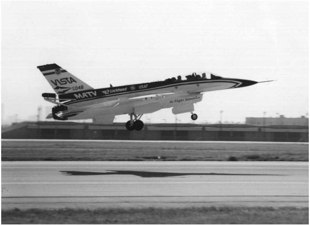
Figure 3.13 The Air Force Wright Laboratory's VISTA, or multiaxis thrust-vectoring airplane, a variable-stability machine based on the General Dynamics F-16D. Thrust is vectored up to 17 degrees in pitch and yaw, primarily for high-angle-of-attack research. (From Aerospace America , Dec. 1993)
