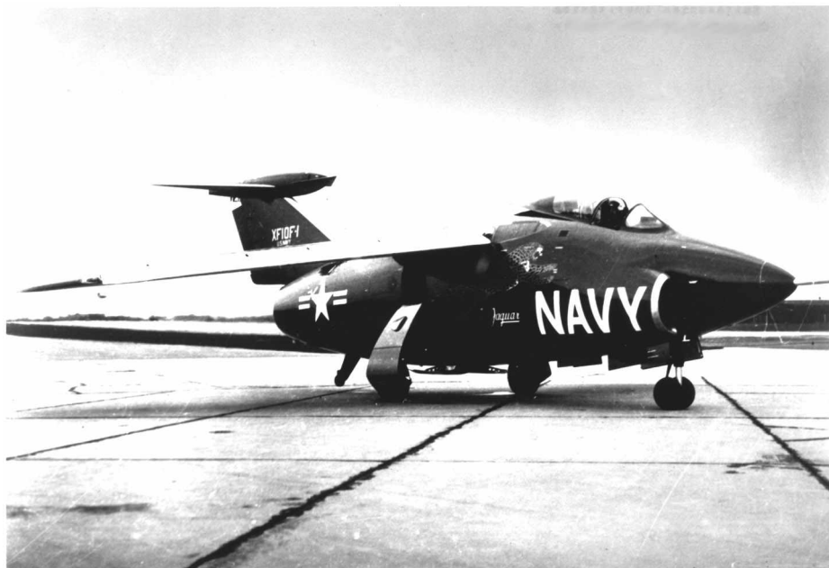
Figure 7.3 The Grumman XF10F-1 Jaguar, an attempt to avoid powered pitch controls. A freely pivoted canard-controlled body and wing is mounted on top of the vertical tail. The pilot's stick moves the canard, which controls the angle of attack of the pivoted body. (From National Air and Space Museum)
