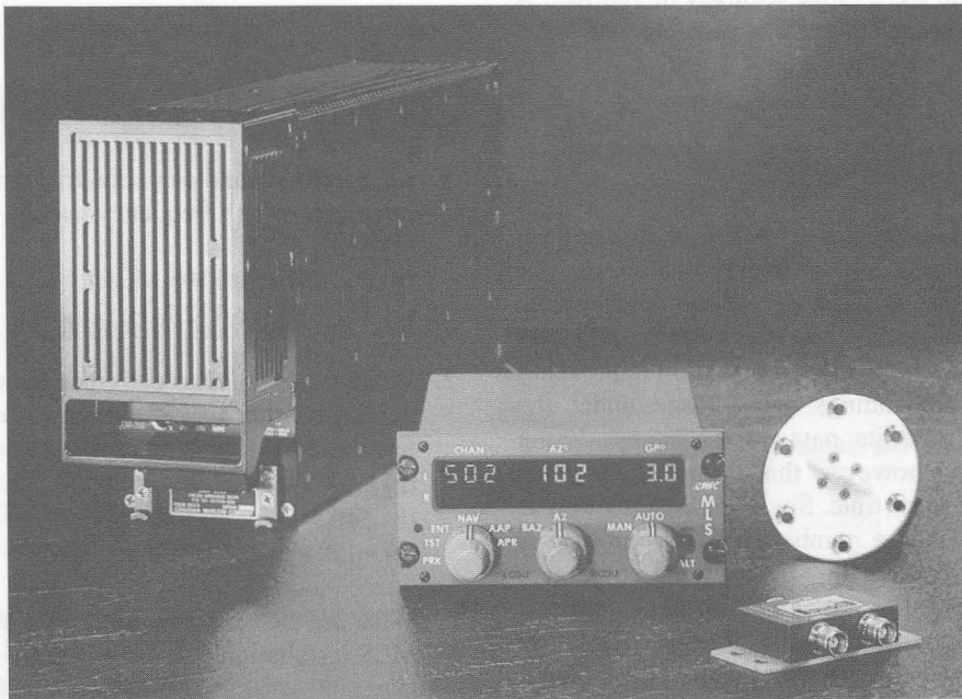
Figure 13.5 MLS airborne equipment (courtesy of CMC electronics)
