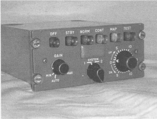
Figure 20.6(b) Typical weather radar control panel
