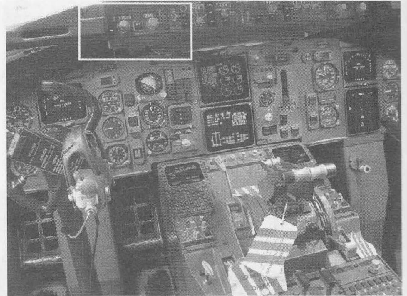
Figure 10.7 Typical VOR control panel
