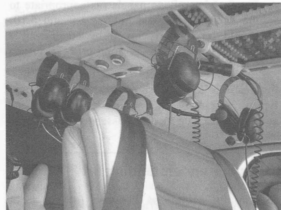
Figure 6.8 Headsets and boom microphones in a four-seat rotorcraft
