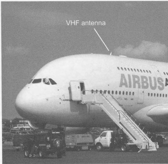
Figure 4.25 The forward quarter-wave VHF blade antenna on the Airbus A380 (see page 15 for the VHF antenna locations on a Boeing 757)
