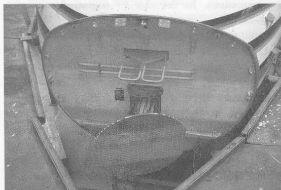
Figure 20.3(a) Weather radar antenna
