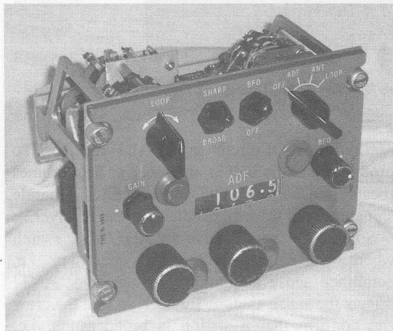
(b) Typical ADF control panel
