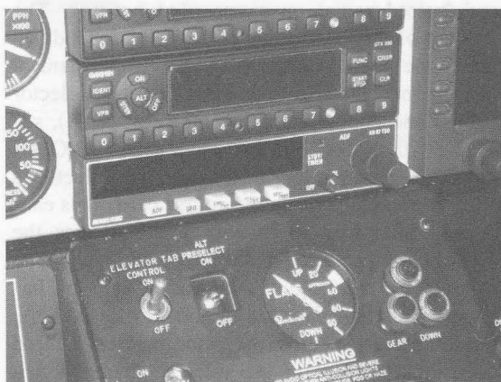
(b) Navigation and communications panel/receiver used in general aviation
