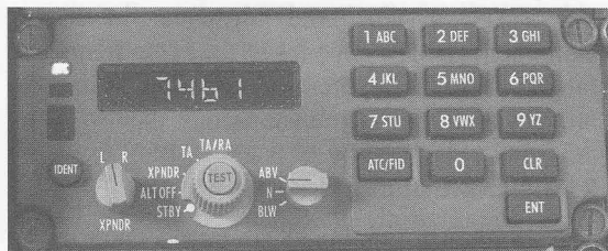
Figure 21.6(b) ATC control panel
