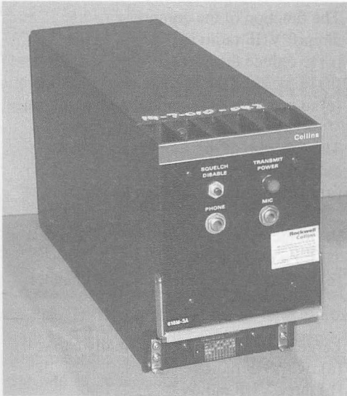
Figure 4.21 Aircraft VHF radio removed from its rack mounting
