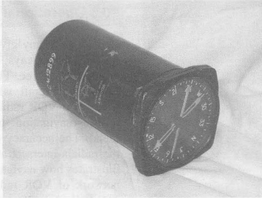
(a) RMI with two bearing pointers
