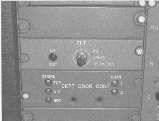
Figure 7.5 Type-AF ELT control panel (note the three switch positions marked ON, ARMED and TEST/RESET)
