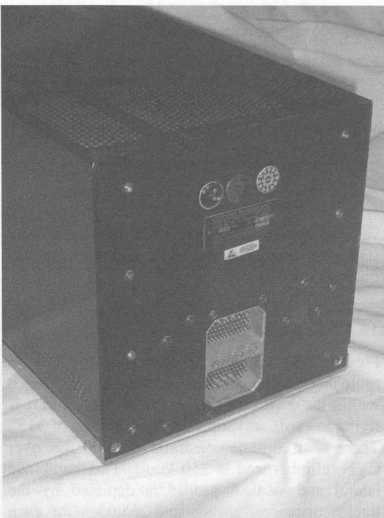
Figure 19.8 Program pins located in the computer's connector
