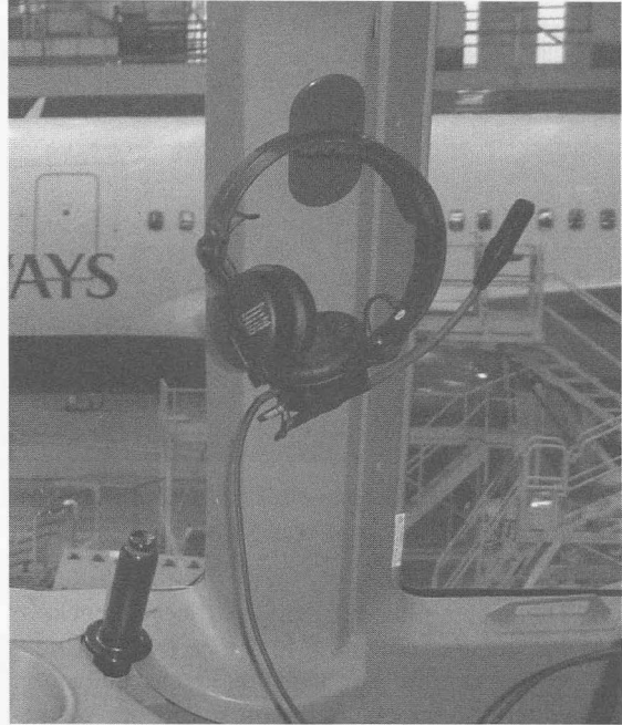
Figure 6.7 First officer's headset and boom microphone in an A320 aircraft
