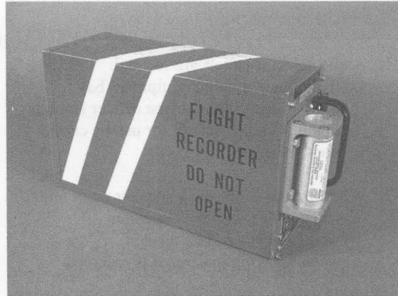
Figure 6.11 Cockpit voice recorder fitted with an underwater locator beacon (ULB)
