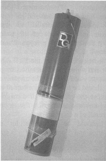
Figure 7.1 Type-W ELT with attachment cord secured by water-soluble tape (the antenna has been removed)
